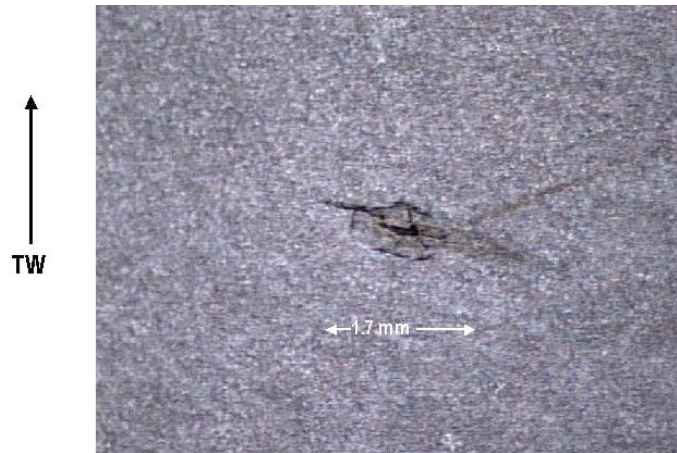
Figure 1 Small Flaw in Plate Material
