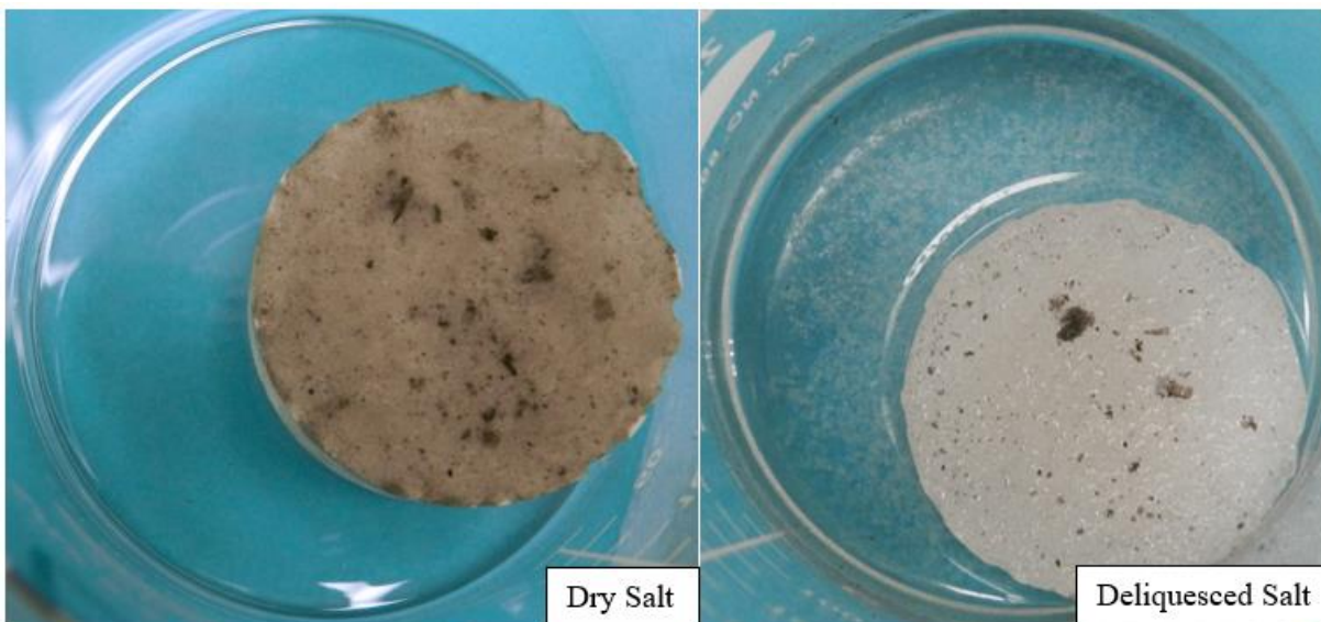
Figure 15. Photographs of LiCl-KCl salt before (left) and after (right) exposure to air at 32°C.
