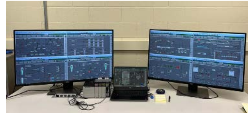
Full-scope Advanced Nuclear CYbersecurity (FANCY) Hardware-in-the-loop testbed
