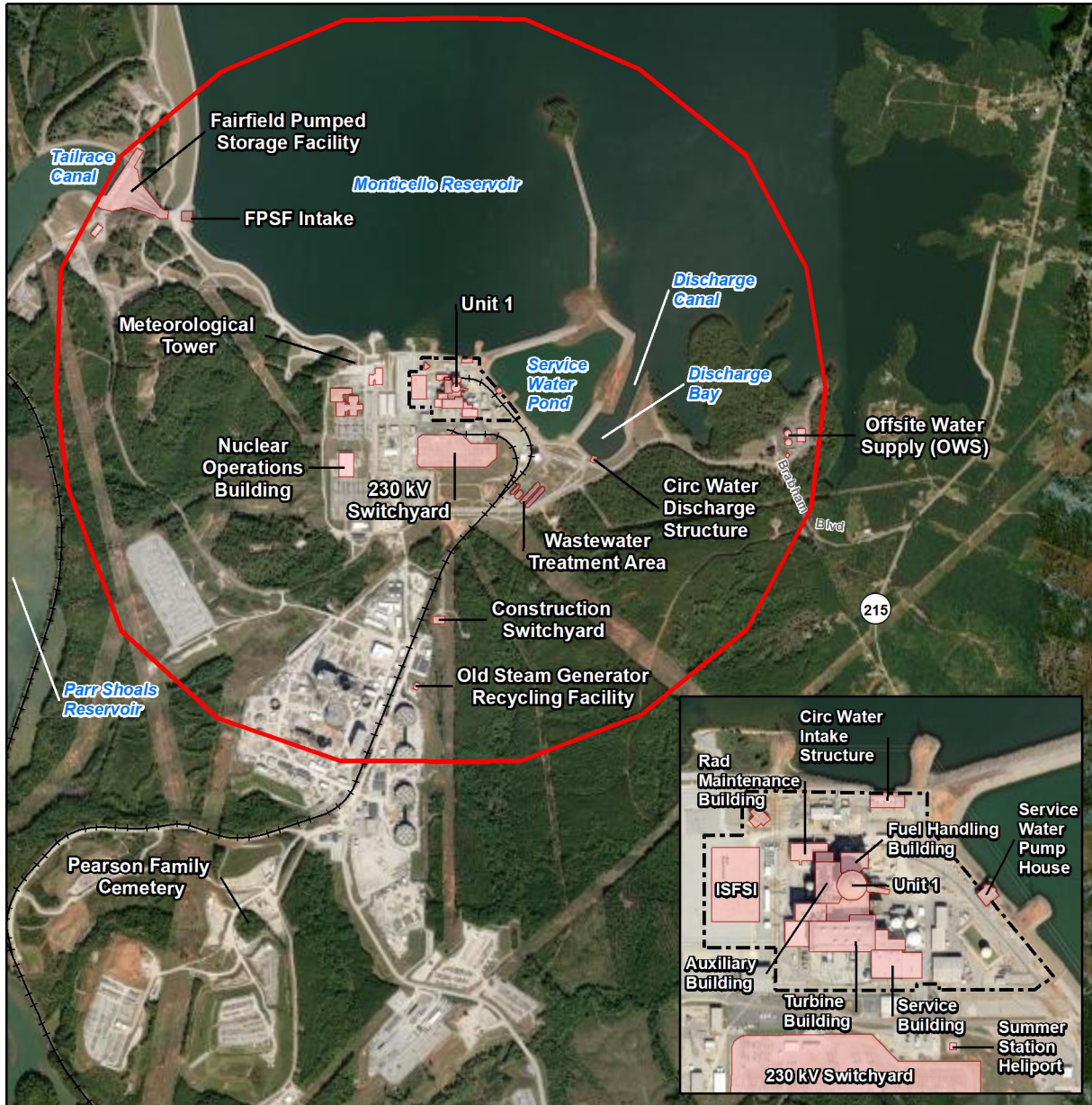
Figure E3.1-1 VCSNS Plant Layout
