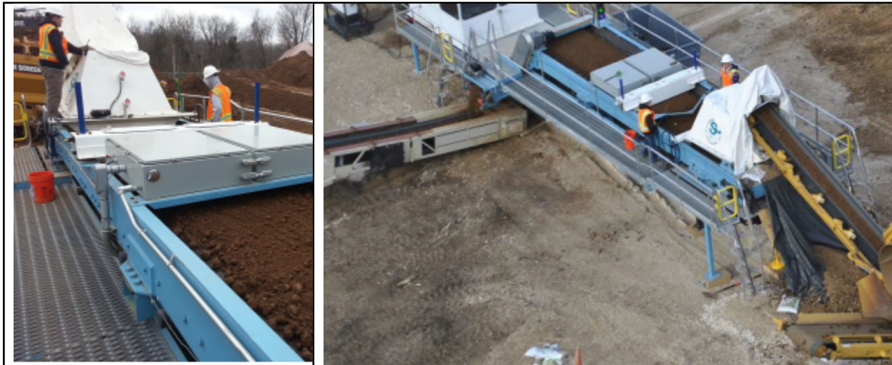
Figure 2.9 Example (Iso-Pacific S3) Soil Sorting System. See Appendix J in SC&A (2022) for Additional Information About Various Systems.
