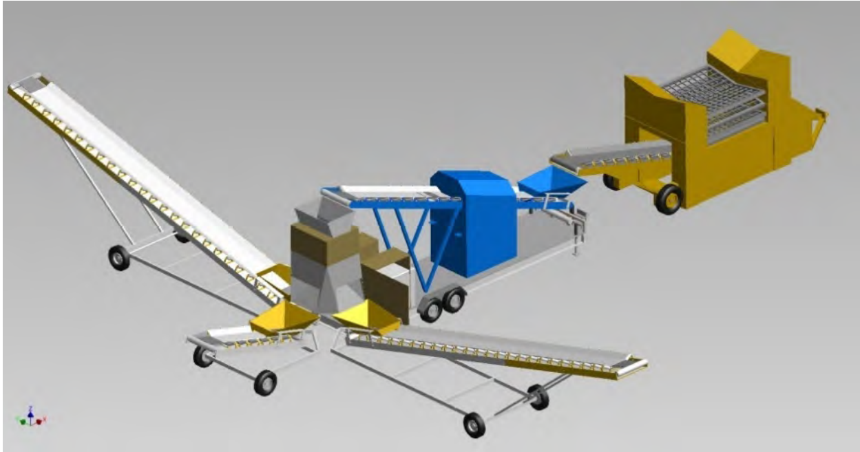
Figure 2.8 Example (ANTECH) Soil Measurement and Segregation System. See Appendix J in SC&A (2022) for Additional Information About Various Systems.
