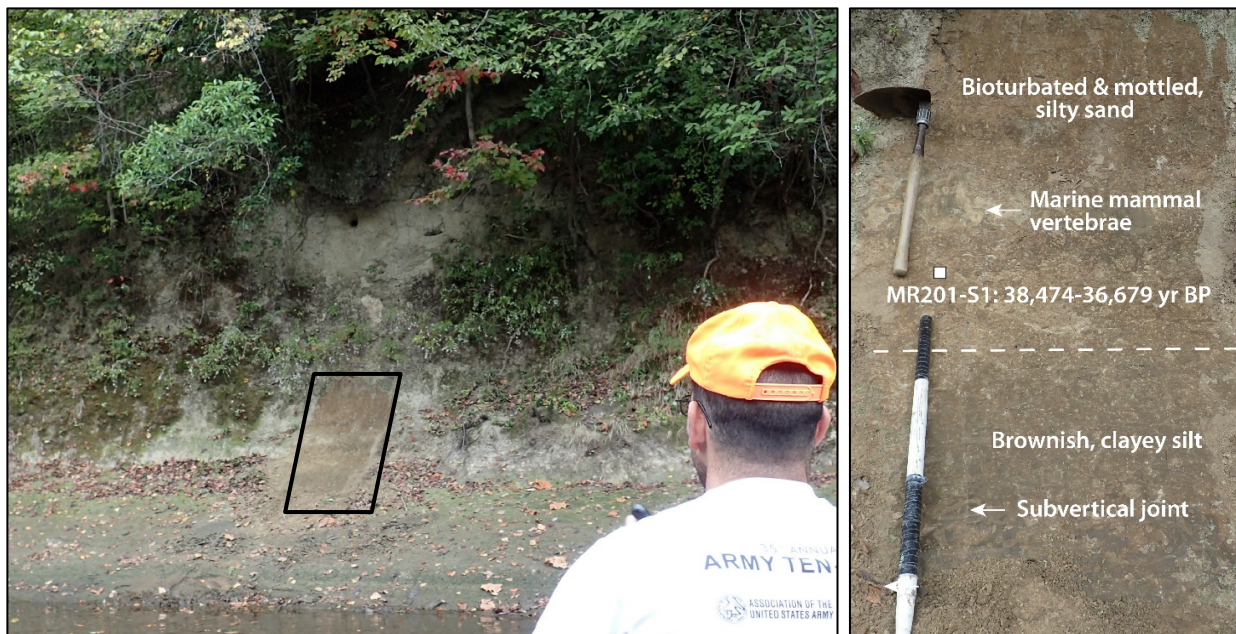
Figure 5-1: Photographs at site MR201 of cutbank exposure in 6-m-high river terrace along Mattaponi River: (left) exposure is very good of lower portion of cutbank; black rectangle outlines area of closeup photo; (right) annotated closeup of bioturbated and mottled silty sand overlying brownish, clayey silt with subvertical joints. C14 dating of sample MR201-S1 indicates mottled silty sand is upper Pleistocene in age. Underlying clayey silt is probably member of Chesapeake Group. For scale, black and white intervals on hoe handle are 25 cm long.
