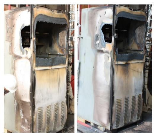
Figure 7. Photographs of 4 sec test enclosure (Left 2-21 26.6kA 101MJ / Right 2-24 29.8kA 122MJ)
