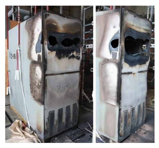
Figure 6. Photographs of 2 sec test enclosures (Left 2-19 25.8kA 39MJ / Right 2-22 32.0kA 51MJ)
