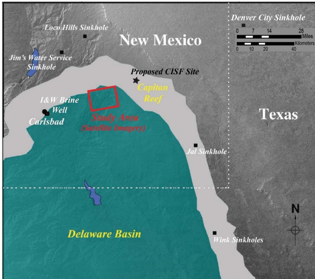
Figure 3.4-13 Regional Map of Southeastern New Mexico and West Texas Showing Locations of Anthropogenic Sinkholes and Satellite Imagery Study Area Discussed in the Text (Modified from Zhang et al., 2018)
