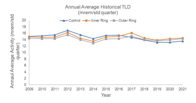
Figure 4.9.1-2: Graph of Historical Direct Gamma Measurements
