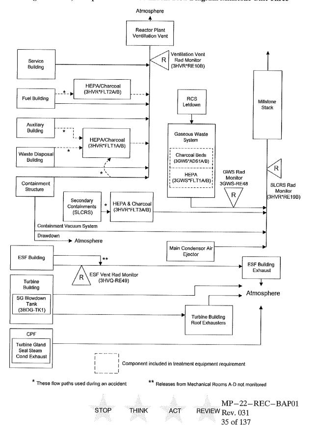
Figure I.D.-3, "Simplified Gaseous Effluent Flow Diagram Millstone Unit Three"
