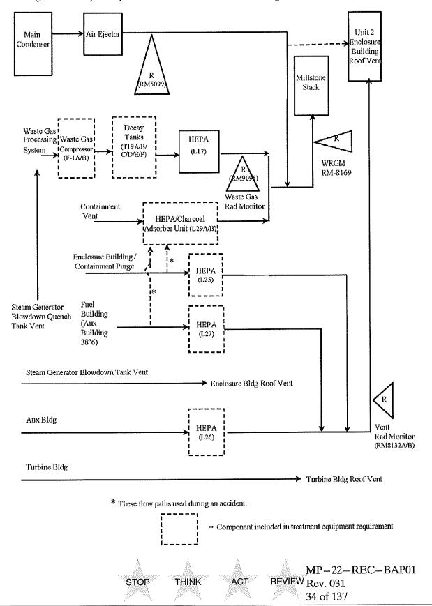
Figure I.D. – 2, "Simplified Gaseous Effluent Flow Diagram Millstone Unit Two"
