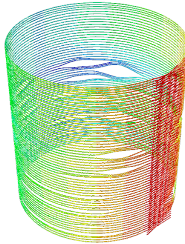
Figure 3-26 Set 1 of 2 hoop tendon stress after jacking.
