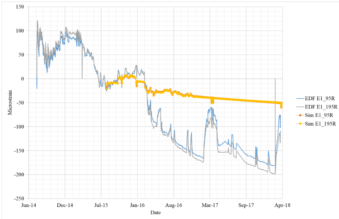
Figure A-16 Comparison strain gage data for C95 and C195R.
