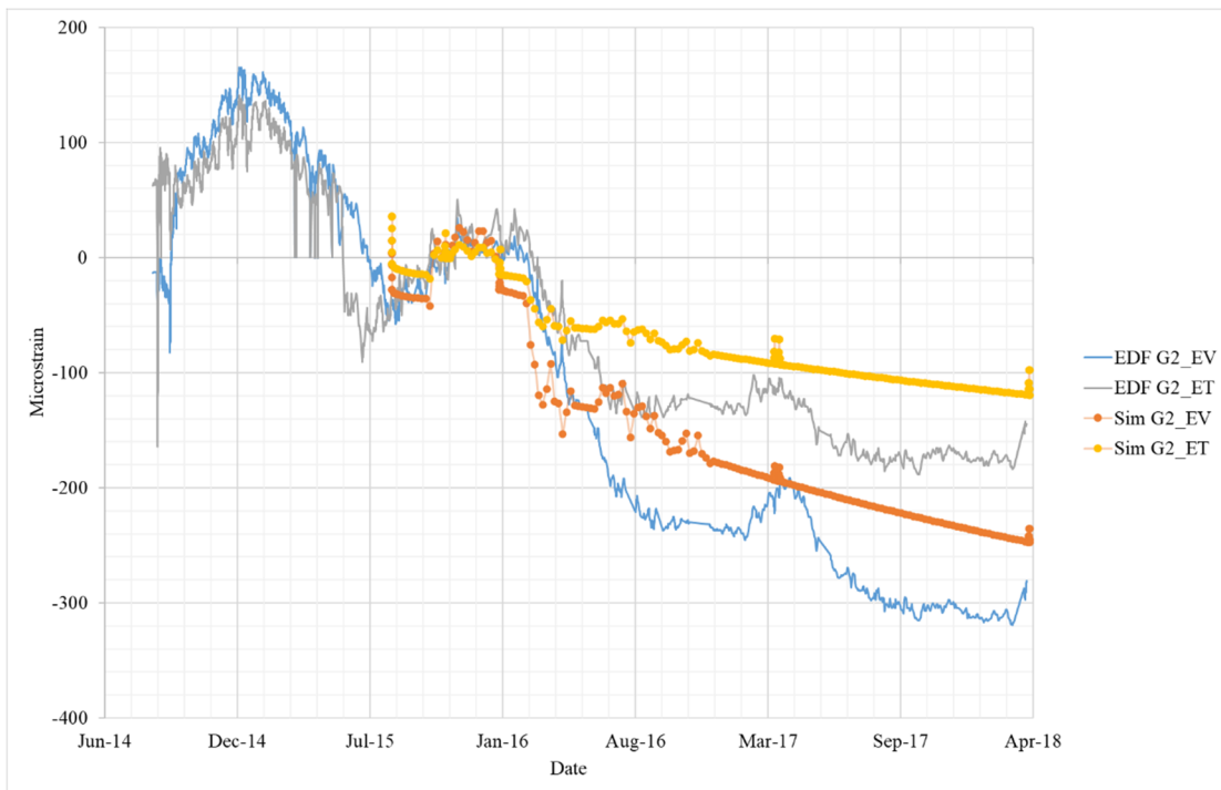
Figure A-19 Comparison strain gage data for G2EV and G2ET.
