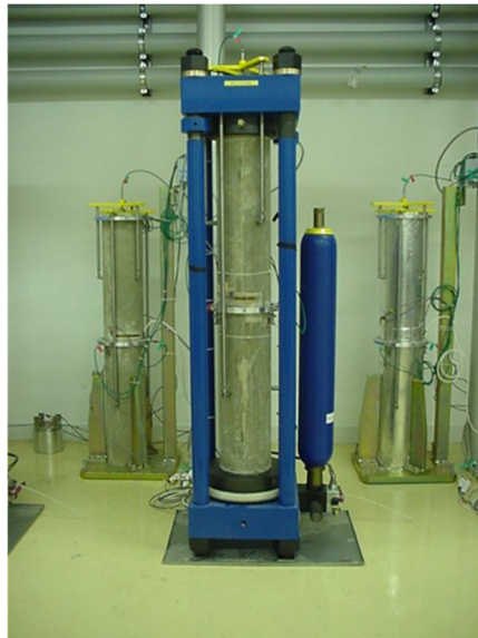
Figure 3-41 EDF creep test configuration. Specimen is 0.16 m diameter and 1 m tall.
