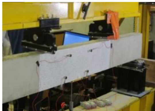
Figure 4-4 3-point bending test of concrete specimen monitored with acoustic emission. (Garnier, et al., 2018)
