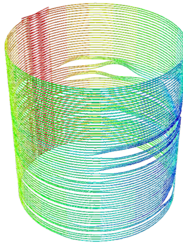
Figure 3-28 Set 2 of 2 hoop tendon stress after jacking.
