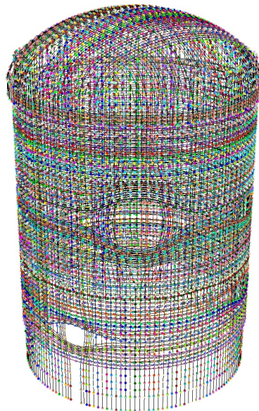
Figure 3-20 VeRCoRs tendon geometry and mesh.
