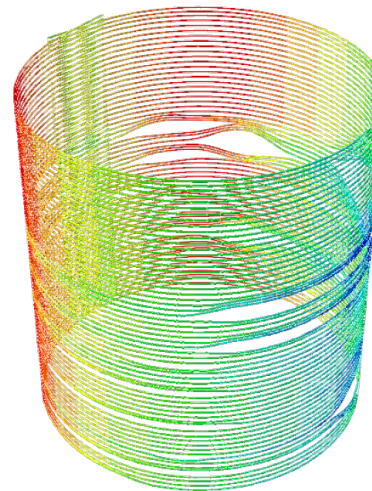
Figure 3-29 Set 2 of 2 hoop tendon stress after anchor set.
