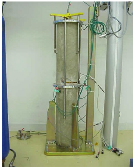
Figure 3-37 Drying shrinkage concrete cylinder specimen.
