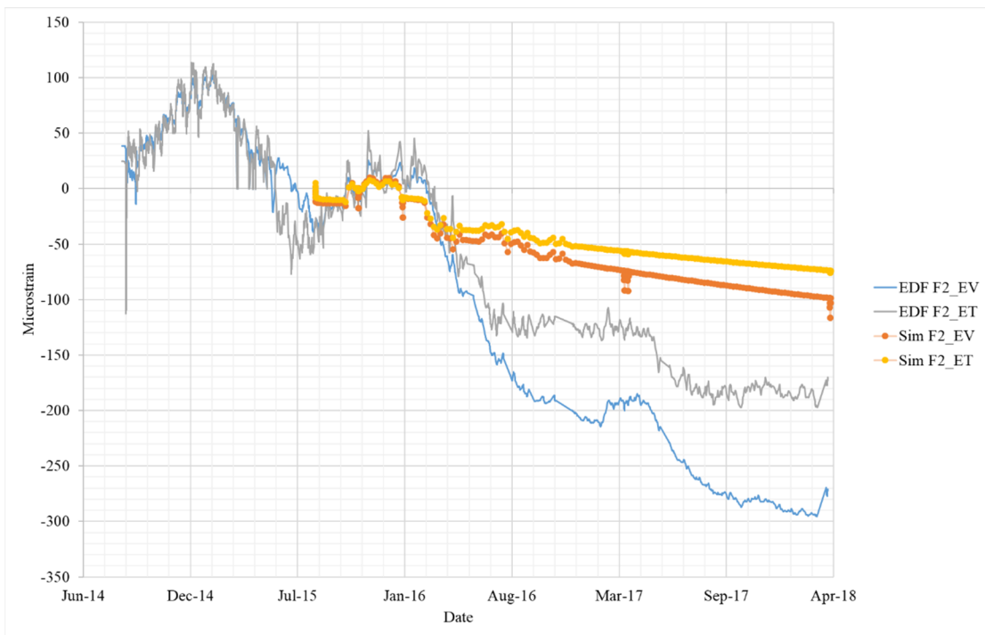
Figure A-21 Comparison strain gage data for F2EV and F2ET.
