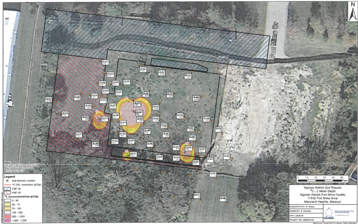
Figure 3. Carbon-14 soil concentrations from 2m depth (adapted from ADAMS Accession No. ML17240A366)
