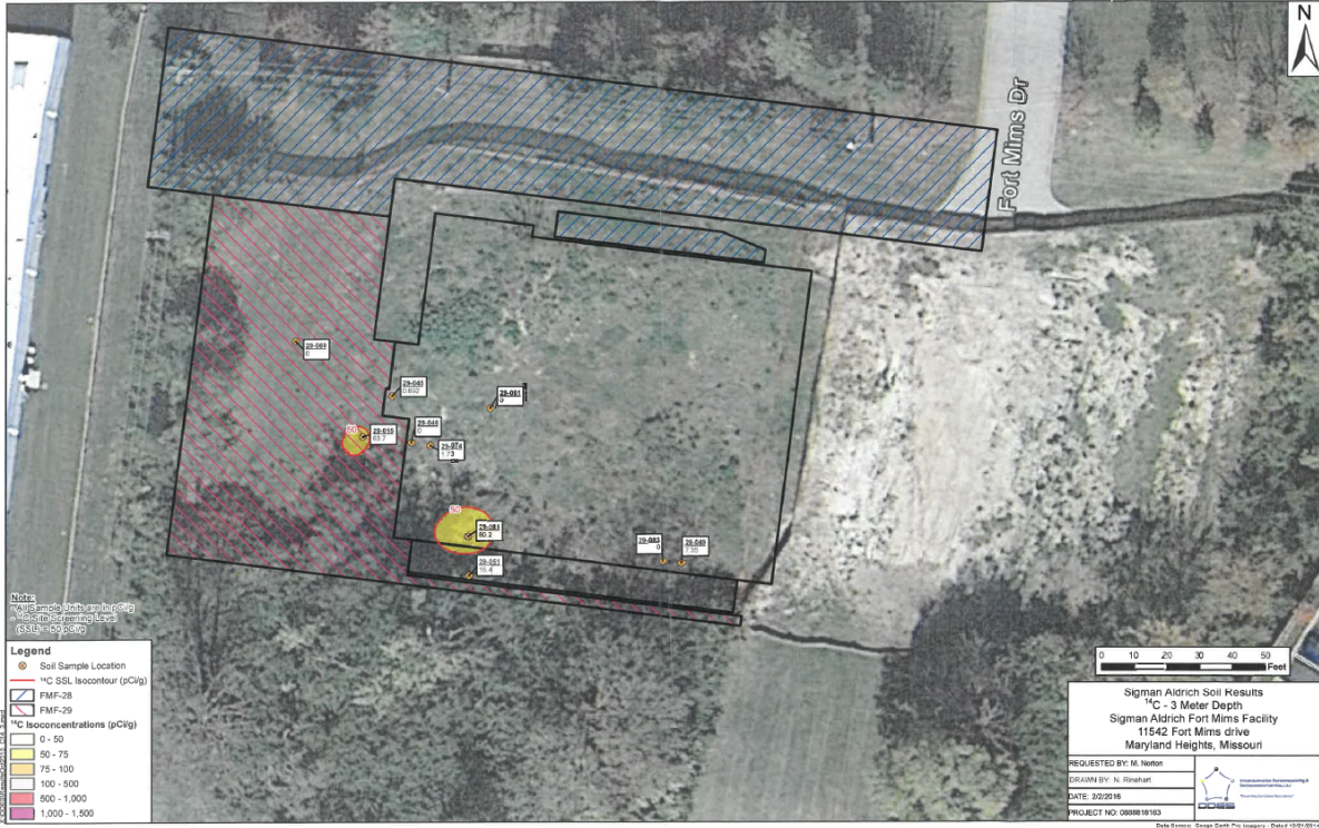
Figure 4. Carbon-14 soil concentrations from 3m depth (adapted from ADAMS Accession No. ML17240A366)
