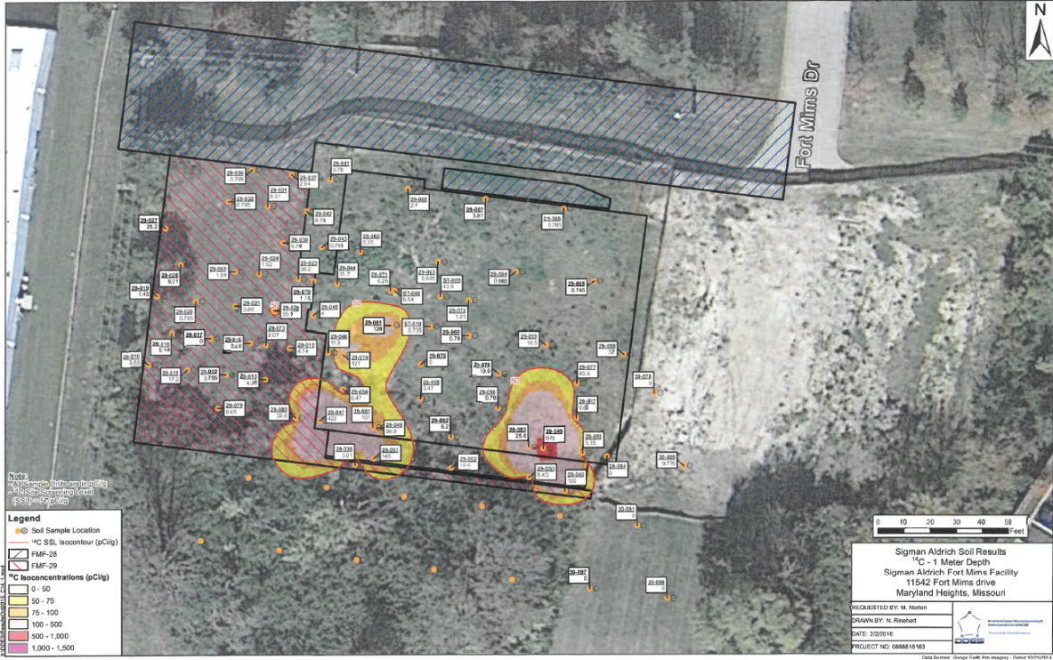
Figure 2. Carbon-14 soil concentrations from 1m depth (adapted from ADAMS Accession No. ML17240A366)
