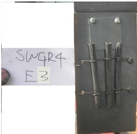
Figure F-14 SWGR Test 10 Detailed Target Damage (continued)
