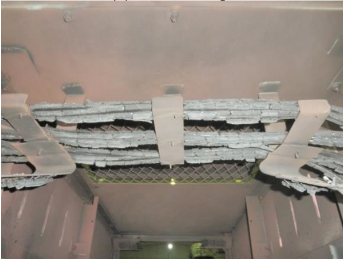
Figure 3.11-5 SWGR Test 9 Cable Damage
