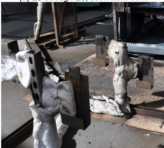
Figure 2.11-7 DP Test 9 Target Damage and Target Numbers
