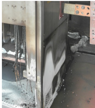
Figure 2.11-4 DP Test 9 Exterior Cabinet Damage
