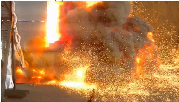
Figure 2.8-3 DP Test 7 Flames during Arc
