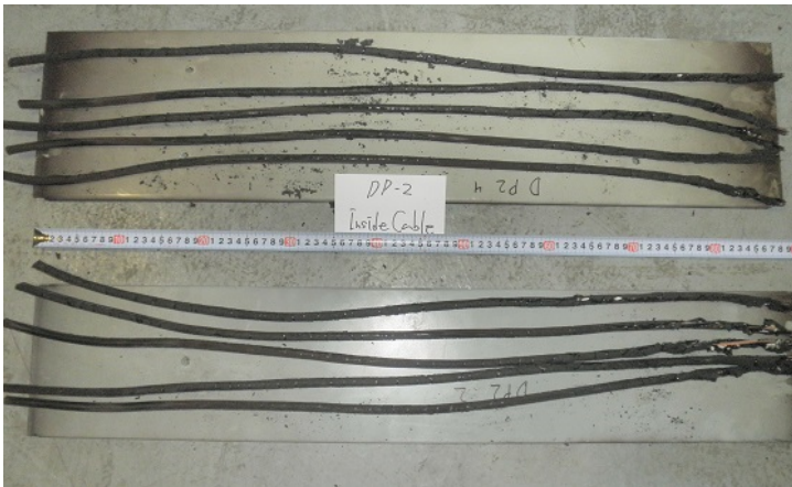
Figure 2.9-5 DP Test 8 Interior Cable Damage
