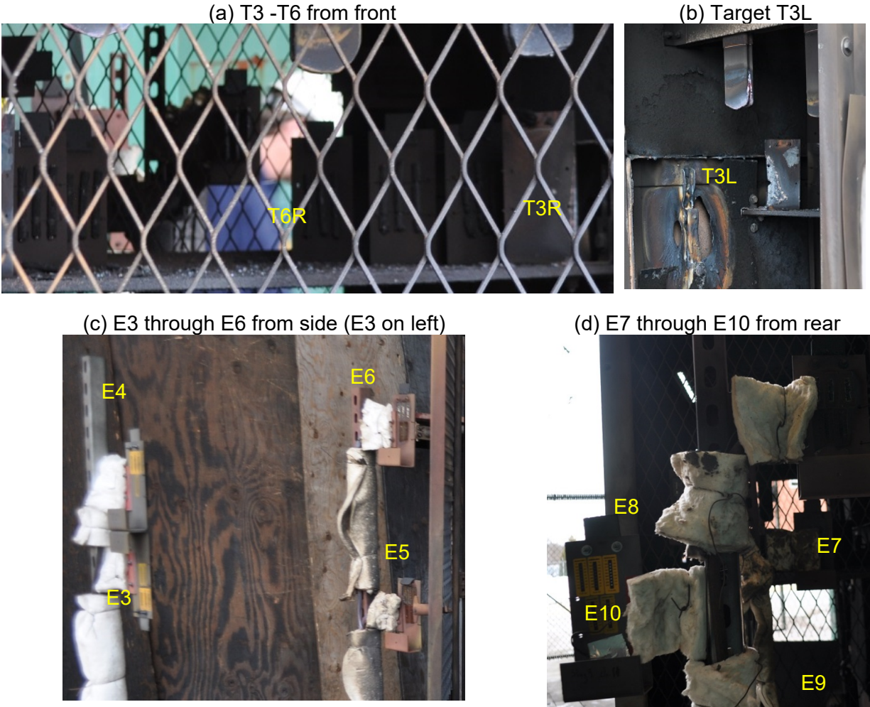
Figure 3.10-7 SWGR Test 8 Target Results and Target Numbers: Observations
