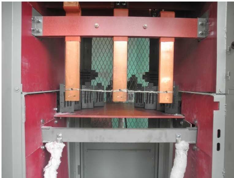
Figure 3.9-1 Red Board Added for SWGR Test 8, 9, 10
