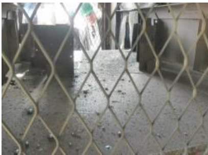
(g) Metal sputter SWGR Test 9 (from front)
