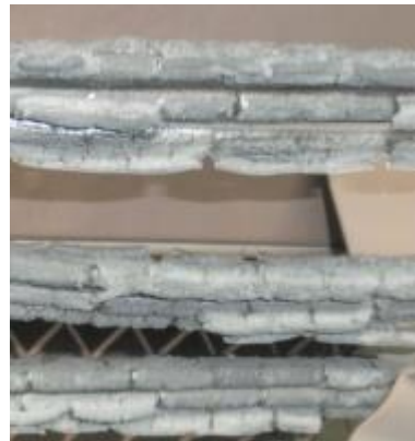
Figure 4.2-1 SWGR Test Interior Cable Bundle Damage
