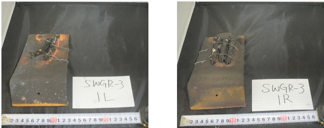
Figure F-12 SWGR Test 9 Detailed Target Damage
