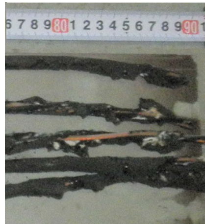
Figure 2.9-5 DP Test 8 Interior Cable Damage
