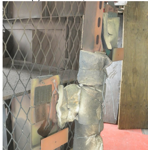
Figure 3.8-7 SWGR Test 7 Target Damage
