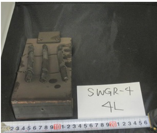
Figure F-14 SWGR Test 10 Detailed Target Damage (continued)
