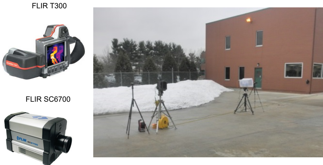
Figure A-10 Thermal and High-Speed Cameras
