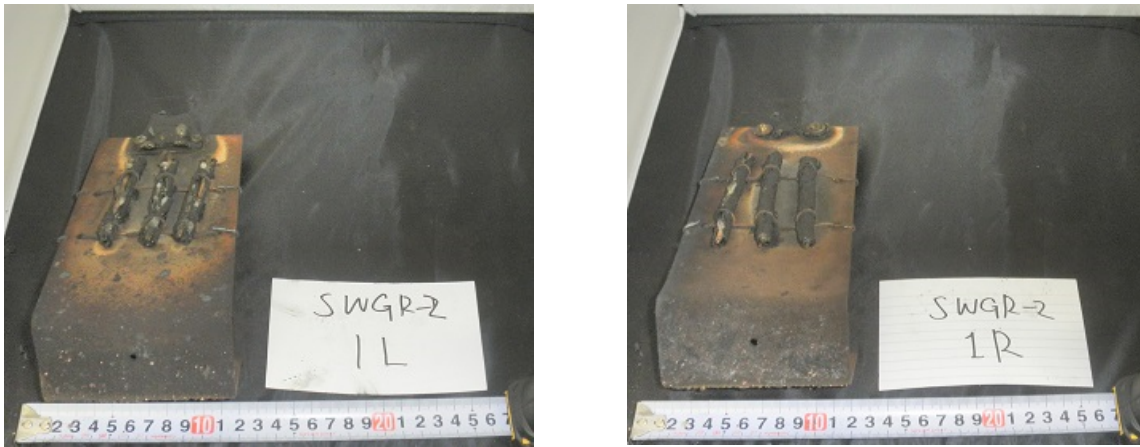
Figure F-10 SWGR Test 8 Detailed Target Damage
