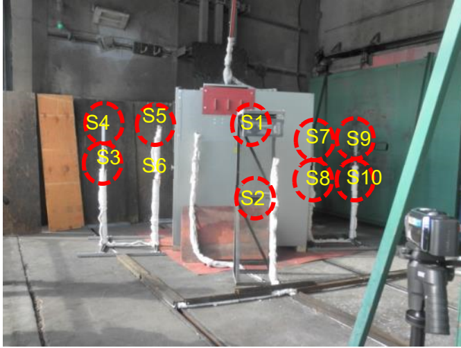
Figure 3.5-2 SWGR Tests 7 through 10 Slug Calorimeter (and External Target) Locations
