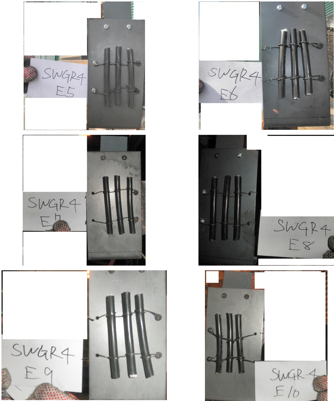
Figure F-14 SWGR Test 10 Detailed Target Damage (continued)
