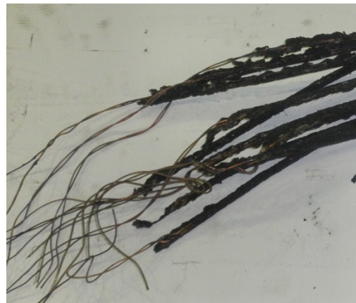
Figure 2.11-5 DP Test 9 Interior Cable Damage
