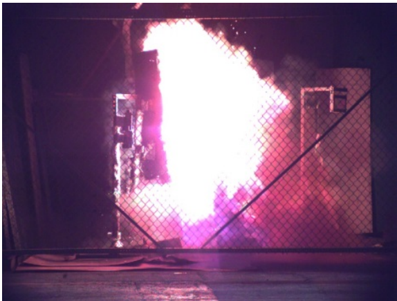
Figure 3.12-3 SWGR Test 10 High Speed Images of Door Opening
