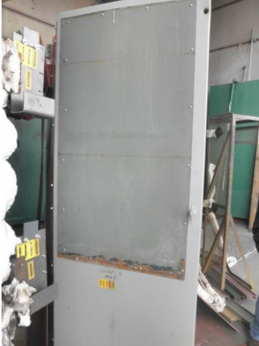
Figure 3.12-5 SWGR Test 10 Exterior Damage
