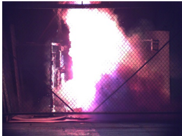
Figure 3.12-3 SWGR Test 10 High Speed Images of Door Opening
