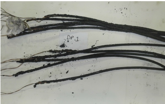
Figure 2.11-5 DP Test 9 Interior Cable Damage
