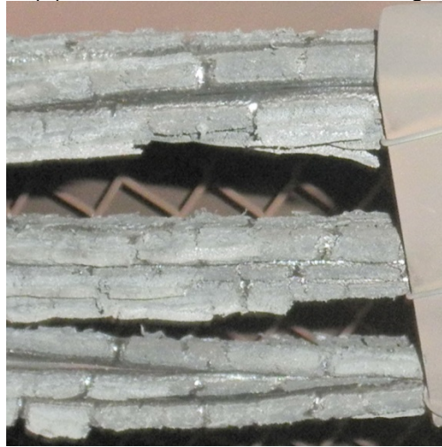
Figure 3.11-5 SWGR Test 9 Cable Damage
