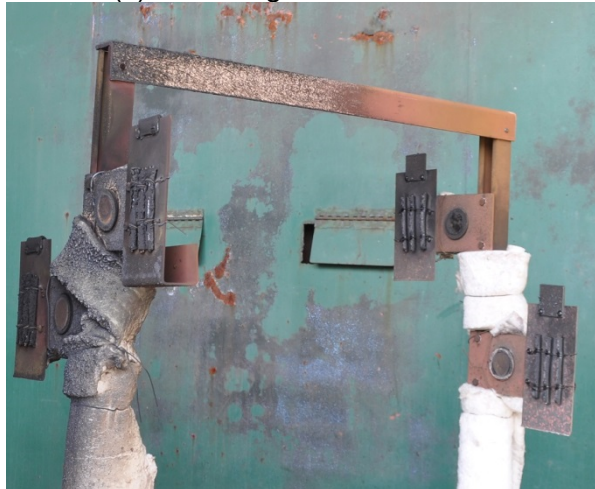
Figure 3.11-7 SWGR Test 9 Target Damage and Target Numbers: Observations
