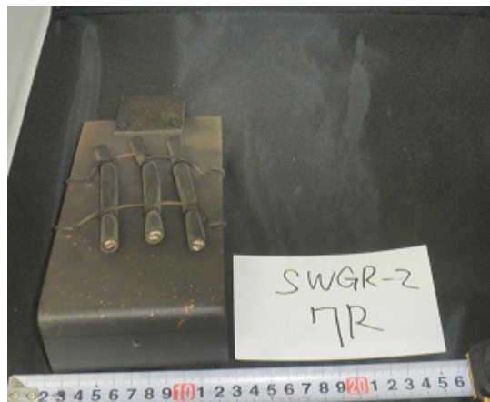
Figure F-14 SWGR Test 10 Detailed Target Damage (continued)
