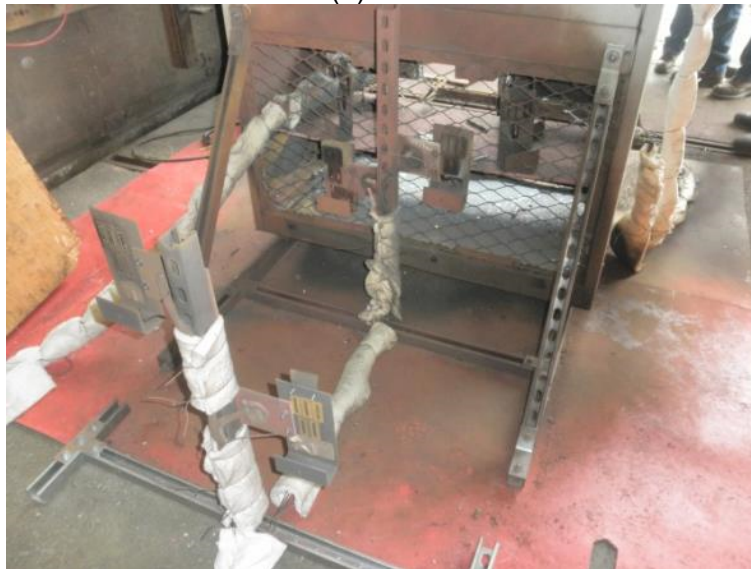
Figure 2.9-4 DP Test 8 Exterior Damage
