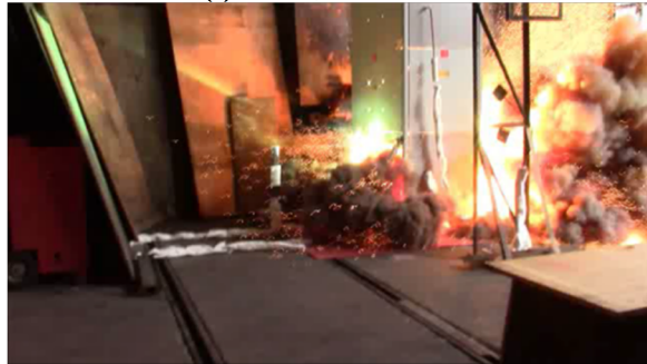
Figure 2.8-3 DP Test 7 Flames during Arc
