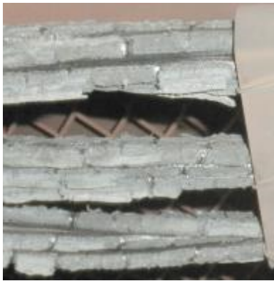
Figure 4.2-1 SWGR Test Interior Cable Bundle Damage
