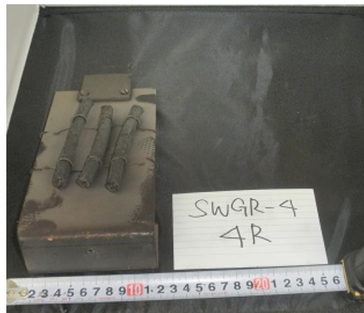
Figure F-14 SWGR Test 10 Detailed Target Damage (continued)
