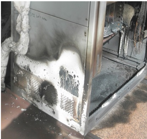
Figure 2.11-4 DP Test 9 Exterior Cabinet Damage
