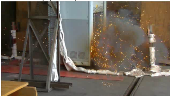
Figure 2.8-4 DP Test 7A Flames during Arc
