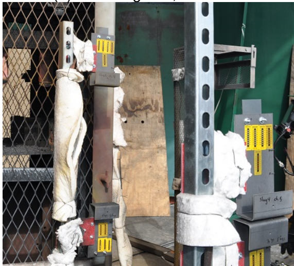
Figure 3.8-7 SWGR Test 7 Target Damage
