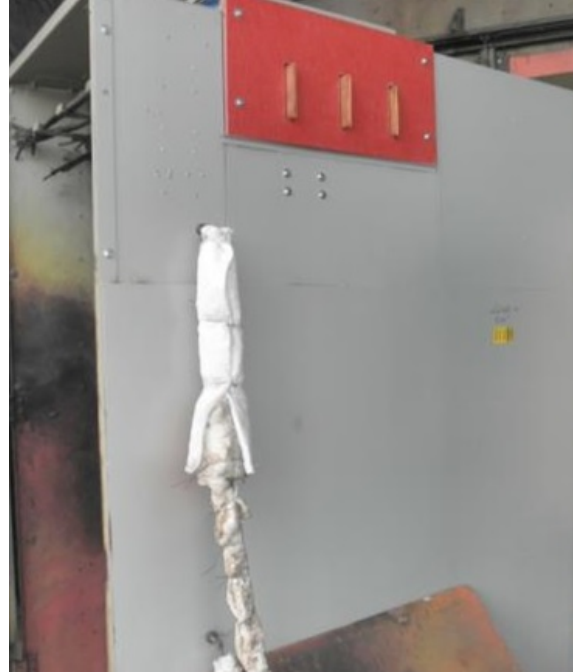
Figure 3.12-5 SWGR Test 10 Exterior Damage
