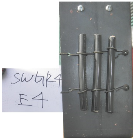
Figure F-14 SWGR Test 10 Detailed Target Damage (continued)
