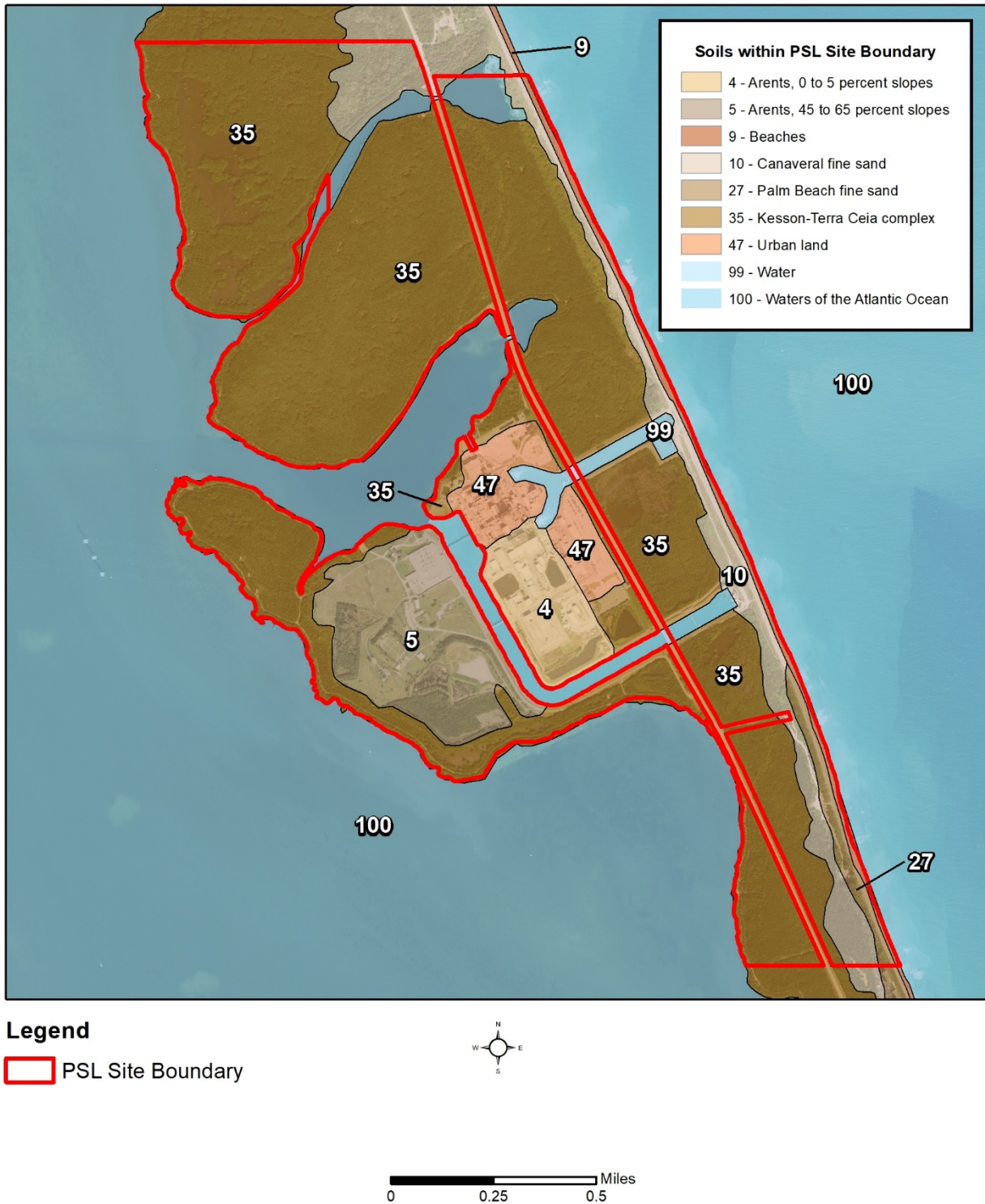
Figure 3.5-4 Distribution of Soil Units, PSL Property
