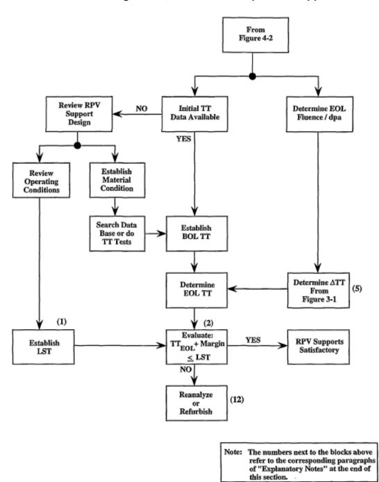
Figure 9-4 NUREG-1509 Figure 4-4, Transition Temperature Approach
