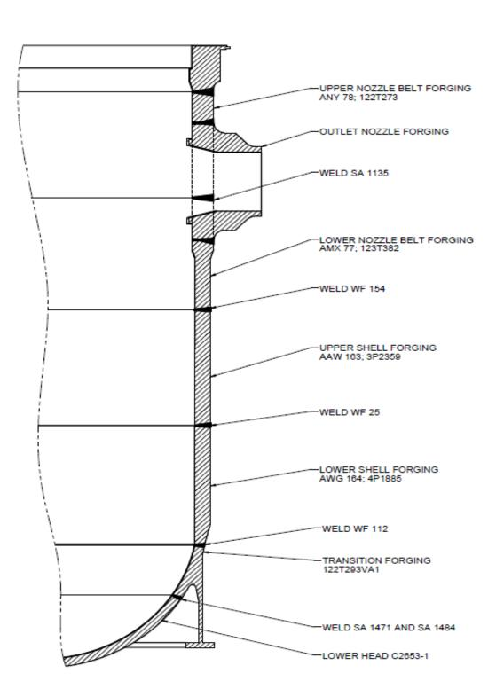
Figure 2-2 ONS Unit 2 Reactor Vessel Shell
