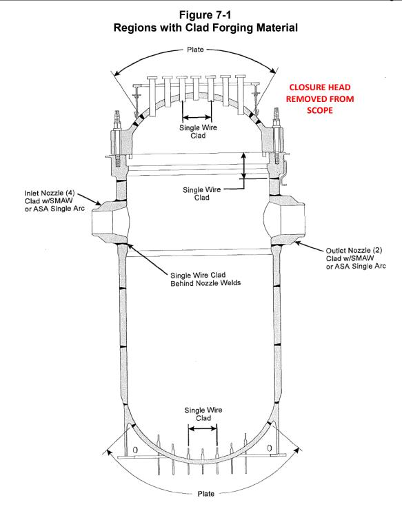
Note: All inside surfaces six-wire clad except as noted All material ASTM A508, Class 2 except plate, as noted.
