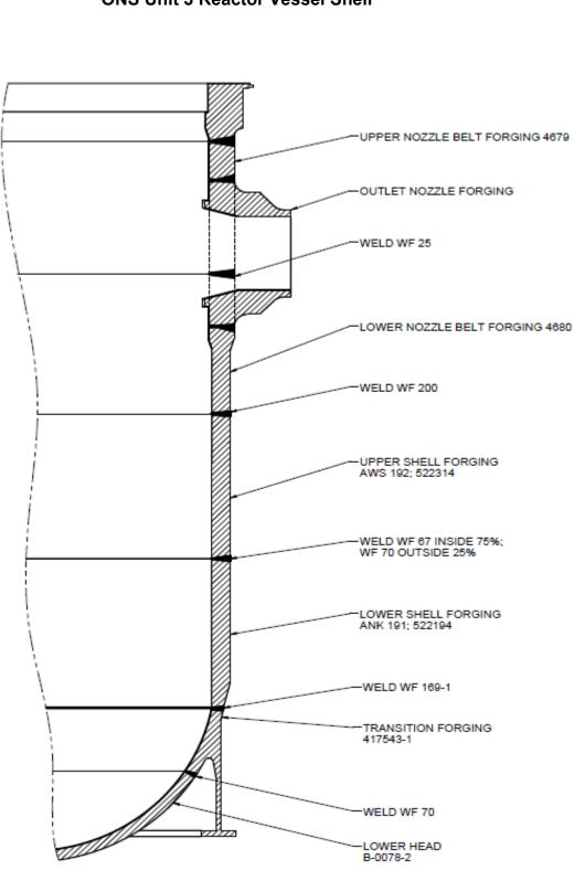
Figure 2-3 ONS Unit 3 Reactor Vessel Shell
