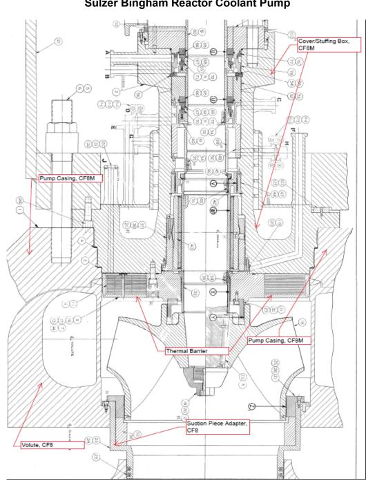
Figure 10-1 Sulzer Bingham Reactor Coolant Pump Framatome Reactor Vessel and RCP TLAA and Aging Management Review Input to the ONS SLRA
