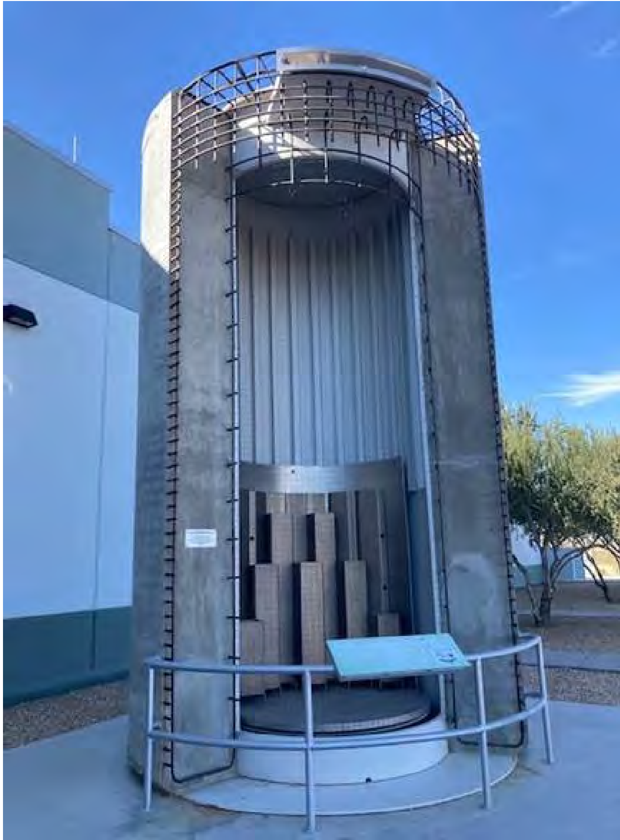
Prototype concrete casks at the Palo Verde Energy Education Center.
