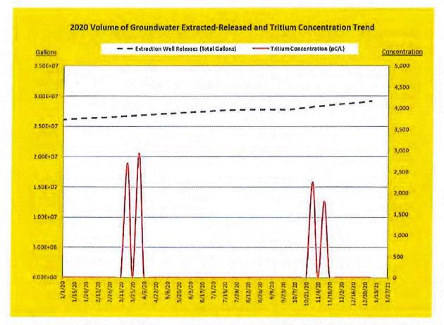
Analysis: the variation in tritium concentration is a function of individual extraction well gallons per minute (GPM) of discharge, simultaneous operation, and the release point.
