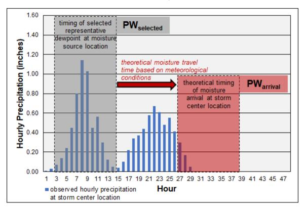
Figure 5-3 Example of Improper Representative Dewpoint Timing Selection Based on Theoretical Moisture Travel Time for Precipitation Event
