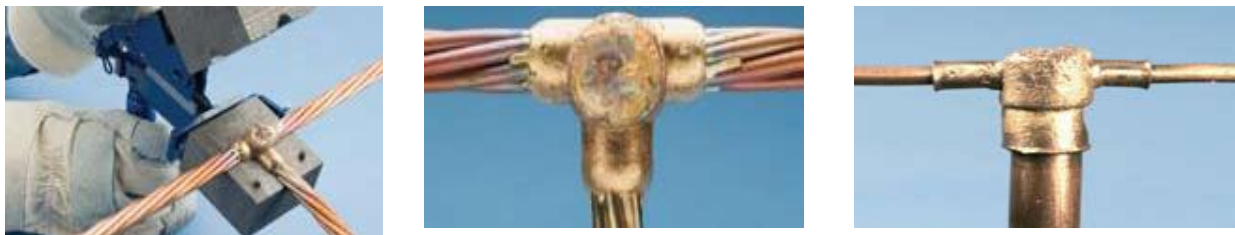
Figure 3: Examples of Cadwelded connections
