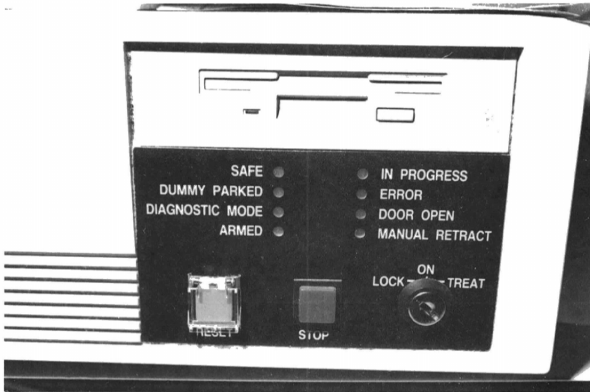
Figure 3.6 Computer Console Status Panel of High Dose Rate Remote Afterloader System
