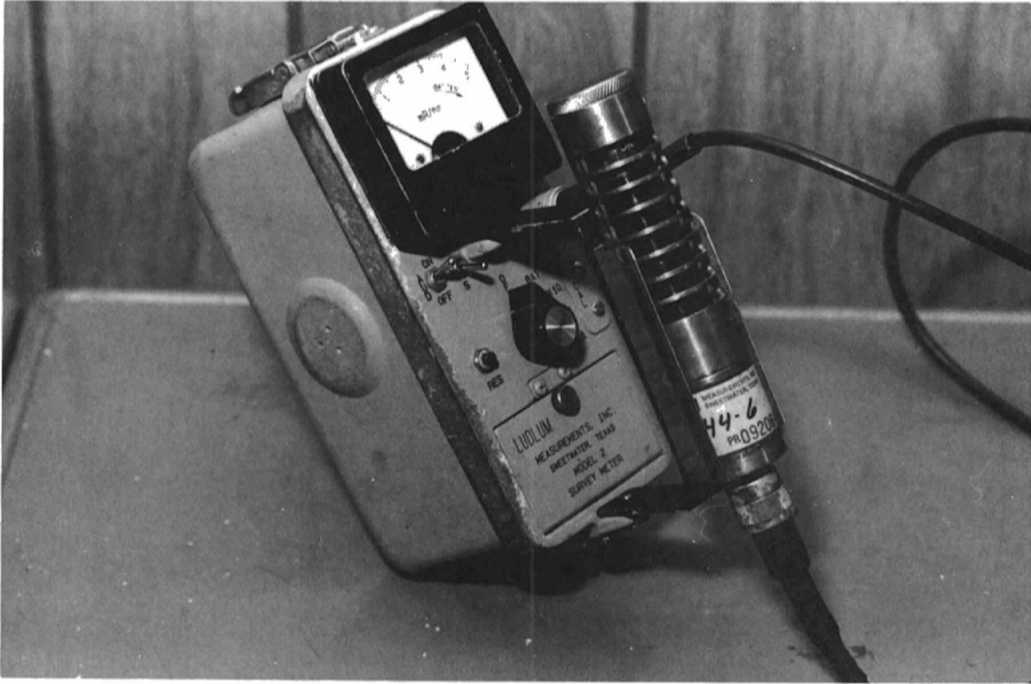
Figure 6.7 Portable Radiation Survey Meter from BFI-Carnegie Straight Truck
