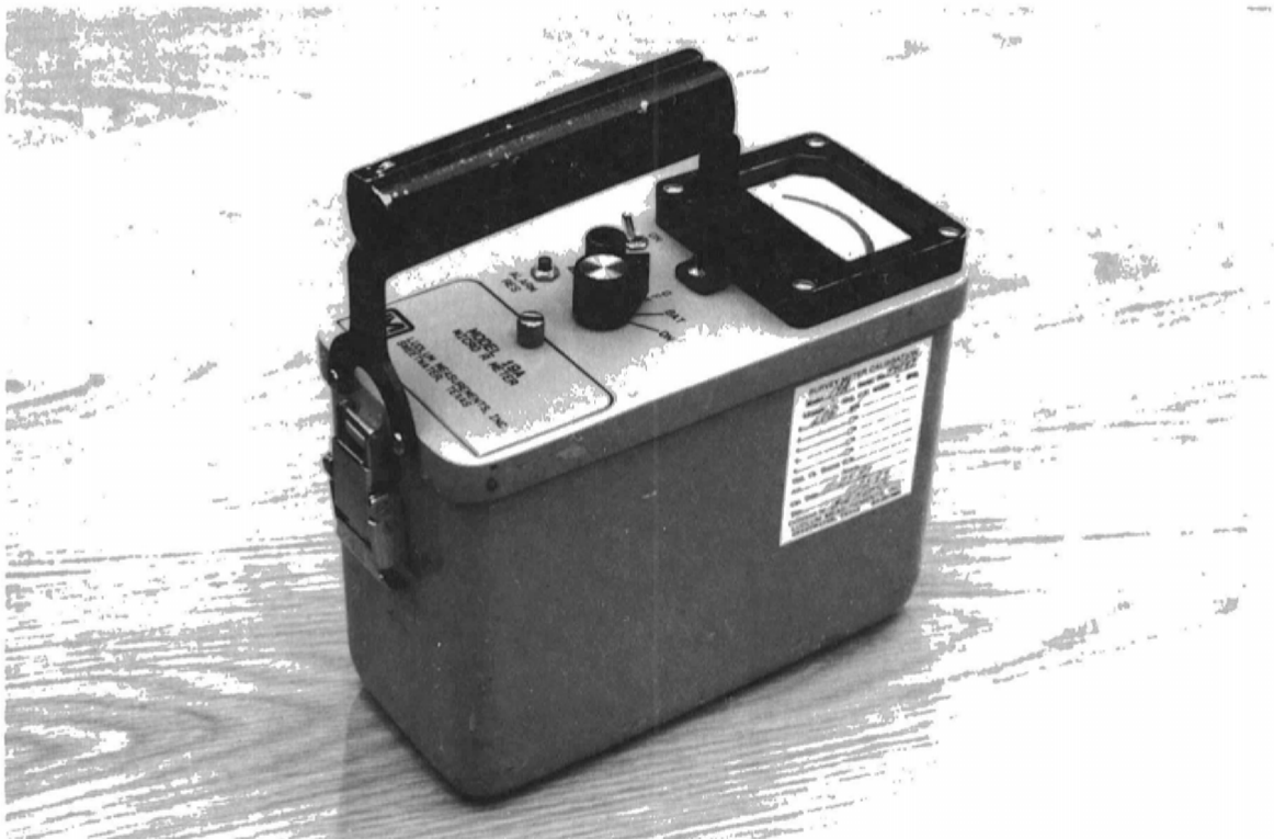
Figure 2.16 Survey Meter Used at BFI – Warren
