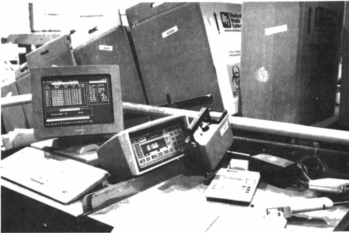
Figure 2.15 Console for Monitoring Radiation at Incinerator Conveyor Feedline
