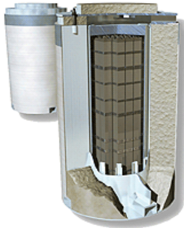
Figure 1-1 Typical Vertical Aboveground Storage Cask System
