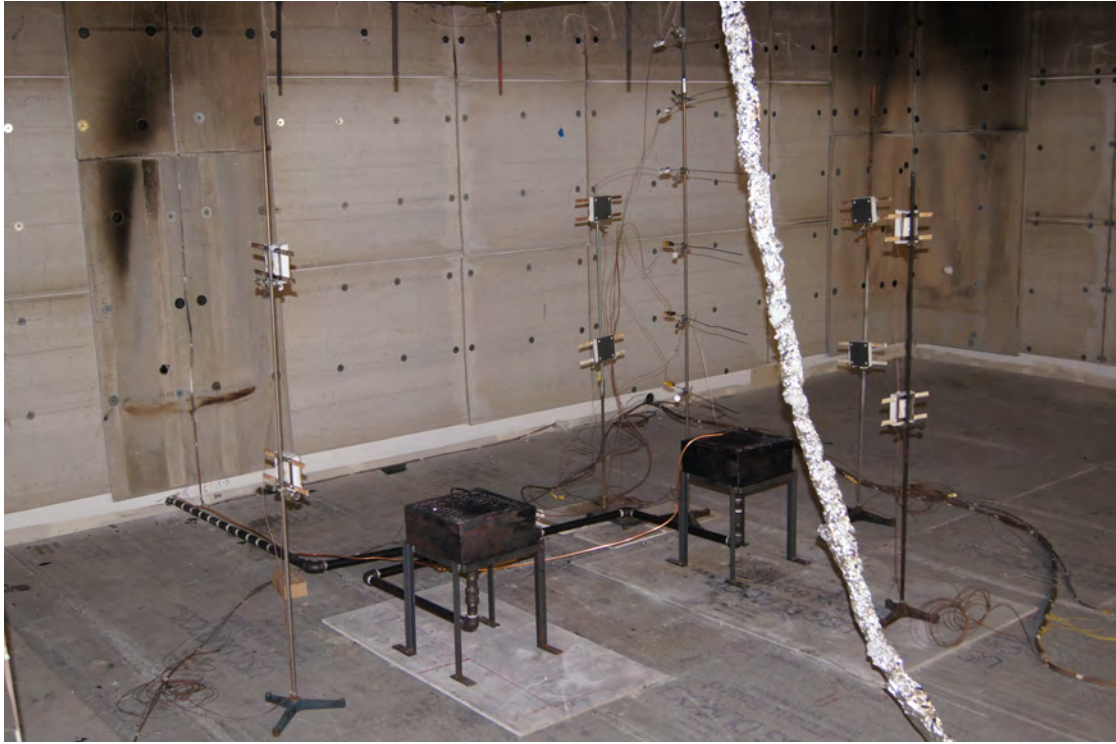
Fig. 27. Configuration of Tests 11 and 12, where the cabinet has been removed.
