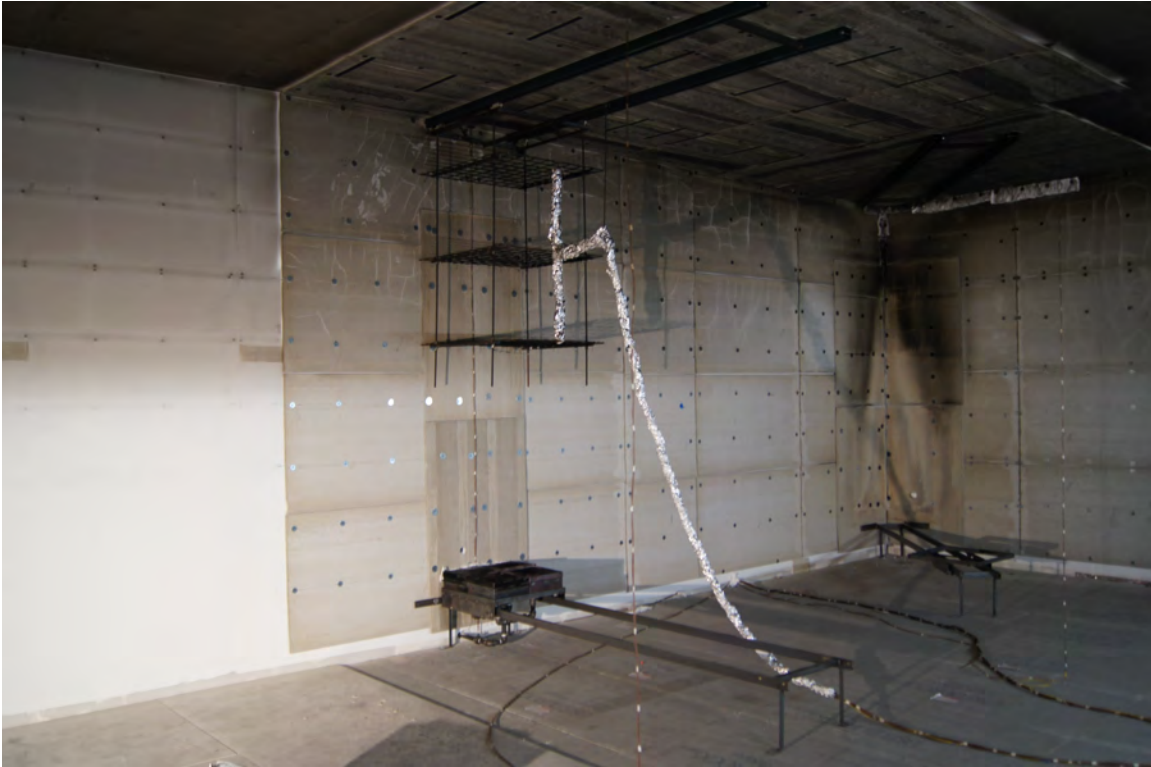
Fig. 5. Photograph of the wall fire experiment.
