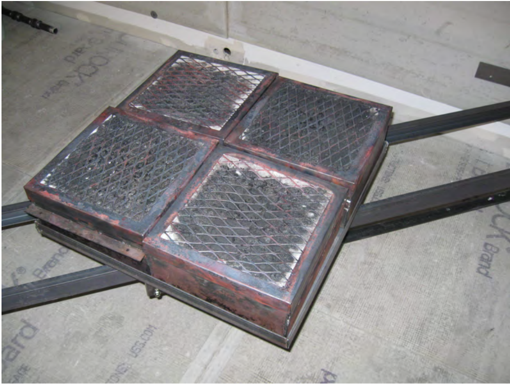
Fig. 2. Photograph of the ganged burners used in the wall and corner experiments.
