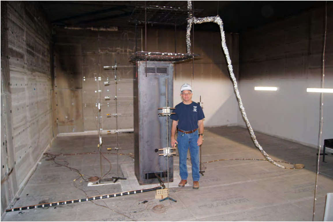
Fig. 18. Photograph of the medium-sized cabinet. Note the position of the thermocouple array just above the front face of the cabinet.
