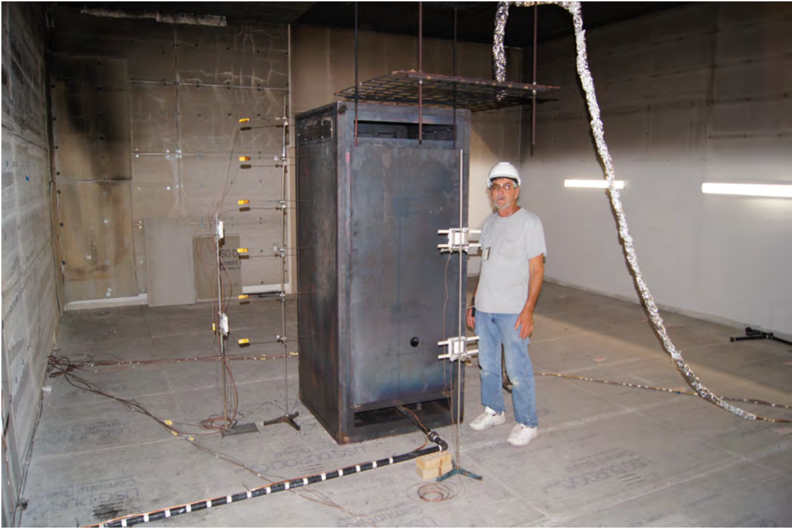
Fig. 16. Photograph of the large cabinet. Note the position of the thermocouple array just above the front face of the cabinet.
