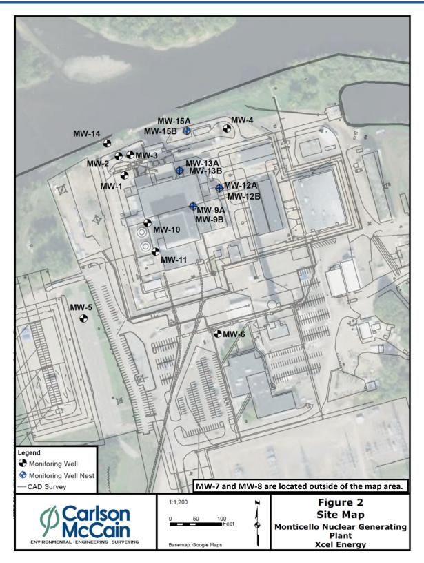
FIGURE 7: MNGP GROUNDWATER MONITORING WELL LOCATIONS (REF. [9]).
