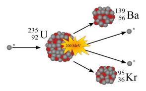
FIGURE 2: EXAMPLE OF A FISSION REACTION. (WIKIMEDIA COMMONS, REF. [12])
