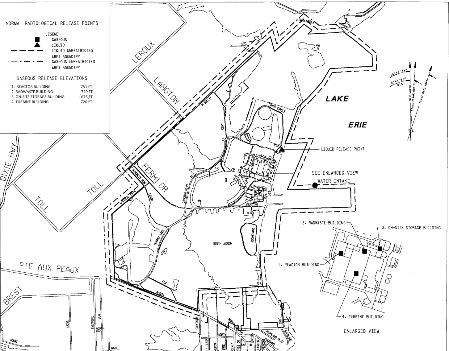
Figure 3.0-1 MAP DEFINING UNRESTRICTED AREA AND SITE BOUNDARY FOR RADIOACTIVE GASEOUS AND LIQUID EFFLUENTS
