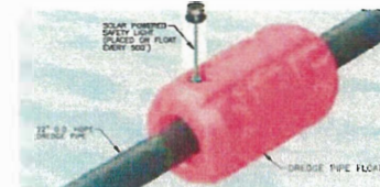
TYPICAL DREDGE PIPE FLOAT DETAIL
