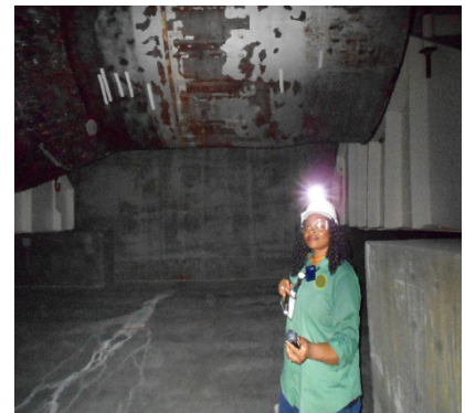
An NRC Inspector verifies dose rates in a steam generator mausoleum at a nuclear power site.
