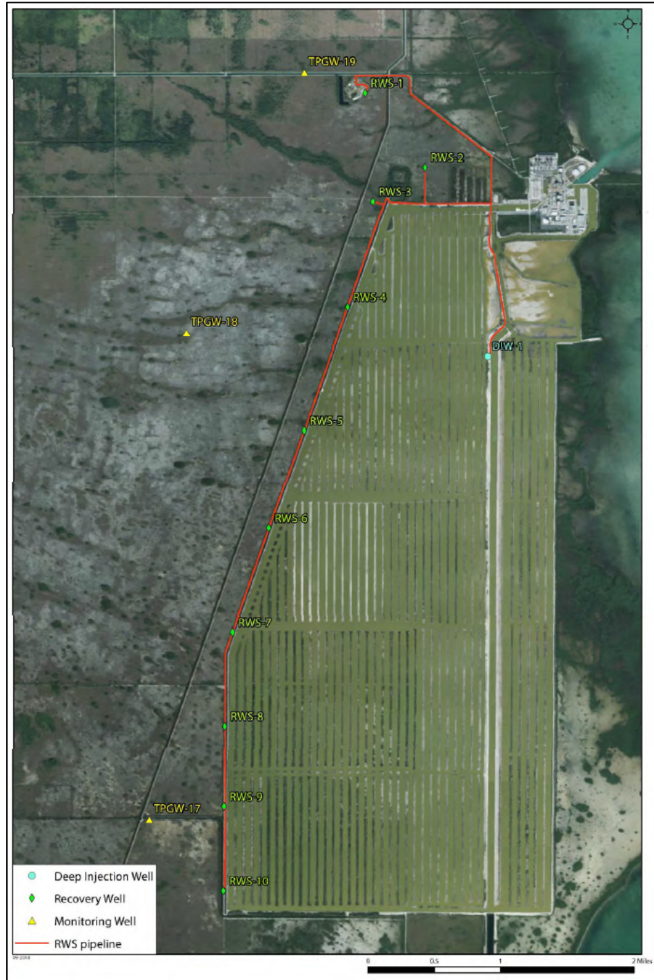
Figure 3-25 Layout of Biscayne Aquifer Recovery Well System and Injection Wells
