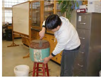
Trimming roughly to take ring-off
