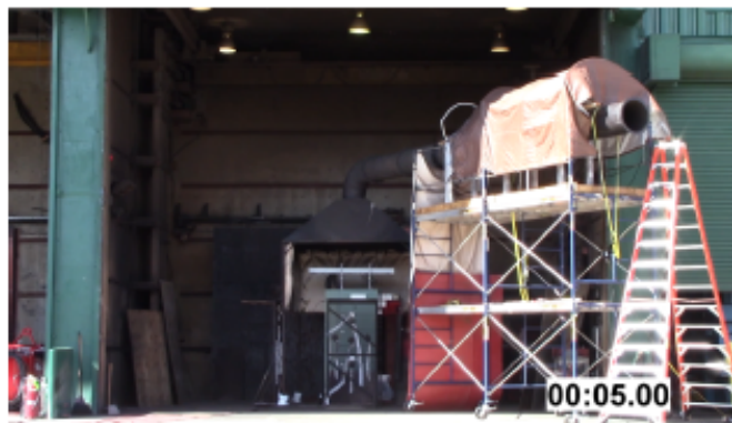
Test #23: 480 V, 40 kA, 7 seconds Aluminum bus bars
