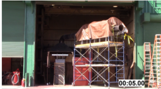
Test #15: 10 kV, 15 kA, 3 seconds Oil-filled breaker (oil removed), copper bus bars
