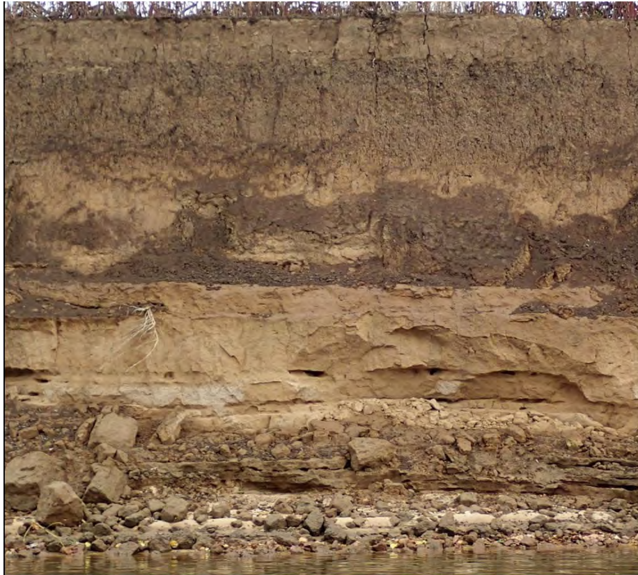
Figure 4-50 Photograph of exposure along the White River near Oil Trough. At this site, recent silt overlies buried soil developed in silt underlain by interbedded silt and sand. No liquefaction feature was found at this or other sites despite conducive sedimentological conditions and very good to excellent exposure. For scale, the cutbank is about 4 m high.
