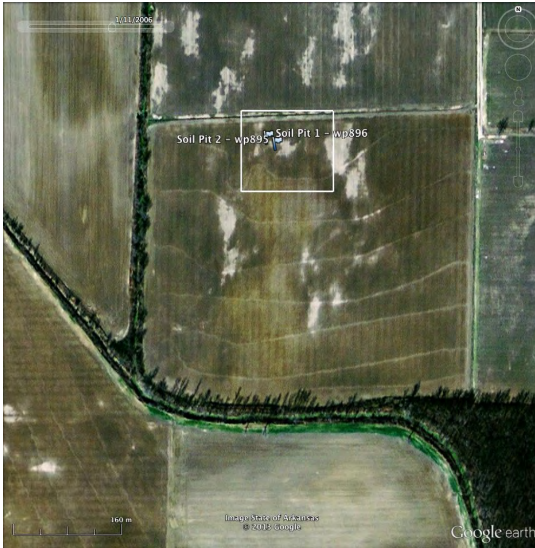
Figure 4-80 GE image showing location of Garner site outlined by solid white line, light-colored patches that cross site, and soil pits (indicated by blue flags) excavated in the patches to evaluate likelihood that they are sand blows. Fields have been graded making sand blows obvious. Lighthouse ditch is drainage south of site. Sand dikes were observed in banks of Lighthouse Ditch during reconnaissance of Late Pleistocene valley-train deposits in 2011. Satellite image was acquired by USDA Farm Service Agency on January 11, 2006.
