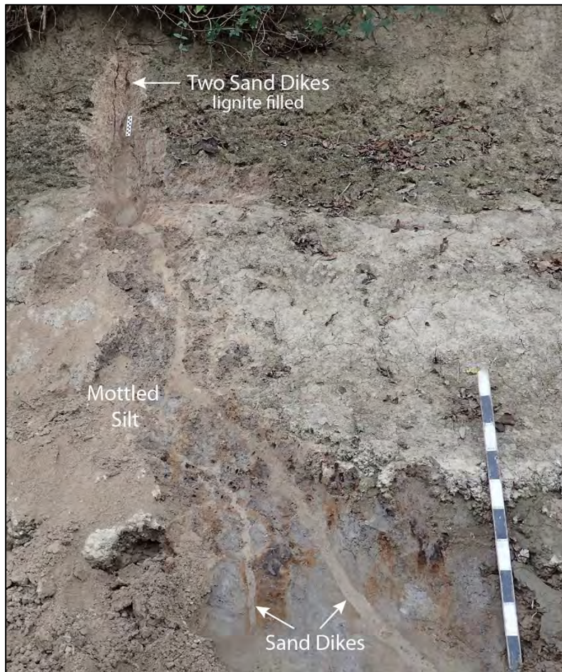
Figure 4-41 Photograph showing relatively unweathered sand dikes at SFR15. Larger dike extends farther up section, where it splits to form two smaller dikes filled with small lignite clasts. Black and white intervals represent 10 cm on meter stick and 1 cm on small scale near split of dike into two smaller dikes.
