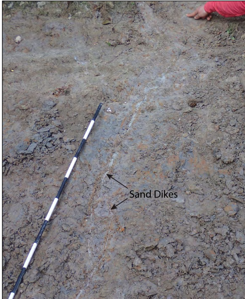
Figure 4-30 Photograph of small sand dike at CWR7. The black and white intervals on the meter stick represent 10 cm. S. Bastin points to the dike tip or termination.
