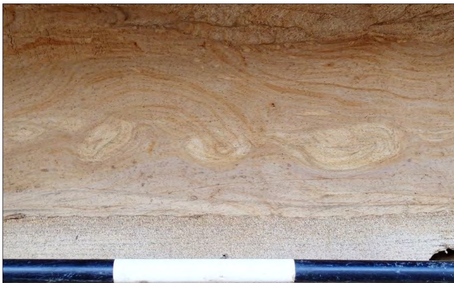
Figure 4-54 Photograph of pseudonodules in Late Pleistocene sediment exposed at WR109. For scale, white interval of meter stick is 10 cm long.
