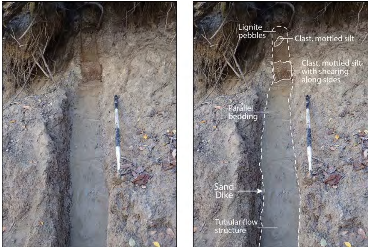
Figure 4-43 Photographs (left - unannotated; right - annotated) showing sand dike with blunt termination at SFR25. Large clasts of mottled silt appear to have collapsed into the dike from above. Horizontal layering as well as tubular flow structure occur within the dike. The upper part of the dike was iron stained, mottled, and contained small manganese nodules. Dashed lines represent clear contacts. Black and white intervals on hoe represent 25 cm.
