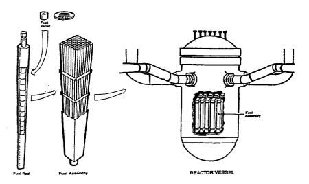
Figure 6: The reactor core at Davis-Besse contains 177 fuel assemblies. Each assembly contains 208 fuel rods. Each fuel rod is filled with approximately five pounds of fuel pellets. Each pellet is approximately 3/8 inch diameter and 5/8 inch long.
