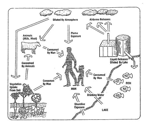
Figure 29: The exposure pathways shown here are monitored through the Radiological Environmental Monitoring Program (REMP) and are considered when calculating doses to the public.
