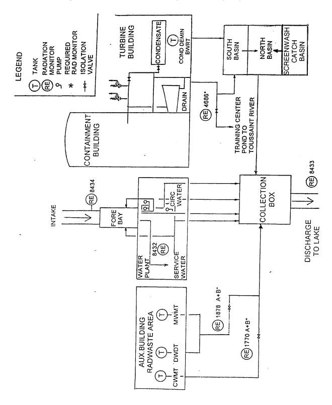
Liquid Radioactive Effluent Monitoring and Processing Diagram
