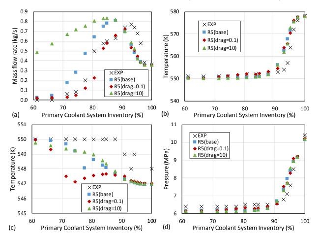
Figure 19 Comparison Between Relap5 Sensitivity Calculations Varying Drag Coefficient (0.1 to 10) and Experiment for S-NC-2 Test as a Function of Primary Coolant System Inventory: (a) Primary System Mass Flowrate, (b) Hot Leg Fluid Temperature, (c) SG Outlet Temperature, (d) Primary Pressure
