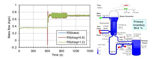
Figure 9 Mass Flowrate Dependence on 20% Drag Coefficient Variation for S-NC-2 Test Case C7\_P-90.9% (left) and Liquid Distribution at 1500 S for Base Case (right)
