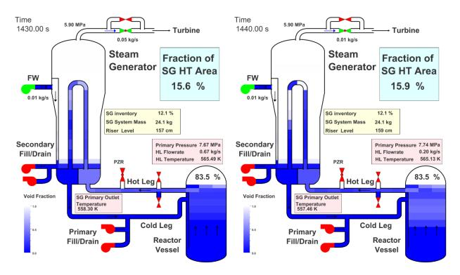
Figure 39 Animation Mask for S-NC-03 Calculated Case C19\_S-15.2% with Primary Side Filled as in S-NC-02\_P-83.6% at 1430 s (left) and 1440 s
