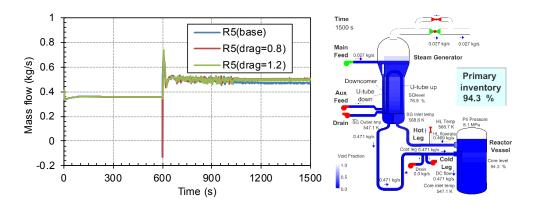
Figure 7 Mass Flowrate Dependence on 20% Drag Coefficient Variation for S-NC-2 Test Case C5\_P-94.2% (left) and Liquid Distribution at 1500 S for Base Case (right)
