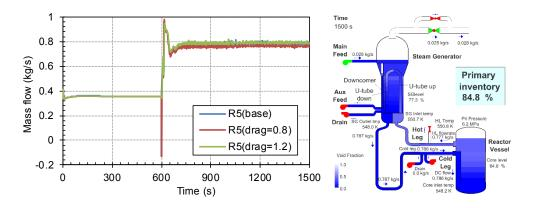
Figure 11 Mass Flowrate Dependence on 20% Drag Coefficient Variation for S-NC-2 Test Case C9\_P-84.8% (left) and Liquid Distribution at 1500 S for Base Case (right)
