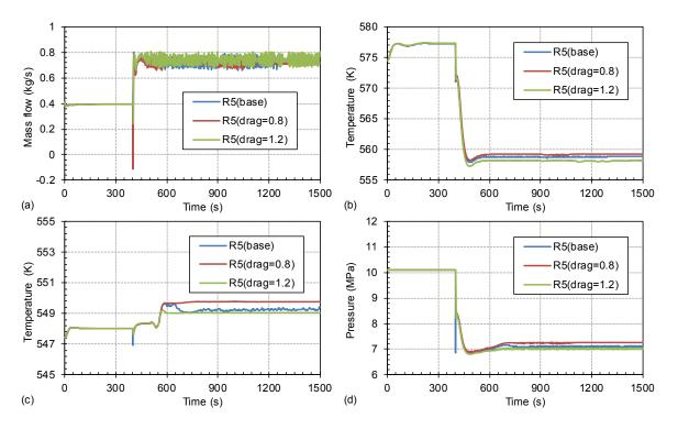
Figure 30 Sensitivity Calculations Varying Drag Coefficient for S-NC-3 Test Case C16\_S-43.6%: (a) Primary System Mass Flowrate, (b) Hot Leg Fluid Temperature, (c) SG Outlet Temperature, (d) Primary Pressure
