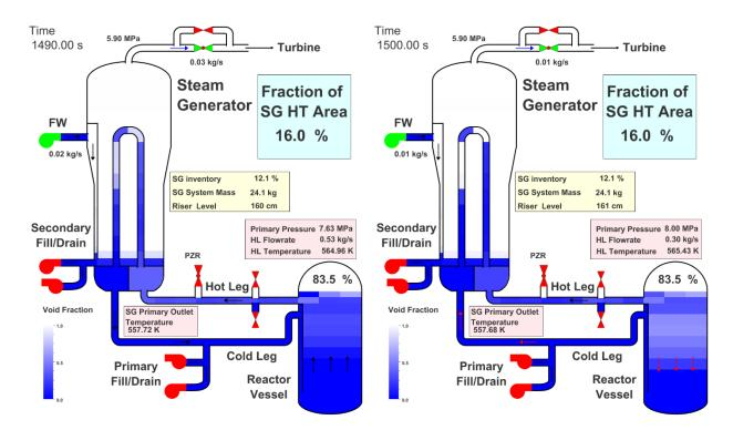
Figure 42 Animation Mask for S-NC-03 Calculated Case C19\_S-15.2% with Primary Side Filled as in S-NC-02\_P-83.6% at 1490 s (left) and 1500 s (right)
