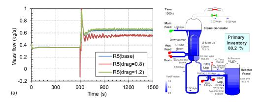
Figure 13 Mass Flowrate Dependence on 20% Drag Coefficient Variation for S-NC-2 Test Case C11\_P-80.6% (left) and Liquid Distribution at 1500 S for Base Case (right)
