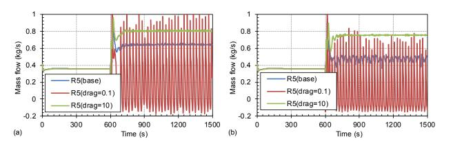
Figure 25 Mass Flowrate Dependence on Dial Value Drag Coefficient Variation for S-NC-2 Test Cases: (a) C11\_P-80.6% and (b) C12\_P-77.6%
