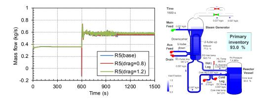
Figure 8 Mass Flowrate Dependence on 20% Drag Coefficient Variation for S-NC-2 Test Case C6\_P-93.1% (left) and Liquid Distribution at 1500 S for Base Case (right)
