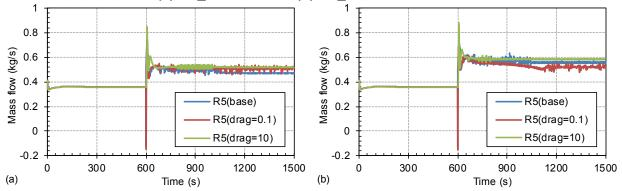
Figure 22 Mass Flowrate Dependence on Dial Value Drag Coefficient Variation for S-NC-2 Test Cases: (a) C5\_P-94.2% and (b) C6\_P-93.1%
