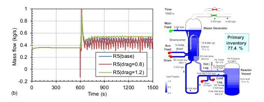
Figure 14 Mass Flowrate Dependence on 20% Drag Coefficient Variation for S-NC-2 Test Case C12\_P-77.6% (left) and Liquid Distribution at 1500 S for Base Case (right)
