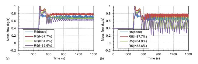
Figure 36 Mass Flowrate Dependence on Initial Primary Coolant System Inventory for S-NC-3 Test Cases: (a) C16\_S-43.6% and (b) C17\_S-33.2%
