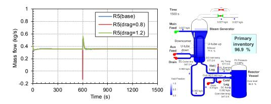
Figure 4 Mass Flowrate Dependence on 20% Drag Coefficient Variation for S-NC-2 Test Case C2\_P-97.6% (left) and Liquid Distribution at 1500 s for Base Case (right)
