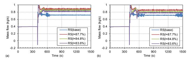
Figure 35 Mass Flowrate Dependence on Initial Primary Coolant System Inventory for S-NC-3 Test Cases: (a) C14\_S-67.4% and (b) C15\_S-55.5%
