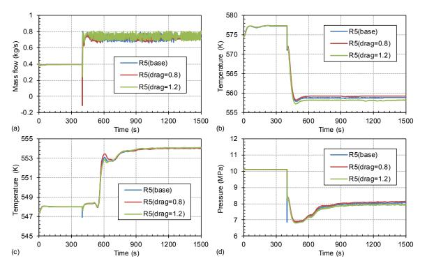
Figure 31 Sensitivity Calculations Varying Drag Coefficient for S-NC-3 Test Case C19\_S-15.2%: (a) Primary System Mass Flowrate, (b) Hot Leg Fluid Temperature, (c) SG Outlet Temperature, (d) Primary Pressure
