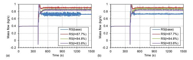
Figure 33 Mass Flowrate Dependence on Initial Primary Coolant System Inventory for S-NC-3 Test Cases: (a) C10\_S-100.0% and (b) C11\_S99.1%
