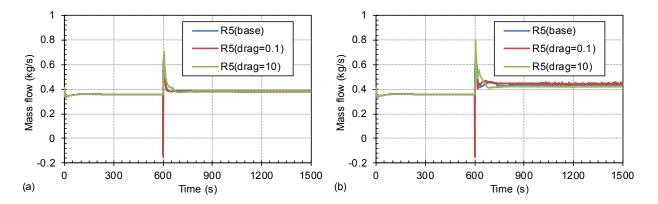
Figure 21 Mass Flowrate Dependence on Dial Value Drag Coefficient Variation for S-NC-2 Test Cases: (a) C3\_P-96.3% and (b) C4\_P-95.2%
