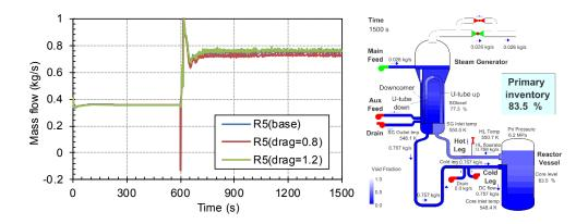
Figure 12 Mass Flowrate Dependence on 20% Drag Coefficient Variation for S-NC-2 Test Case C10\_P-83.6% (left) and Liquid Distribution at 1500 S for Base Case (right)
