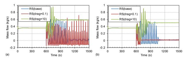
Figure 27 Mass Flowrate Dependence on Dial Value Drag Coefficient Variation for S-NC-2 Test Cases: (a) C15\_P-66.3% and (b) C16\_P-61.2%
