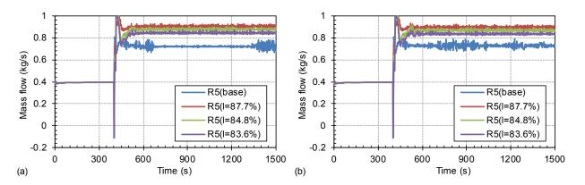
Figure 34 Mass Flowrate Dependence on Initial Primary Coolant System Inventory for S-NC-3 Test Cases: (a) Cases C12\_S-86.9% and (b) C13\_S-75.5%
