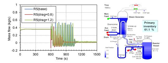
Figure 18 Mass Flowrate Dependence on 20% Drag Coefficient Variation for S-NC-2 Test Case C16\_P-61.2% (left) and Liquid Distribution at 1500 S for Base Case (right)
