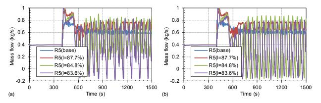
Figure 37 Mass Flowrate Dependence on Initial Primary Coolant System Inventory for S-NC-3 Test Cases: (a) C18\_S-22.7% and (b) C19\_S-15.2%
