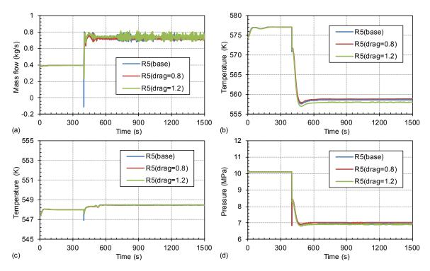
Figure 29 Sensitivity Calculations Varying Drag Coefficient for S-NC-3 Test Case C13\_S-75.5%: (a) Primary System Mass Flowrate, (b) Hot Leg Fluid Temperature, (c) SG Outlet Temperature, (d) Primary Pressure
