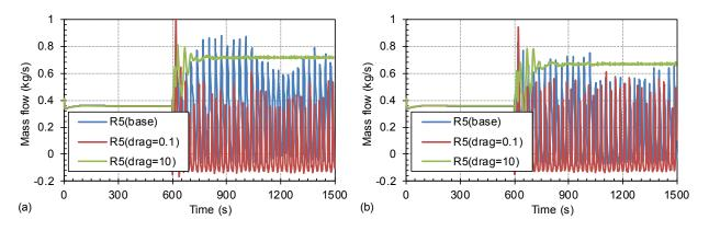
Figure 26 Mass Flowrate Dependence on Dial Value Drag Coefficient Variation for S-NC-2 Test Cases: (a) C13\_P-74.4% and (b) C14\_P-71.4%
