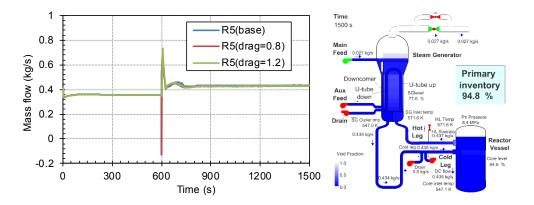
Figure 6 Mass Flowrate Dependence on 20% Drag Coefficient Variation for S-NC-2 Test Case C4\_P-95.2% (left) and Liquid Distribution at 1500 S for Base Case (right)
