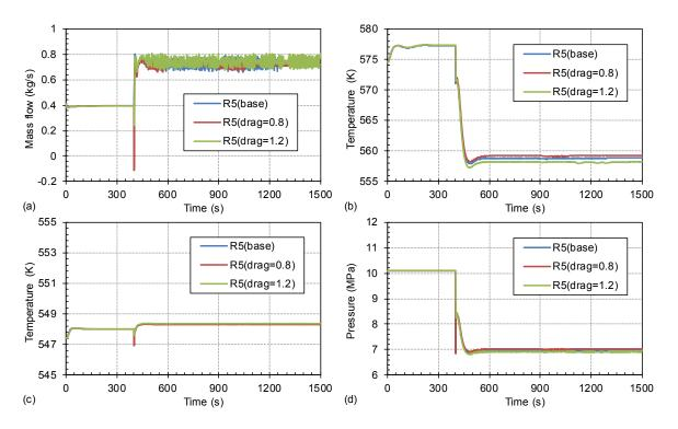
Figure 28 Sensitivity Calculations Varying Drag Coefficient for S-NC-3 Test Case C10\_S-100.0%: (a) Primary System Mass Flowrate, (b) Hot Leg Fluid Temperature, (c) SG Outlet Temperature, (d) Primary Pressure
