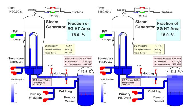
Figure 40 Animation Mask for S-NC-03 Calculated Case C19\_S-15.2% with Primary Side Filled as in S-NC-02\_P-83.6% at 1450 s (left) and 1460 s
