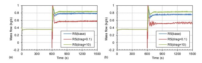
Figure 24 Mass Flowrate Dependence on Dial Value Drag Coefficient Variation for S-NC-2 Test Cases: (a) C9\_P-84.8% and (b) C10\_P-83.6%
