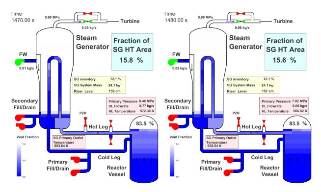
Figure 41 Animation Mask for S-NC-03 Calculated Case C19\_S-15.2% with Primary Side Filled as in S-NC-02\_P-83.6% at 1470 s (left) and 1480 s
