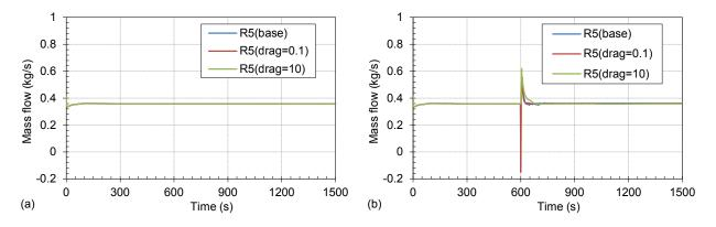
Figure 20 Mass Flowrate Dependence on Dial Value Drag Coefficient Variation for S-NC-2 Test Cases: (a) C1\_P-100.0% and (b) C2\_P-97.6%
