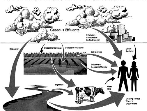
Graphic 1. Examples of Gaseous and Liquid Effluent Pathways
