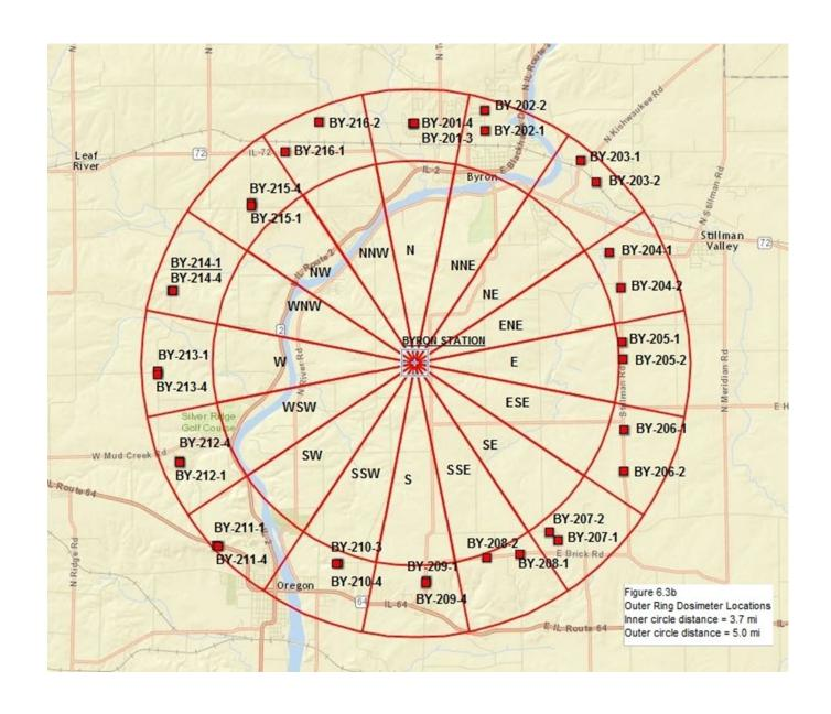
Figure B-2 Outer Ring OSLD Locations of the Byron Nuclear Generating Station, 2018
