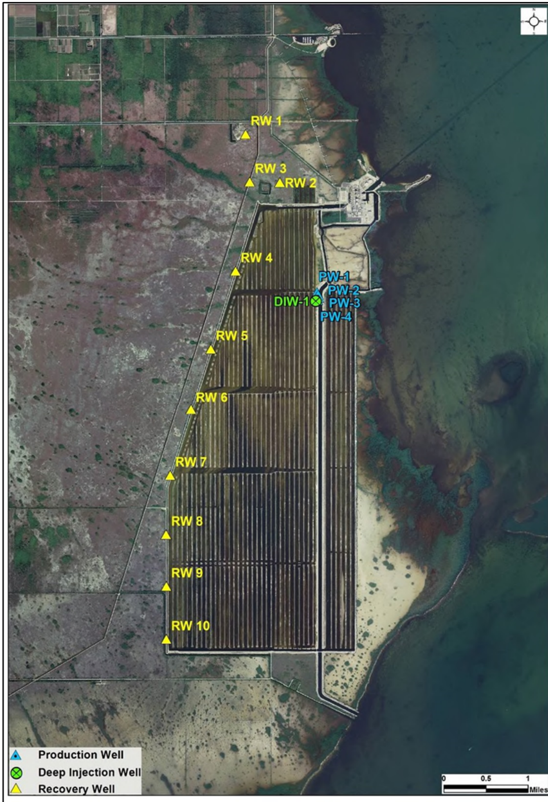
Figure 3-14 Layout of Biscayne Aquifer Recovery Well System and Testing Wells
