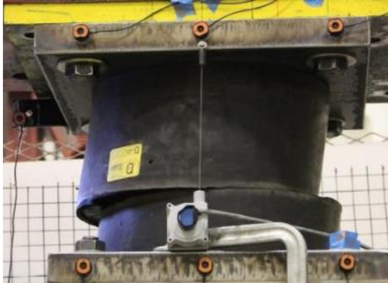
Figure 7-36 Slippage across the damaged interface of bearing MA4 in a shear test (axial pressure = 0.5 MPa)
