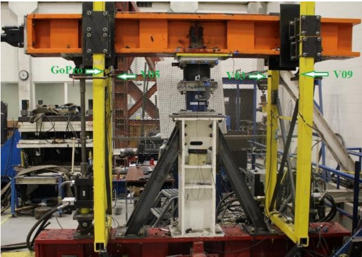
Figure 6-17 Location of the four cameras on the columns of the SBTM
