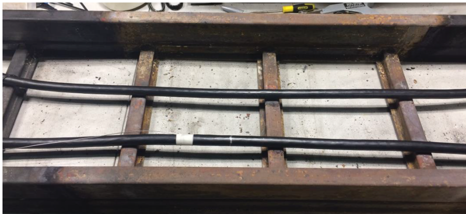
Figure 3-13 Representative Cable Setup Illustrating TC Placement (Test 21)
