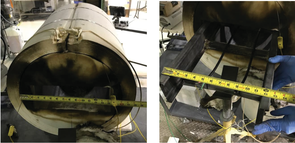
Figure 3-5 Picture of Cable Test Setup (Left) and Ceramic Heater (Right)
