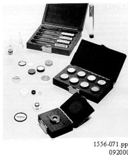
Figure 5-6. Calibration Standards. Certain calibration and reference sources containing americium-241 (Am-241) or Ra-226 can be possessed under a general license authorized in 10 CFR 31.8 by those otherwise specifically licensed.
