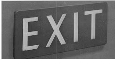
Figure F-3. Self-Luminous Exit Sign. Certain self-luminous, tritium exit signs can be possessed under 10 CFR 31.5. (Typical devices initially contain 25 curies of tritium per sign.)
