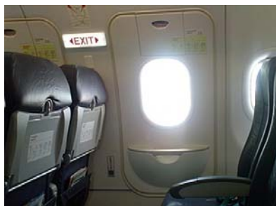
Figure 5-5. Luminous Exit Sign. Safety devices, such as luminous exit signs, containing tritium or Pm-147 that are used in aircraft may be used under the 10 CFR 31.7 general license.
