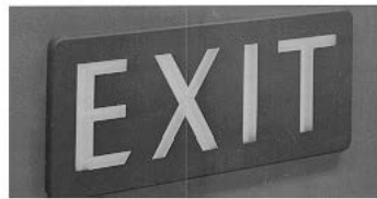
Figure G–1. Self-Luminous Exit Sign. Certain self-luminous, tritium exit signs can be possessed under Title 10 of the Code of Federal Regulations (10 CFR) 10 CFR 31.5, “Certain detecting, measuring, gauging, or controlling devices and certain devices for producing light or an ionized atmosphere.” (Typical devices initially contain 25 curies of tritium per sign.)
