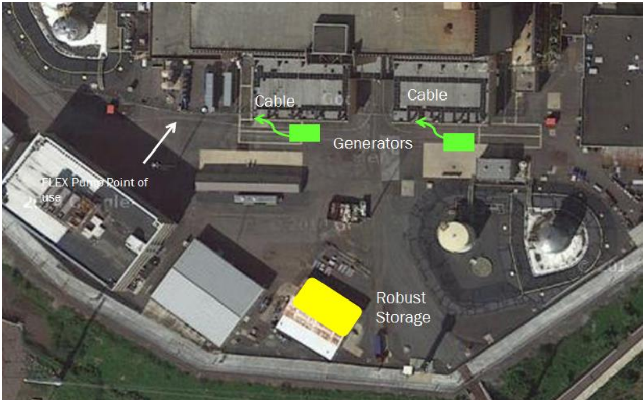
Figure 14 - FLEX Generator Storage Building and Haul Route
