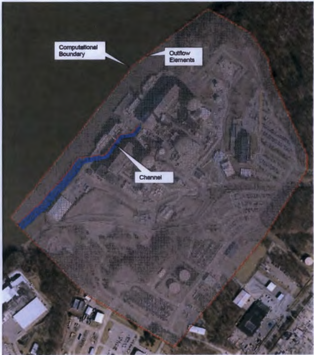
Figure 3.2-1. Map Showing Boundary of FLO-2D Model Used to Calculate Local Intense Precipitation Flood at the Indian Point Energy Center Site. Source: Entergy (2014c)
