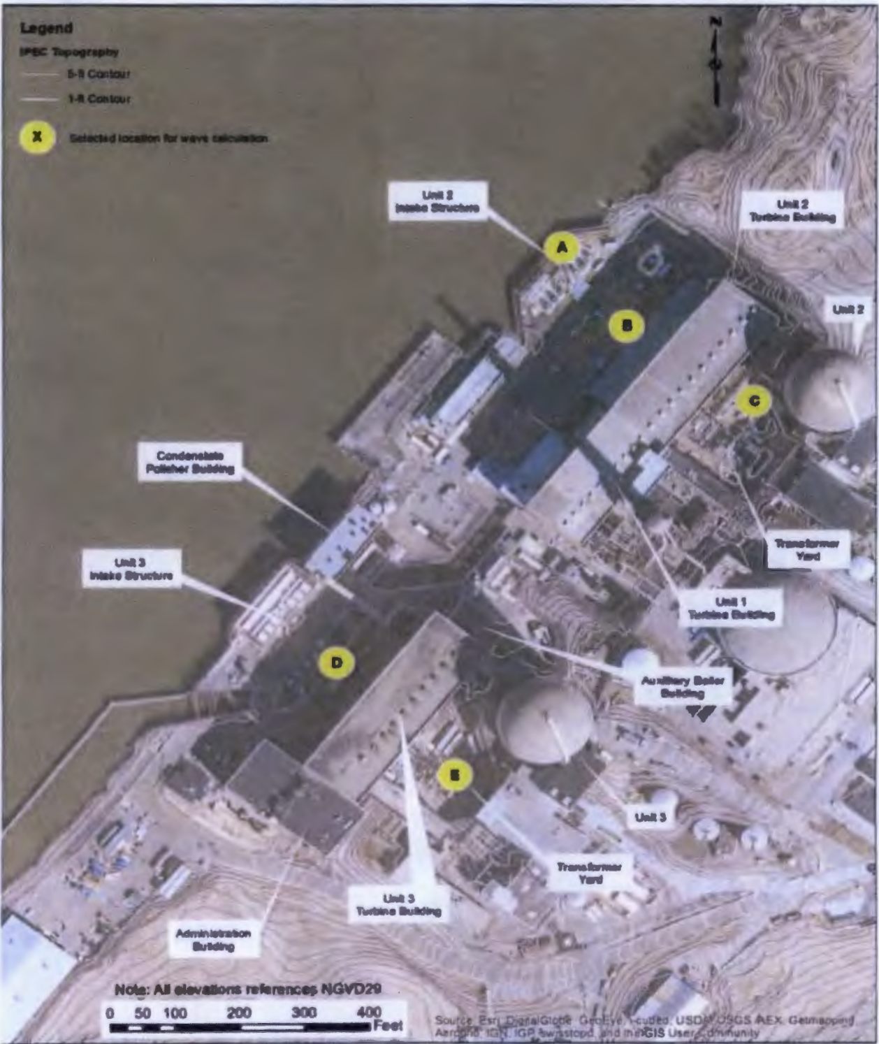
Figure 3.5-1. Figure Showing Locations of Reported WSEs for the Storm Surge Flood Reevaluation at the Indian Point Energy Center Site. Locations are Indexed to Table 3.5-1. Source: Entergy (2016a)
