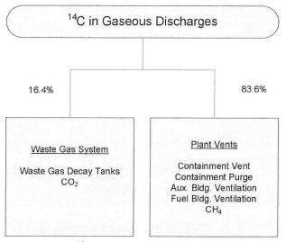
Figure 2: <sup>14</sup>C Gaseous Discharge Balance
