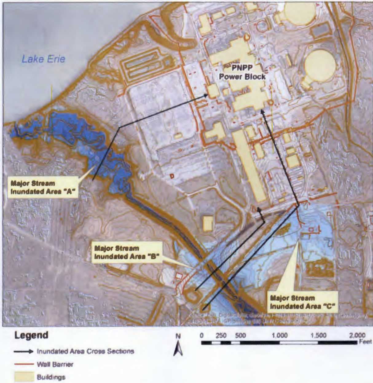
Figure 3.6.4 Perry Nuclear Power Plant Major Stream Combined Effect Inundation Area (Source: FENOC Audit –Licensee generated figure. Used with approval. See Section 4)
