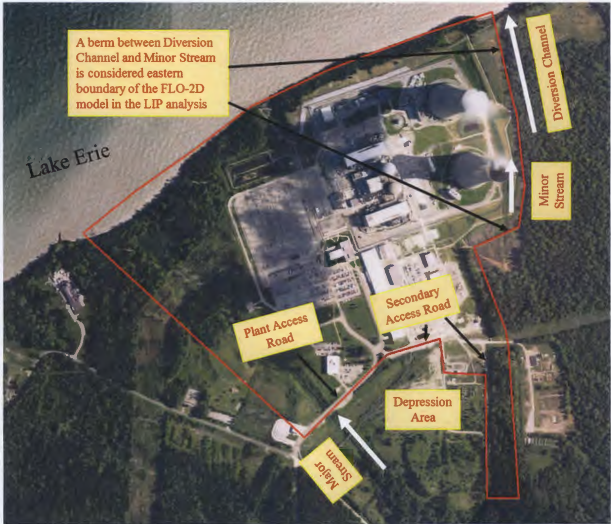
Figure 3.2-2. LIP FLO-2D model domain showing Major Stream, Minor Stream, Diversion Channel, Plant Access Road, Secondary Access Road and Depression Area.
