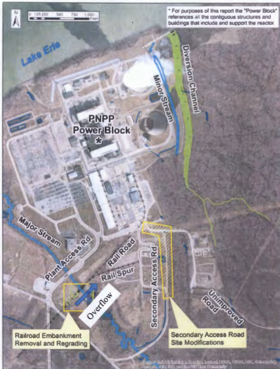
Figure 3.3-1. Site layout showing Major Stream, Minor Stream, Diversion Channel (Re-aligned Channel), Secondary Access Road, and overbank flow (see the blue arrow) that would occur when the model is driven by the ORNL's ssPMP. (Modified from Figure 2.0.1, FHRR, Revision 1)
