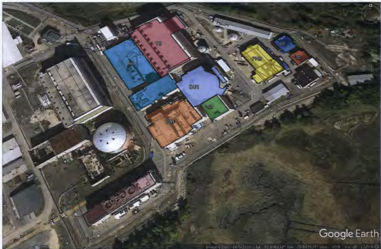
Figure 3.1-2. Seabrook site (adapted from FHRR Figure 4-1); Intake Building (IB), Discharge Building (DB), Pump House Building (PHB), Fuel Storage Building (FSB), Containment Unit 1 (CU1), Turbine Building (TB), Administration Building (AB), Waste Handling Building (WB), Cooling Tower (CT) are shown.
