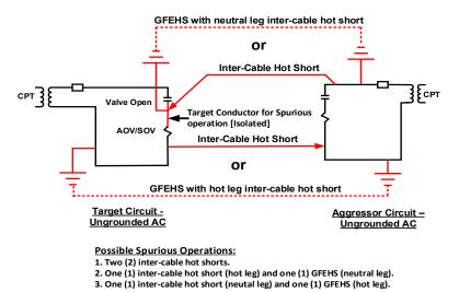
Figure 3-2 Sub-Case 2 – Multiple Inter-cable Hot Shorts or Single Inter-cable Hot Short and GFEHS
