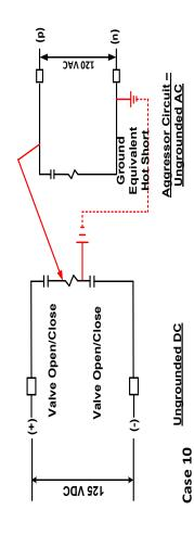
Figure C-3 Ungrounded DC – Double Break Design (Continued)
