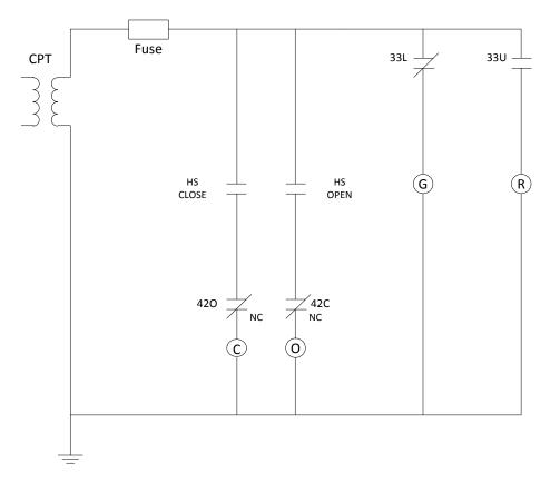
Figure 4-1 Simplified MOV Circuit
