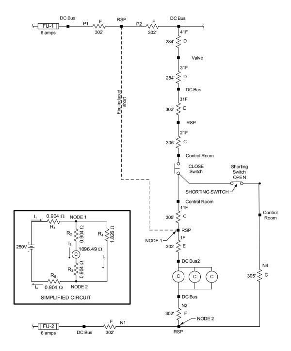
Figure 4-7 Simplified Circuit (Lumped Model)
