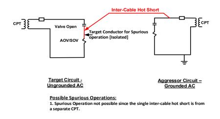
Figure 3-1 Sub-Case 1 – Single Inter-cable Hot Short
