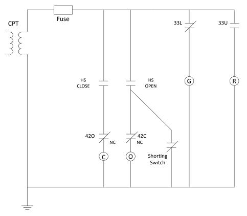
Figure 4-2 Simplified MOV Circuit with Shorting Switch
