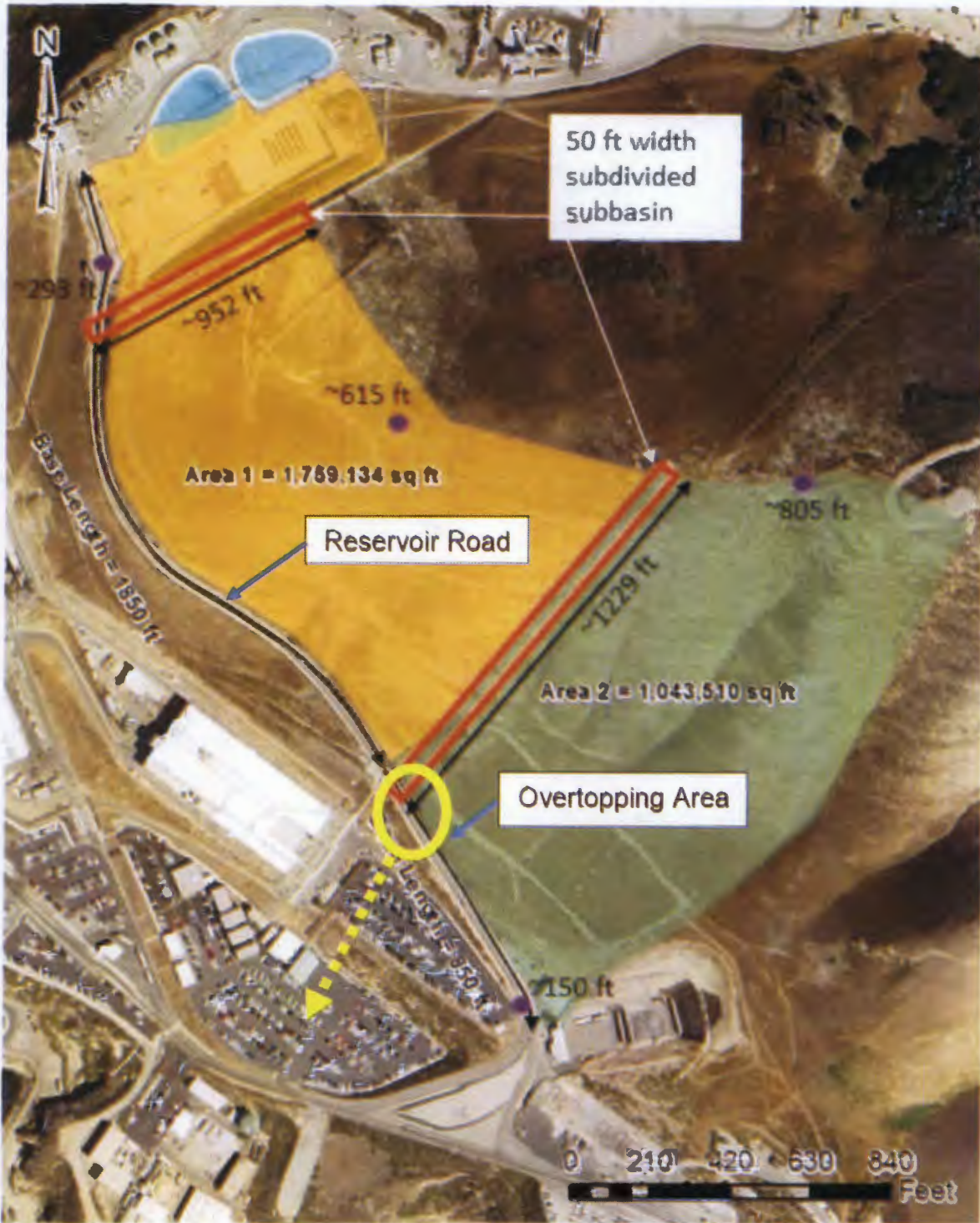
Figure 3.2-4. Additional watershed areas east of the Reservoir Road evaluated to determine their contribution to LIP water surface elevation estimates. Location of overtopping area estimated by the licensee using the HEC-HMS computer code. Source: PG&E (2017a)
