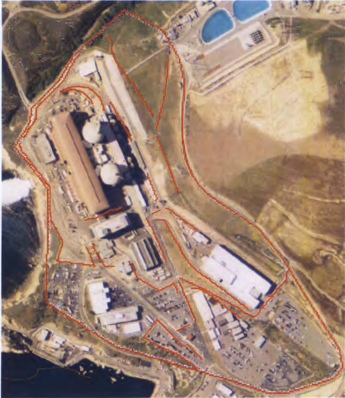
Figure 3.2-2. Site map with showing the boundary of the refined FLO-2D LIP model (outside red line) and surface-based features within the powerblock such as levees and the VBS (also depicted as red lines). Source: PG&E (2017b).
