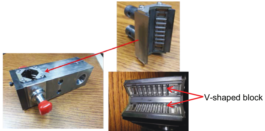
Figure 6 Assembled grip blocks (left) and two views (right) of detached grip body
