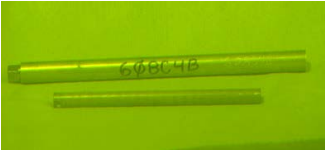
Figure 13 Segment 608C4B for DL2 taken from rod G10, with the storage tube
