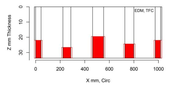
Figure H.294 Indication Plot for Procedure MM.28.1 Applied to Test Block P4 in PARENT Open Testing (X – Z view)
