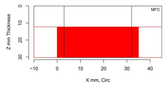
Figure H.286 Indication Plot for Procedure MM.28.1 Applied to Test Block P30 in PARENT Open Testing (X – Z view)
