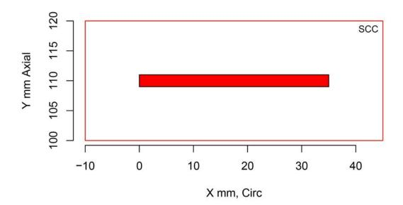
Figure H.283 Indication Plot for Procedure MM.28.1 Applied to Test Block P29 in PARENT Open Testing (X – Y view)
