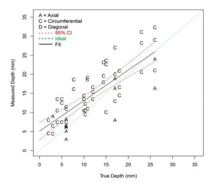
Figure F.23 Depth Sizing Regression (in mm) for ADVPAUT Procedures SBDMW Test Blocks in PARENT Open Testing (O.D. access – w/ FB test blocks)
