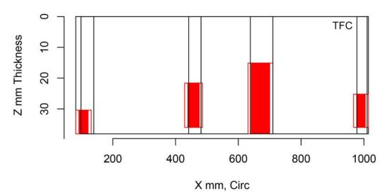
Figure H.172 Indication Plot for Procedure ECT.16 Applied to Test Block P1 in PARENT Open Testing (X – Z view)
