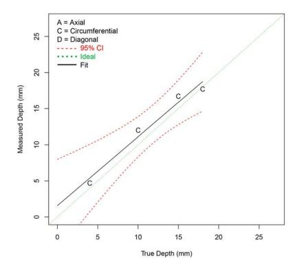
Figure F.65 Depth Sizing Regression (in mm) for Procedure SAFT.17 on FB Test Blocks in PARENT Open Testing (O.D. access)
