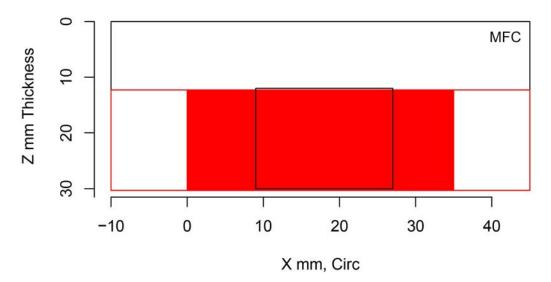
Figure H.114 Indication Plot for Procedure PAUT.122.1 Applied to Test Block P30 in PARENT Open Testing (X – Z view)
