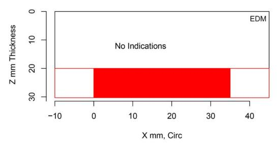
Figure H.64 Indication Plot for Procedure RT.109 Applied to Test Block P42 in PARENT Open Testing (X – Z view)
