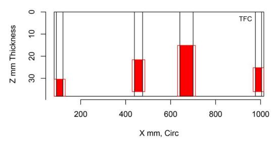
Figure H.292 Indication Plot for Procedure MM.28.1 Applied to Test Block P1 in PARENT Open Testing (X – Z view)
