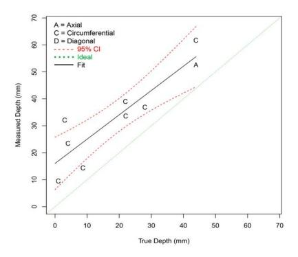
Figure F.87 Depth Sizing Regression (in mm) for Procedure SAFT.17 on LBDMW Test Blocks in PARENT Open Testing (O.D. access)
