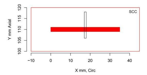
Figure H.119 Indication Plot for Procedure PAUT.122.2 Applied to Test Block P31 in PARENT Open Testing (X – Y view)
