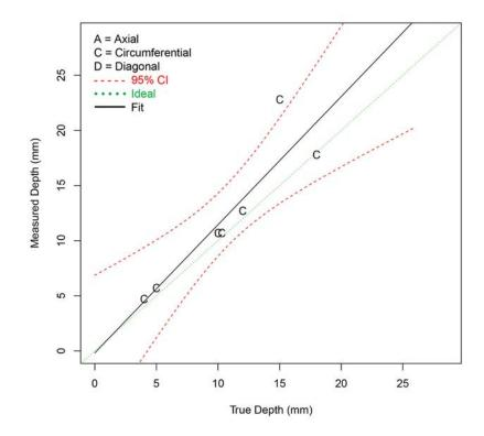
Figure F.31 Depth Sizing Regression (in mm) for Procedure PAATOFD.29.2 on SBDMW Test Blocks in PARENT Open Testing (I.D. access – w/ FB test blocks)
