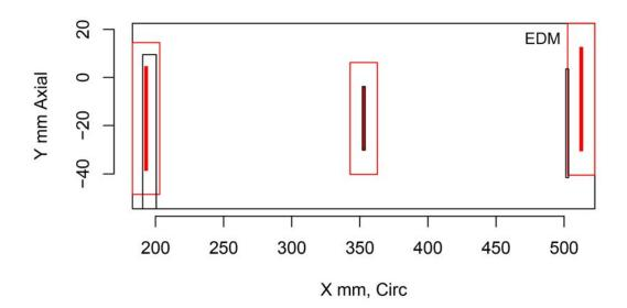
Figure H.201 Indication Plot for Procedure SAFT.17 Applied to Test Block P23 in PARENT Open Testing (X – Y view)
