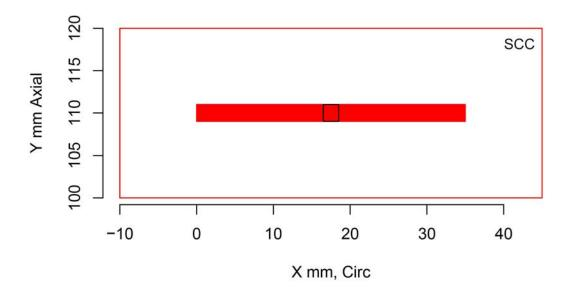
Figure H.135 Indication Plot for Procedure PAUT.131.1 Applied to Test Block P29 in PARENT Open Testing (X – Y view)
