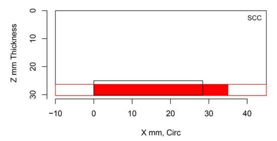
Figure H.246 Indication Plot for Procedure UIR.20 Applied to Test Block P31 in PARENT Open Testing (X – Z view)
