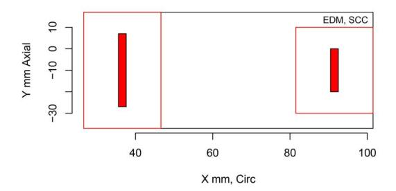
Figure H.371 Indication Plot for Procedure PAATOFD.29.2 Applied to Test Block P12 in PARENT Open Testing (X – Y view)
