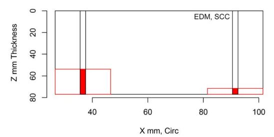
Figure H.200 Indication Plot for Procedure SAFT.17 Applied to Test Block P12 in PARENT Open Testing (X – Z view)
