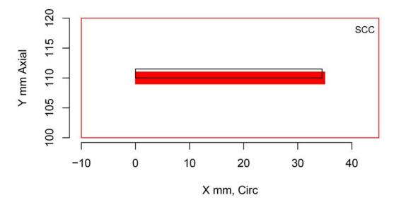
Figure H.435 Indication Plot for Procedure SHPA.6.1 Applied to Test Block P28 in PARENT Open Testing (X – Y view)
