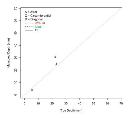
Figure F.86 Depth Sizing Regression (in mm) for ProcedurePAUT.150 on LBDMW Test Blocks in PARENT Open Testing (O.D. access)
