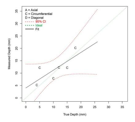
Figure F.27 Depth Sizing Regression (in mm) for UIR Procedures SBDMW Test Blocks in PARENT Open Testing (O.D. access – w/ FB test blocks)
