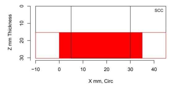
Figure H.416 Indication Plot for Procedure AECT.33 Applied to Test Block P32 in PARENT Open Testing (X – Z view)
