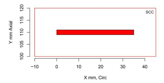
Figure H.225 Indication Plot for Procedure LASH.18 Applied to Test Block P32 in PARENT Open Testing (X – Y view)
