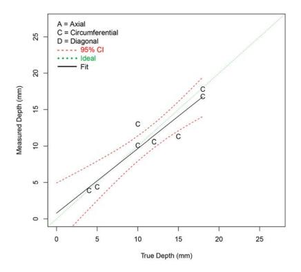
Figure F.73 Depth Sizing Regression (in mm) for RT Procedures on FB Test Blocks in PARENT Open Testing (O.D. access)
