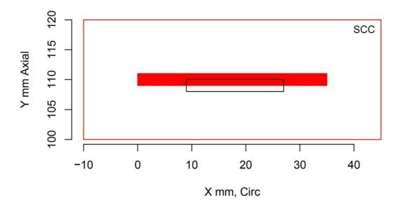
Figure H.95 Indication Plot for Procedure PAUT.114 Applied to Test Block P38 in PARENT Open Testing (X – Y view)
