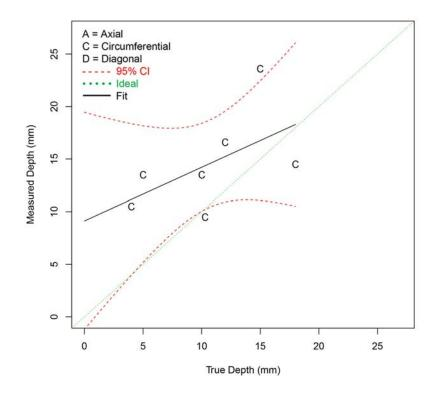
Figure F.57 Depth Sizing Regression (in mm) for Procedure PAATOFD.29.2 on FB Test Blocks in PARENT Open Testing (O.D. access)
