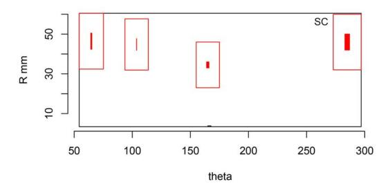
Figure H.15 Indication Plot for Procedure LUV.170 Applied to Test Block P7 in PARENT Open Testing (theta – R view)
