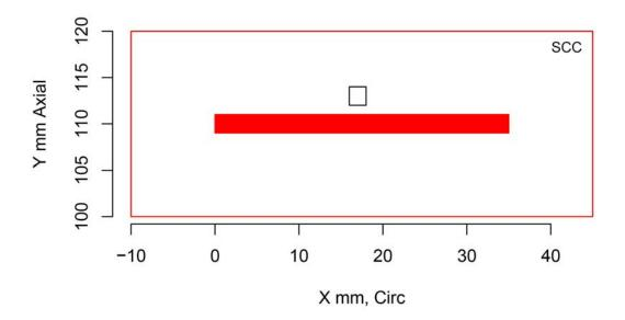
Figure H.309 Indication Plot for Procedure PAATOFD.29.2 Applied to Test Block P28 in PARENT Open Testing (X – Y view)
