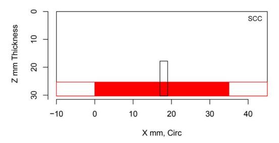
Figure H.348 Indication Plot for Procedure PAATOFD.29.1 Applied to Test Block P38 in PARENT Open Testing (X – Z view)
