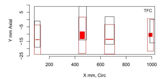
Figure H.97 Indication Plot for Procedure PAUT.114 Applied to Test Block P1 in PARENT Open Testing (X – Y view)
