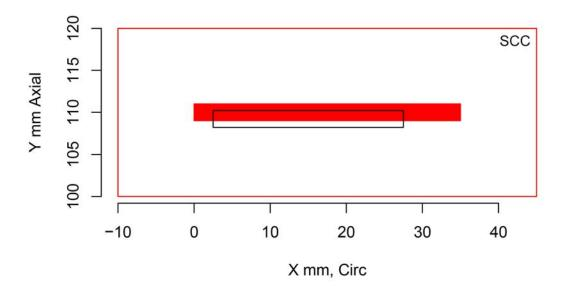
Figure H.165 Indication Plot for Procedure ECT.16 Applied to Test Block P31 in PARENT Open Testing (X – Y view)
