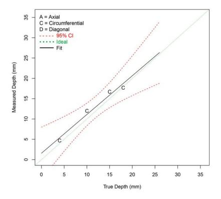
Figure F.20 Depth Sizing Regression (in mm) for Procedure SHPA.6.3 on SBDMW Test Blocks in PARENT Open Testing (O.D. access – w/ FB test blocks)
