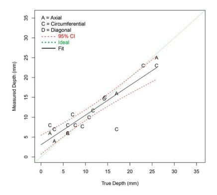
Figure F.40 Depth Sizing Regression (in mm) for Procedure PAUT.114 on SBDMW Test Blocks in PARENT Open Testing (O.D. access – w/o FB test blocks)
