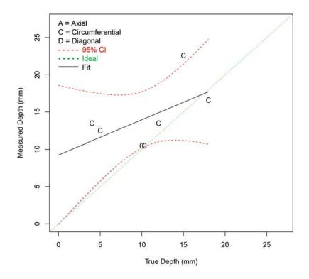
Figure F.56 Depth Sizing Regression (in mm) for Procedure PAATOFD.29.1 on FB Test Blocks in PARENT Open Testing (O.D. access)
