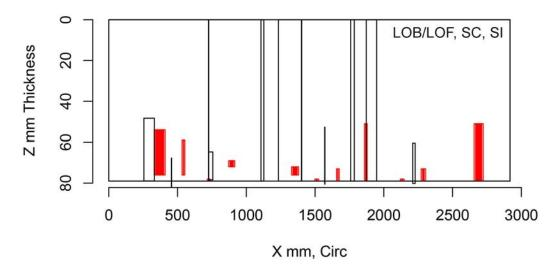
Figure H.156 Indication Plot for Procedure PAUT.150 Applied to Test Block P37 in PARENT Open Testing (X – Z view)
