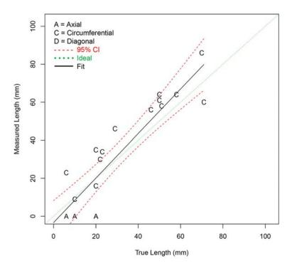
Figure G.2 Length Sizing Regression (in mm) for Procedure PAUT.114 on SBDMW Test Blocks in PARENT Open Testing (O.D. access)
