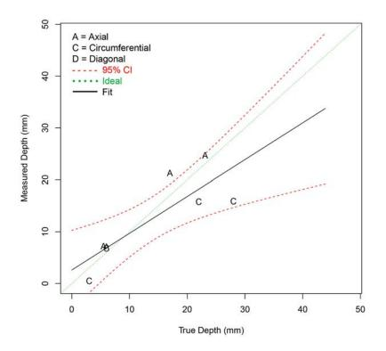
Figure F.94 Depth Sizing Regression (in mm) for PAUT Procedures on LBDMW Test Blocks in PARENT Open Testing (I.D. access)
