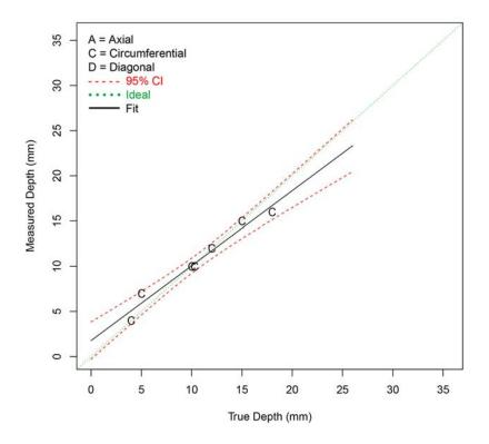
Figure F.10 Depth Sizing Regression (in mm) for Procedure PAUT.122.2 on SBDMW Test Blocks in PARENT Open Testing (O.D. access – w/ FB test blocks)
