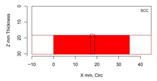
Figure H.306 Indication Plot for Procedure PATP.29 Applied to Test Block P28 in PARENT Open Testing (X – Z view)
