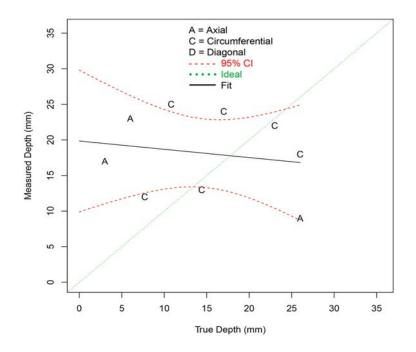
Figure F.36 Depth Sizing Regression (in mm) for Procedure HHUT.27.1 on SBDMW Test Blocks in PARENT Open Testing (O.D. access – w/o FB test blocks)
