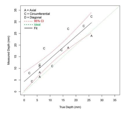
Figure F.45 Depth Sizing Regression (in mm) for Procedure SAFT.17 on SBDMW Test Blocks in PARENT Open Testing (O.D. access – w/o FB test blocks)
