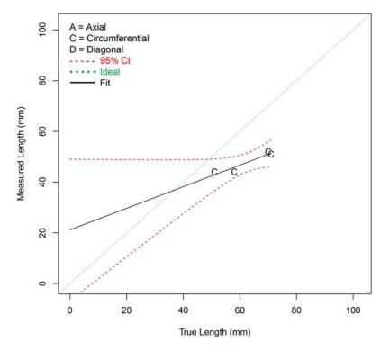
Figure G.8 Length Sizing Regression (in mm) for Procedure SHPA.6.2 on SBDMW Test Blocks in PARENT Open Testing (O.D. access)
