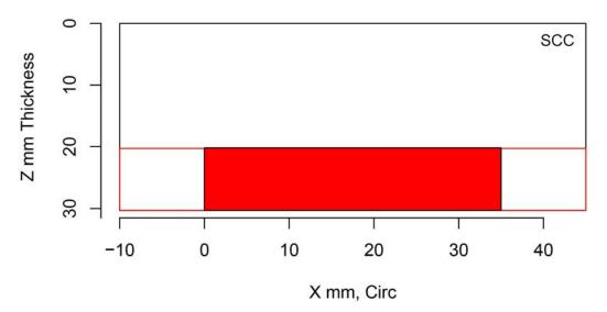
Figure H.80 Indication Plot for Procedure RT.112 Applied to Test Block P29 in PARENT Open Testing (X – Z view)
