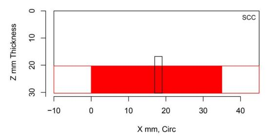
Figure H.318 Indication Plot for Procedure PAATOFD.29.2 Applied to Test Block P29 in PARENT Open Testing (X – Z view)
