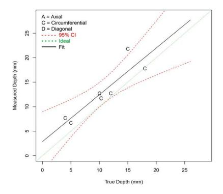
Figure F.30 Depth Sizing Regression (in mm) for Procedure PAATOFD.29.1 on SBDMW Test Blocks in PARENT Open Testing (I.D. access – w/ FB test blocks)
