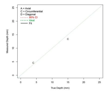
Figure F.79 Depth Sizing Regression (in mm) for Procedure PAUT.131.1 on FB Test Blocks in PARENT Open Testing (I.D. access)
