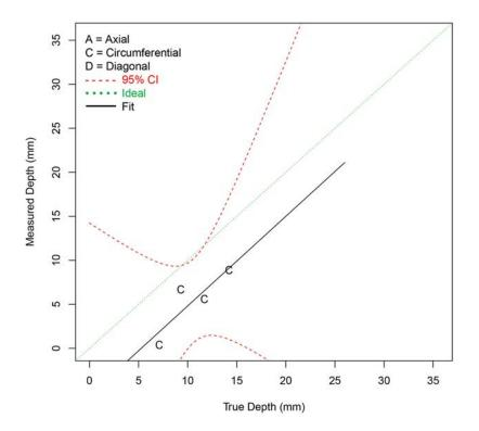
Figure F.19 Depth Sizing Regression (in mm) for Procedure SHPA.6.2 on SBDMW Test Blocks in PARENT Open Testing (O.D. access – w/ FB test blocks)
