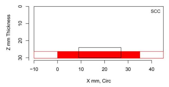
Figure H.118 Indication Plot for Procedure PAUT.122.1 Applied to Test Block P31 in PARENT Open Testing (X – Z view)
