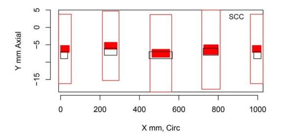
Figure H.143 Indication Plot for Procedure PAUT.131.1 Applied to Test Block P38 in PARENT Open Testing (X – Y view)
