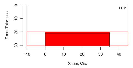
Figure H.206 Indication Plot for Procedure SAFT.17 Applied to Test Block P42 in PARENT Open Testing (X – Z view)
