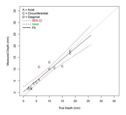
Figure F.26 Depth Sizing Regression (in mm) for RT Procedures SBDMW Test Blocks in PARENT Open Testing (O.D. access – w/ FB test blocks)
