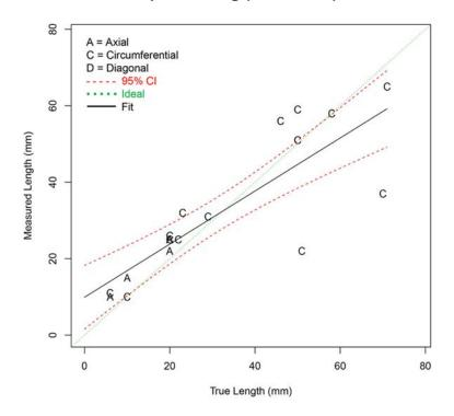
Figure G.15 Length Sizing Regression (in mm) for Procedure ECT.16 on SBDMW Test Blocks in PARENT Open Testing (I.D. access)
