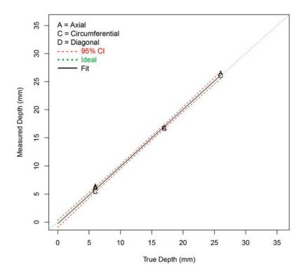
Figure F.42 Depth Sizing Regression (in mm) for Procedure 131.4 on SBDMW Test Blocks in PARENT Open Testing (O.D. access – w/o FB test blocks)
