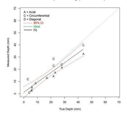
Figure F.85 Depth Sizing Regression (in mm) for Procedure PATP.29 on LBDMW Test Blocks in PARENT Open Testing (O.D. access)
