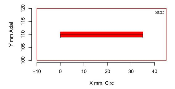
Figure H.247 Indication Plot for Procedure PAUT.20 Applied to Test Block P32 in PARENT Open Testing (X – Y view)
