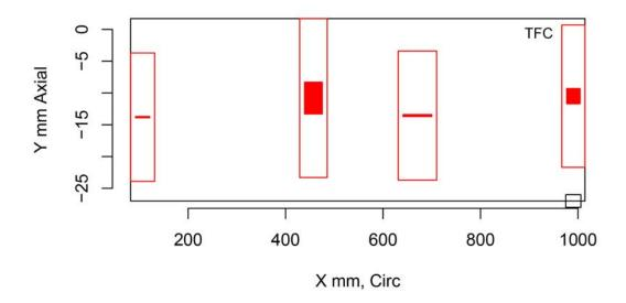
Figure H.215 Indication Plot for Procedure LUV.170 Applied to Test Block P1 in PARENT Open Testing (X – Y view)
