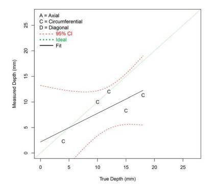
Figure F.55 Depth Sizing Regression (in mm) for Procedure LASH.18 on FB Test Blocks in PARENT Open Testing (O.D. access)
