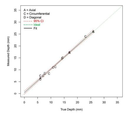
Figure F.12 Depth Sizing Regression (in mm) for Procedure PAUT.131.2 on SBDMW Test Blocks in PARENT Open Testing (O.D. access – w/ FB test blocks)
