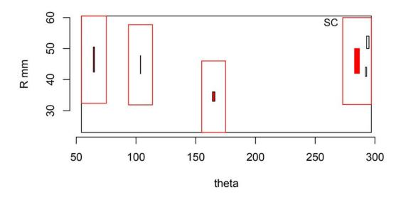
Figure H.23 Indication Plot for Procedure AECT.33 Applied to Test Block P7 in PARENT Open Testing (theta – R view)
