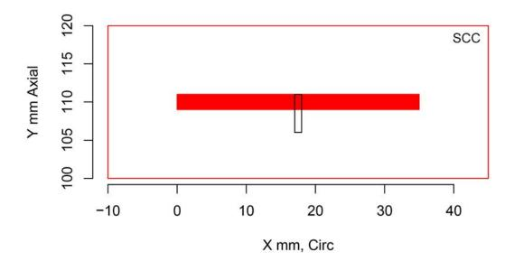
Figure H.107 Indication Plot for Procedure PAUT.122.2 Applied to Test Block P28 in PARENT Open Testing (X – Y view)
