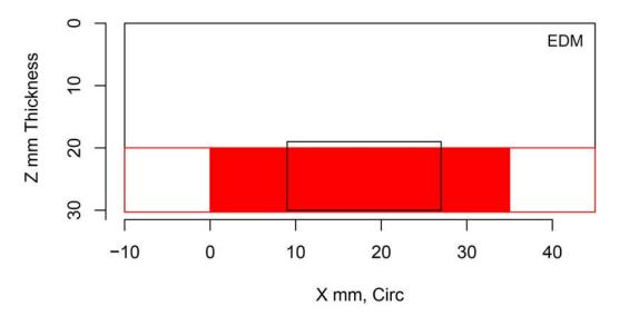
Figure H.104 Indication Plot for Procedure PAUT.114 Applied to Test Block P42 in PARENT Open Testing (X – Z view)
