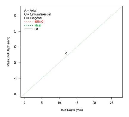
Figure F.64 Depth Sizing Regression (in mm) for Procedure RT.112 on FB Test Blocks in PARENT Open Testing (O.D. access)
