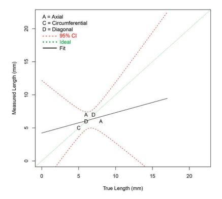
Figure G.32 Length Sizing Regression (in mm) for Procedure LUV.170 on BMI Test Blocks in PARENT Open Testing (J-groove weld access)
