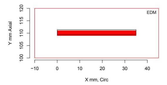
Figure H.179 Indication Plot for Procedure ECT.16 Applied to Test Block P42 in PARENT Open Testing (X – Y view)
