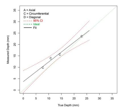
Figure F.46 Depth Sizing Regression (in mm) for Procedure SHPA.6.1 on SBDMW Test Blocks in PARENT Open Testing (O.D. access – w/o FB test blocks)
