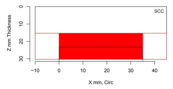
Figure H.190 Indication Plot for Procedure SAFT.17 Applied to Test Block P32 in PARENT Open Testing (X – Z view)
