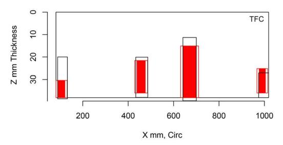
Figure H.196 Indication Plot for Procedure SAFT.17 Applied to Test Block P1 in PARENT Open Testing (X – Z view)
