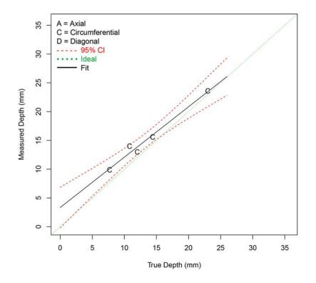
Figure F.18 Depth Sizing Regression (in mm) for Procedure SHPA.6.1 on SBDMW Test Blocks in PARENT Open Testing (O.D. access – w/ FB test blocks)
