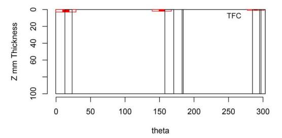
Figure H.2 Indication Plot for Procedure ECT.16 Applied to Test Block P5 in PARENT Open Testing (theta – Z view)
