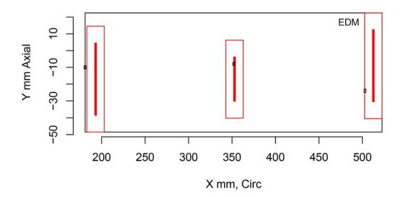
Figure H.373 Indication Plot for Procedure PAATOFD.29.0 Applied to Test Block P23 in PARENT Open Testing (X – Y view)
