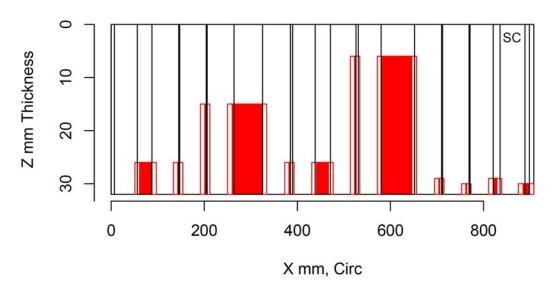
Figure H.422 Indication Plot for Procedure AECT.33 Applied to Test Block P41 in PARENT Open Testing (X – Z view)
