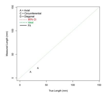
Figure G.22 Length Sizing Regression (in mm) for Procedure CEECT.5.2 on LBDMW Test Blocks in PARENT Open Testing (I.D. access)
