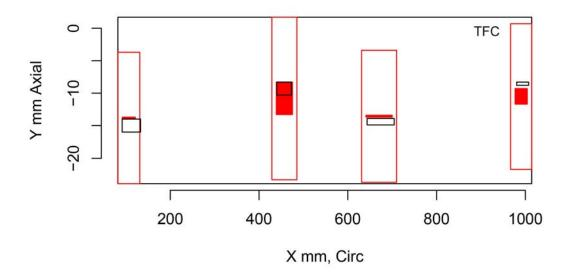
Figure H.445 Indication Plot for Procedure SHPA.6.1 Applied to Test Block P1 in PARENT Open Testing (X – Y view)
