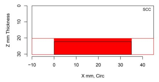
Figure H.236 Indication Plot for Procedure PAUT.20 Applied to Test Block P29 in PARENT Open Testing (X – Z view)
