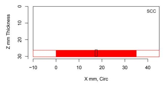
Figure H.120 Indication Plot for Procedure PAUT.122.2 Applied to Test Block P31 in PARENT Open Testing (X – Z view)
