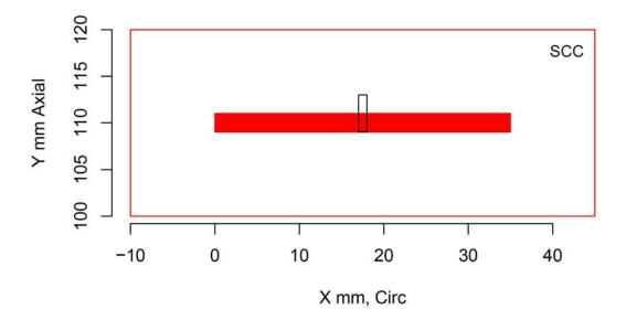
Figure H.127 Indication Plot for Procedure PAUT.122.2 Applied to Test Block P38 in PARENT Open Testing (X – Y view)
