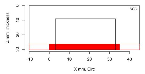
Figure H.268 Indication Plot for Procedure HHUT.27.1 Applied to Test Block P31 in PARENT Open Testing (X – Z view)
