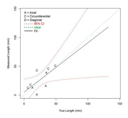
Figure G.25 Length Sizing Regression (in mm) for Procedure PAUT.7 on LBDMW Test Blocks in PARENT Open Testing (I.D. access)
