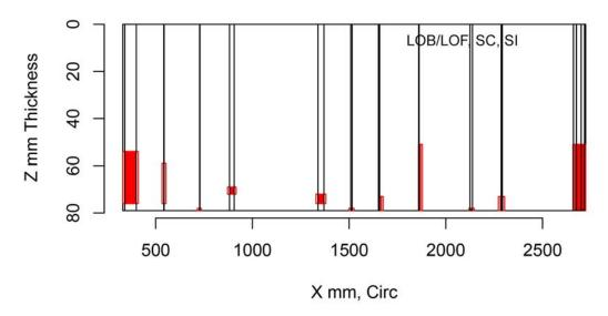
Figure H.420 Indication Plot for Procedure AECT.33 Applied to Test Block P37 in PARENT Open Testing (X – Z view)
