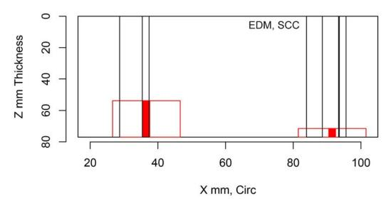
Figure H.178 Indication Plot for Procedure ECT.16 Applied to Test Block P12 in PARENT Open Testing (X – Z view)
