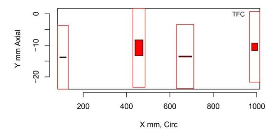
Figure H.227 Indication Plot for Procedure LASH.18 Applied to Test Block P1 in PARENT Open Testing (X – Y view)
