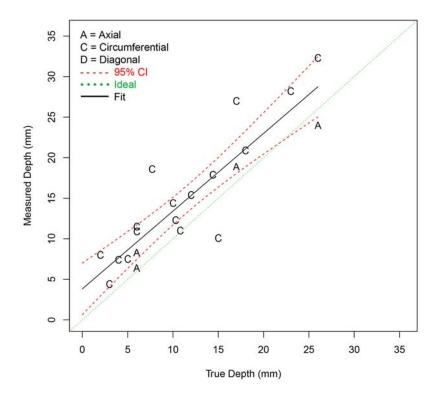
Figure F.17 Depth Sizing Regression (in mm) for Procedure SAFT.17 on SBDMW Test Blocks in PARENT Open Testing (O.D. access – w/ FB test blocks)
