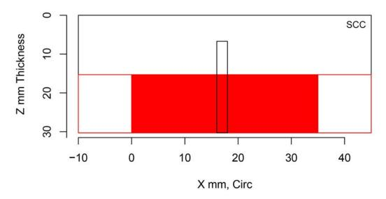
Figure H.342 Indication Plot for Procedure PAATOFD.29.2 Applied to Test Block P32 in PARENT Open Testing (X – Z view)
