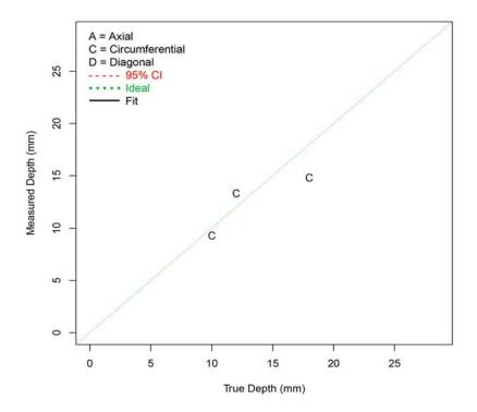
Figure F.29 Depth Sizing Regression (in mm) for Procedure HHUT.30 on SBDMW Test Blocks in PARENT Open Testing (I.D. access – w/ FB test blocks)
