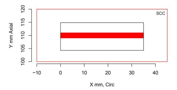
Figure H.237 Indication Plot for Procedure UIR.20 Applied to Test Block P29 in PARENT Open Testing (X – Y view)
