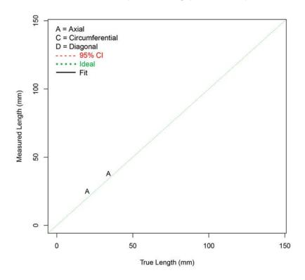
Figure G.23 Length Sizing Regression (in mm) for Procedure ECT.16 on LBDMW Test Blocks in PARENT Open Testing (I.D. access)
