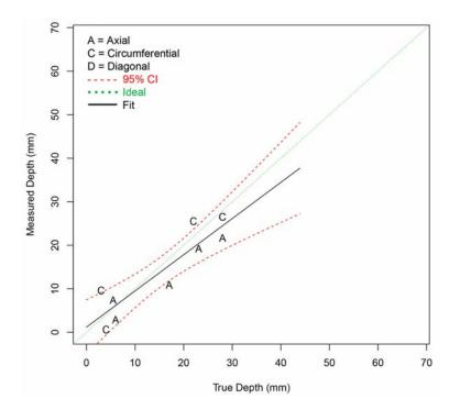
Figure F.84 Depth Sizing Regression (in mm) for Procedure PAATOFD.29.0 on LBDMW Test Blocks in PARENT Open Testing (O.D. access)
