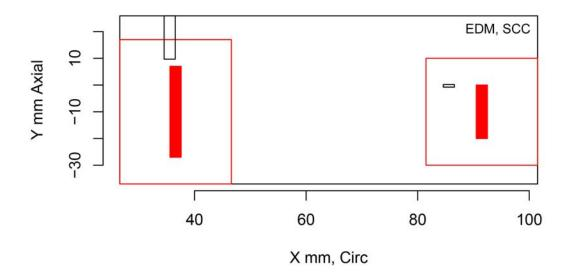
Figure H.451 Indication Plot for Procedure ECT.7 Applied to Test Block P12 in PARENT Open Testing (X – Y view)
