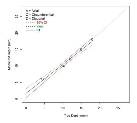
Figure F.59 Depth Sizing Regression (in mm) for Procedure PAUT.122.1 on FB Test Blocks in PARENT Open Testing (O.D. access)
