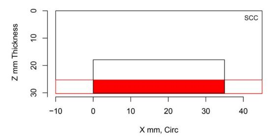
Figure H.254 Indication Plot for Procedure UIR.20 Applied to Test Block P38 in PARENT Open Testing (X – Z view)
