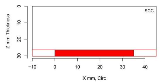
Figure H.58 Indication Plot for Procedure RT.109 Applied to Test Block P31 in PARENT Open Testing (X – Z view)
