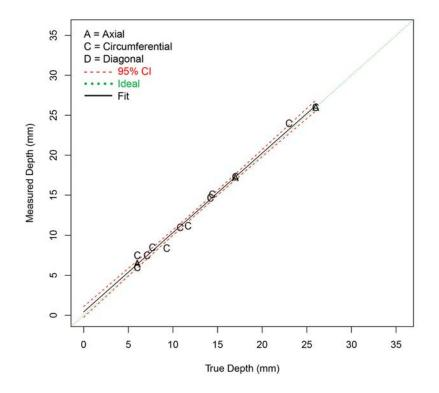
Figure F.41 Depth Sizing Regression (in mm) for Procedure PAUT.131.2 on SBDMW Test Blocks in PARENT Open Testing (O.D. access – w/o FB test blocks)
