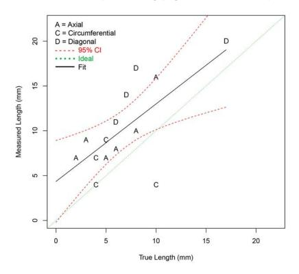
Figure G.31 Length Sizing Regression (in mm) for Procedure ECT.7 on BMI Test Blocks in PARENT Open Testing (J-groove weld access)
