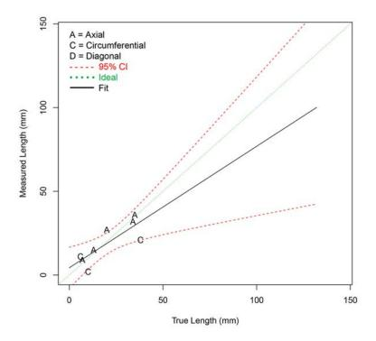
Figure G.21 Length Sizing Regression (in mm) for Procedure AECT.33 on LBDMW Test Blocks in PARENT Open Testing (I.D. access)
