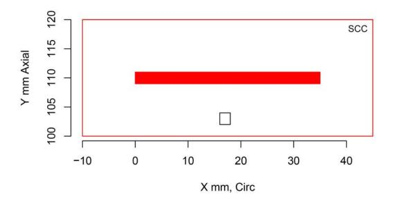
Figure H.343 Indication Plot for Procedure PAATOFD.29.0 Applied to Test Block P38 in PARENT Open Testing (X – Y view)
