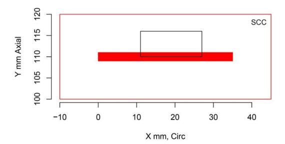
Figure H.93 Indication Plot for Procedure PAUT.114 Applied to Test Block P32 in PARENT Open Testing (X – Y view)
