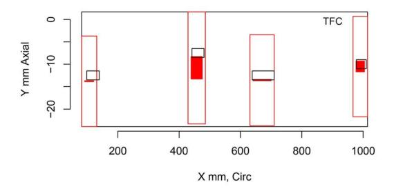
Figure H.171 Indication Plot for Procedure ECT.16 Applied to Test Block P1 in PARENT Open Testing (X – Y view)
