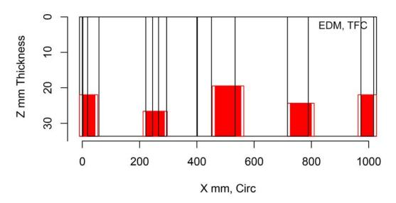
Figure H.174 Indication Plot for Procedure ECT.16 Applied to Test Block P4 in PARENT Open Testing (X – Z view)
