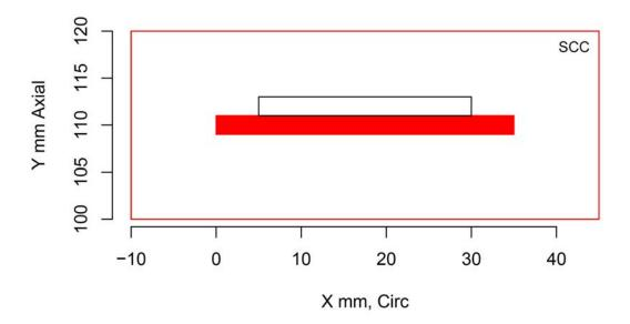
Figure H.415 Indication Plot for Procedure AECT.33 Applied to Test Block P32 in PARENT Open Testing (X – Y view)
