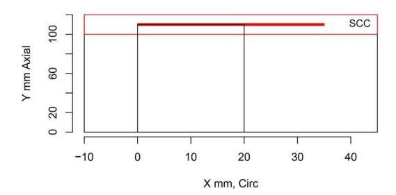
Figure H.71 Indication Plot for Procedure PECT.11 Applied to Test Block P29 in PARENT Open Testing (X – Y view)
