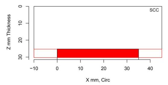
Figure H.192 Indication Plot for Procedure SAFT.17 Applied to Test Block P38 in PARENT Open Testing (X – Z view)
