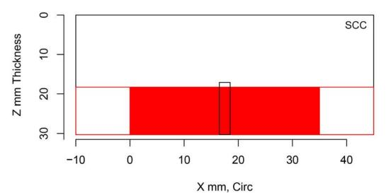
Figure H.134 Indication Plot for Procedure PAUT.131.1 Applied to Test Block P28 in PARENT Open Testing (X – Z view)
