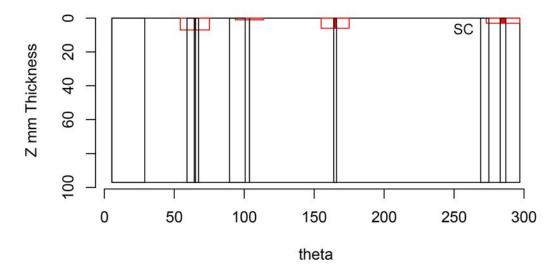
Figure H.4 Indication Plot for Procedure ECT.16 Applied to Test Block P7 in PARENT Open Testing (theta – Z view)
