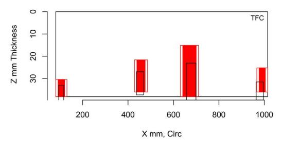
Figure H.256 Indication Plot for Procedure PAUT.20 Applied to Test Block P1 in PARENT Open Testing (X – Z view)
