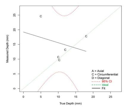
Figure F.69 Depth Sizing Regression (in mm) for Procedure UT.104 on FB Test Blocks in PARENT Open Testing (O.D. access)
