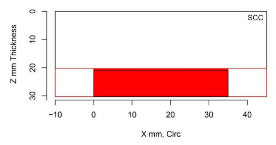
Figure H.38 Indication Plot for Procedure UT.104 Applied to Test Block P29 in PARENT Open Testing (X – Z view)
