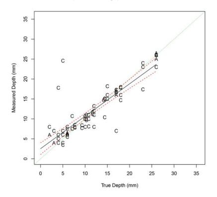
Figure F.25 Depth Sizing Regression (in mm) for PAUT Procedures SBDMW Test Blocks in PARENT Open Testing (O.D. access – w/ FB test blocks)
