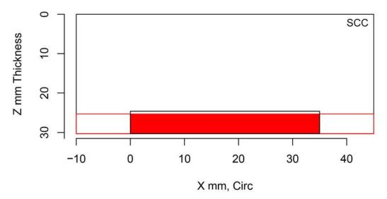
Figure H.46 Indication Plot for Procedure UT.104 Applied to Test Block P38 in PARENT Open Testing (X – Z view)
