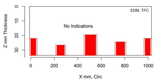
Figure H.258 Indication Plot for Procedure PAUT.20 Applied to Test Block P1 in PARENT Open Testing (X – Z view)
