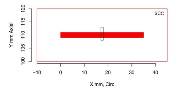
Figure H.123 Indication Plot for Procedure PAUT.122.2 Applied to Test Block P32 in PARENT Open Testing (X – Y view)
