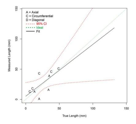
Figure G.28 Length Sizing Regression (in mm) for PAUT Procedures on LBDMW Test Blocks in PARENT Open Testing (I.D. access)
