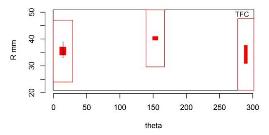
Figure H.5 Indication Plot for Procedure LUV.170 Applied to Test Block P5 in PARENT Open Testing (theta – R view)
