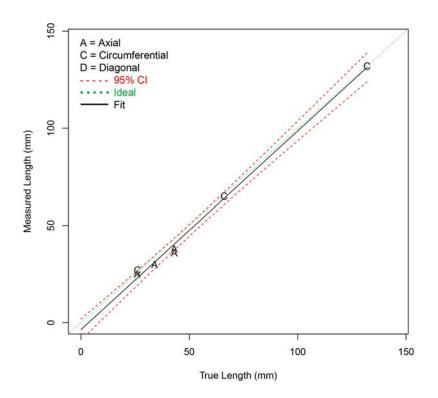
Figure G.24 Length Sizing Regression (in mm) for Procedure MM.28.1 on LBDMW Test Blocks in PARENT Open Testing (I.D. access)
