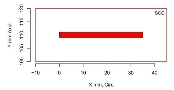
Figure H.159 Indication Plot for Procedure ECT.16 Applied to Test Block P28 in PARENT Open Testing (X – Y view)
