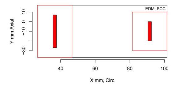
Figure H.229 Indication Plot for Procedure LASH.18 Applied to Test Block P12 in PARENT Open Testing (X – Y view)
