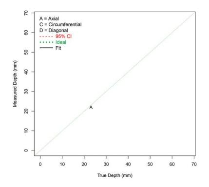
Figure F.89 Depth Sizing Regression (in mm) for NLUT Procedures on LBDMW Test Blocks in PARENT Open Testing (O.D. access)
