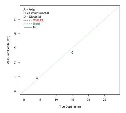
Figure F.32 Depth Sizing Regression (in mm) for Procedure PAUT.131.1 on SBDMW Test Blocks in PARENT Open Testing (I.D. access – w/ FB test blocks)
