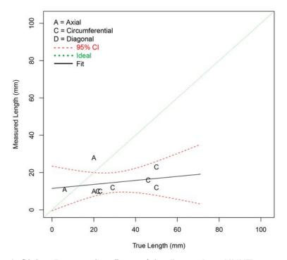
Figure G.1 Length Sizing Regression (in mm) for Procedure HHUT.27.1 on SBDMW Test Blocks in PARENT Open Testing (O.D. access)
