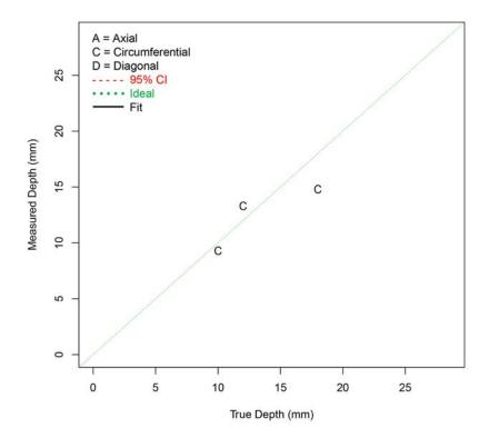
Figure F.34 Depth Sizing Regression (in mm) for NLUT Procedures on SBDMW Test Blocks in PARENT Open Testing (I.D. access – w/ FB test blocks)
