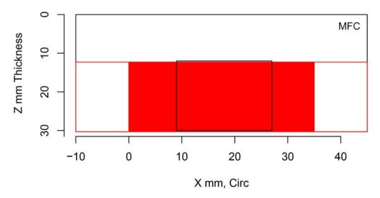
Figure H.90 Indication Plot for Procedure PAUT.114 Applied to Test Block P30 in PARENT Open Testing (X – Z view)
