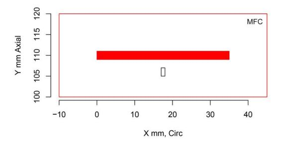
Figure H.115 Indication Plot for Procedure PAUT.122.2 Applied to Test Block P30 in PARENT Open Testing (X – Y view)
