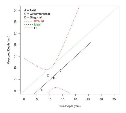
Figure F.47 Depth Sizing Regression (in mm) for Procedure SHPA.6.2 on SBDMW Test Blocks in PARENT Open Testing (O.D. access – w/o FB test blocks)
