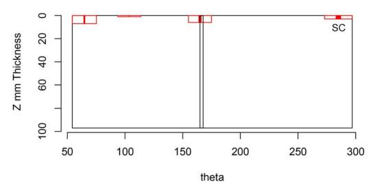
Figure H.16 Indication Plot for Procedure LUV.170 Applied to Test Block P7 in PARENT Open Testing (theta – Z view)
