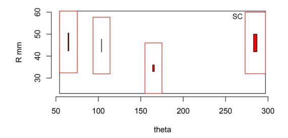
Figure H.25 Indication Plot for Procedure CEECT.5.1 Applied to Test Block P7 in PARENT Open Testing (theta – R view)
