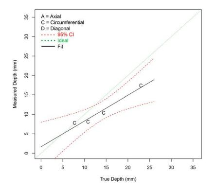
Figure F.43 Depth Sizing Regression (in mm) for Procedure PAUT.20 on SBDMW Test Blocks in PARENT Open Testing (O.D. access – w/o FB test blocks)
