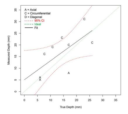
Figure F.39 Depth Sizing Regression (in mm) for Procedure PATP.29 on SBDMW Test Blocks in PARENT Open Testing (O.D. access – w/o FB test blocks)
