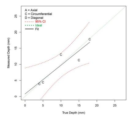
Figure F.62 Depth Sizing Regression (in mm) for Procedure PAUT.20 on FB Test Blocks in PARENT Open Testing (O.D. access)
