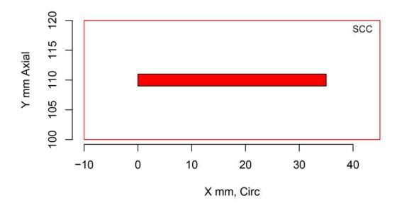
Figure H.251 Indication Plot for Procedure PAUT.20 Applied to Test Block P38 in PARENT Open Testing (X – Y view)
