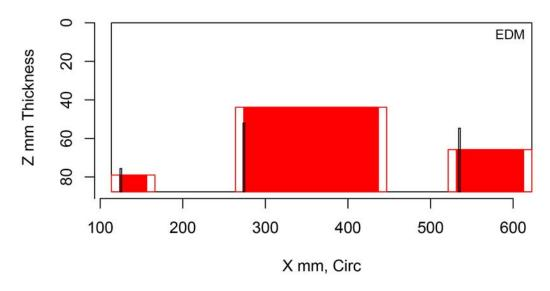
Figure H.384 Indication Plot for Procedure PAATOFD.29.1 Applied to Test Block P24 in PARENT Open Testing (X – Z view)
