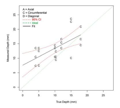
Figure F.70 Depth Sizing Regression (in mm) for ADVPAUT Procedures on FB Test Blocks in PARENT Open Testing (O.D. access)
