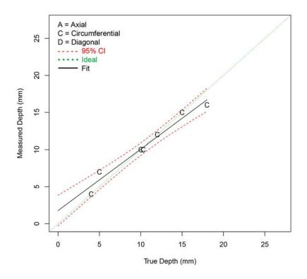
Figure F.60 Depth Sizing Regression (in mm) for Procedure PAUT.122.2 on FB Test Blocks in PARENT Open Testing (O.D. access)
