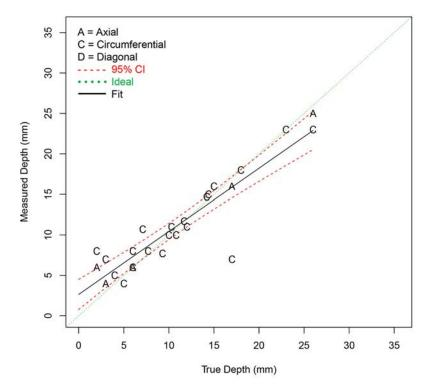
Figure F.8 Depth Sizing Regression (in mm) for Procedure PAUT.114 on SBDMW Test Blocks in PARENT Open Testing (O.D. access – w/ FB test blocks)
