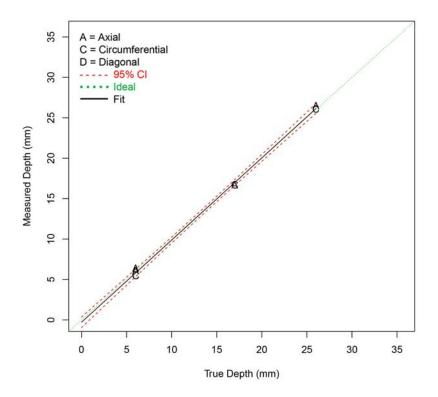
Figure F.13 Depth Sizing Regression (in mm) for Procedure PAUT.131.4 on SBDMW Test Blocks in PARENT Open Testing (O.D. access – w/ FB test blocks)
