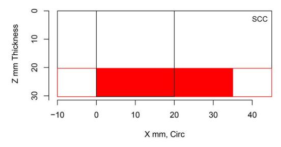
Figure H.72 Indication Plot for Procedure PECT.11 Applied to Test Block P29 in PARENT Open Testing (X – Z view)
