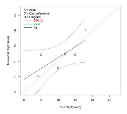
Figure F.66 Depth Sizing Regression (in mm) for Procedure SHPA.6.1 on FB Test Blocks in PARENT Open Testing (O.D. access)
