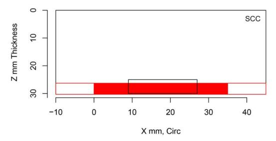
Figure H.92 Indication Plot for Procedure PAUT.114 Applied to Test Block P31 in PARENT Open Testing (X – Z view)
