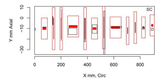
Figure H.197 Indication Plot for Procedure SAFT.17 Applied to Test Block P41 in PARENT Open Testing (X – Y view)
