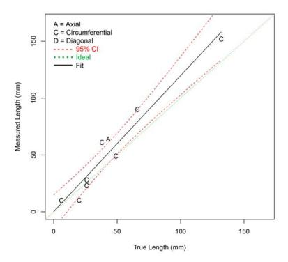
Figure G.19 Length Sizing Regression (in mm) for ADVPAUT Procedures on LBDMW Test Blocks in PARENT Open Testing (O.D. access)
