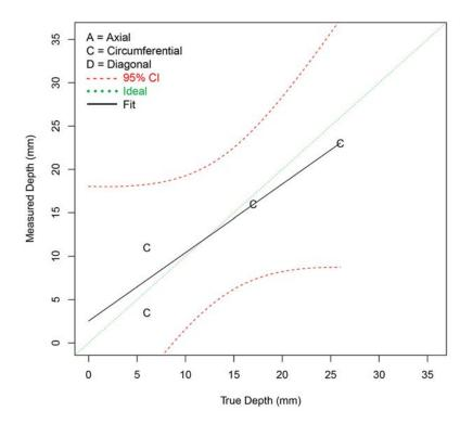
Figure F.52 Depth Sizing Regression (in mm) for RT Procedures on SBDMW Test Blocks in PARENT Open Testing (O.D. access – w/o FB test blocks)
