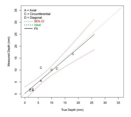
Figure F.16 Depth Sizing Regression (in mm) for Procedure RT.112 on SBDMW Test Blocks in PARENT Open Testing (O.D. access – w/ FB test blocks)
