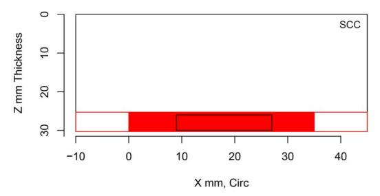
Figure H.96 Indication Plot for Procedure PAUT.114 Applied to Test Block P38 in PARENT Open Testing (X – Z view)
