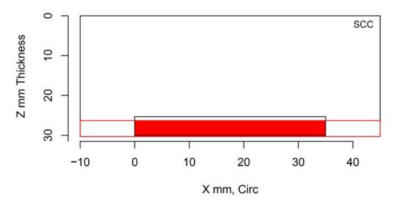
Figure H.442 Indication Plot for Procedure SHPA.6.1 Applied to Test Block P31 in PARENT Open Testing (X – Z view)
