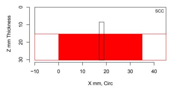
Figure H.336 Indication Plot for Procedure PAATOFD.29.0 Applied to Test Block P32 in PARENT Open Testing (X – Z view)
