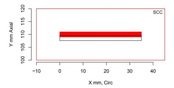
Figure H.43 Indication Plot for Procedure UT.104 Applied to Test Block P32 in PARENT Open Testing (X – Y view)
