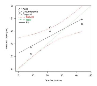
Figure F.93 Depth Sizing Regression (in mm) for ADVPAUT Procedures on LBDMW Test Blocks in PARENT Open Testing (I.D. access)
