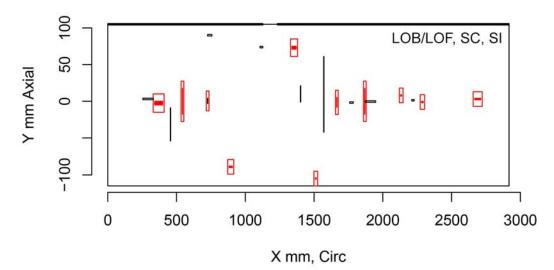
Figure H.155 Indication Plot for Procedure PAUT.150 Applied to Test Block P37 in PARENT Open Testing (X – Y view)
