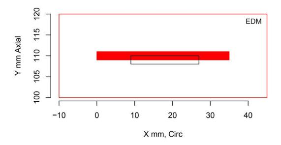
Figure H.103 Indication Plot for Procedure PAUT.114 Applied to Test Block P42 in PARENT Open Testing (X – Y view)
