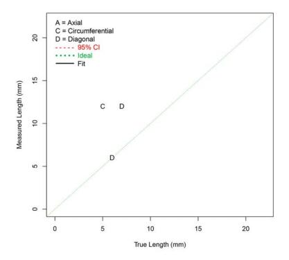
Figure G.30 Length Sizing Regression (in mm) for Procedure ECT.16 on BMI Test Blocks in PARENT Open Testing (J-groove weld access)
