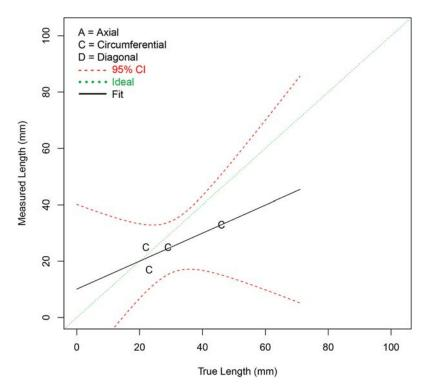
Figure G.5 Length Sizing Regression (in mm) for Procedure PAUT.20 on SBDMW Test Blocks in PARENT Open Testing (O.D. access)
