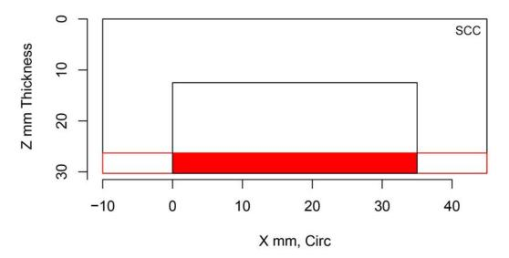
Figure H.244 Indication Plot for Procedure PAUT.20 Applied to Test Block P31 in PARENT Open Testing (X – Z view)
