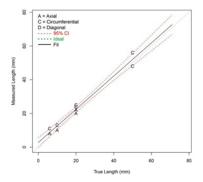
Figure G.14 Length Sizing Regression (in mm) for Procedure AECT.33 on SBDMW Test Blocks in PARENT Open Testing (I.D. access)
