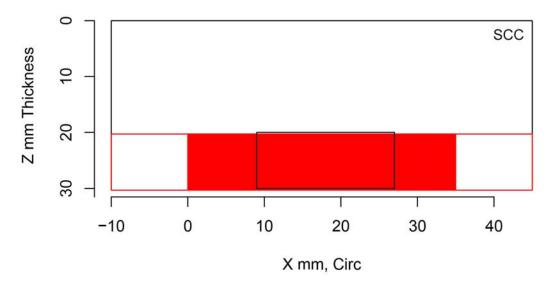
Figure H.88 Indication Plot for Procedure PAUT.114 Applied to Test Block P29 in PARENT Open Testing (X – Z view)
