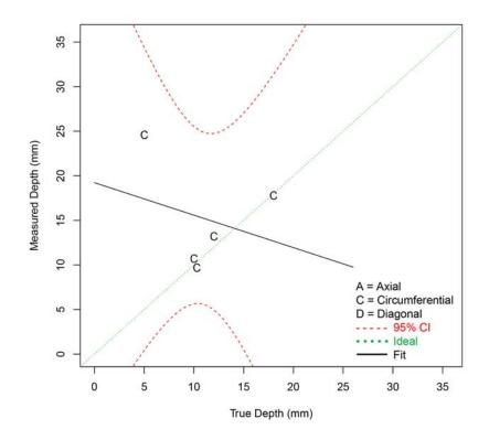
Figure F.11 Depth Sizing Regression (in mm) for Procedure PAUT.131.1 on SBDMW Test Blocks in PARENT Open Testing (O.D. access – w/ FB test blocks)
