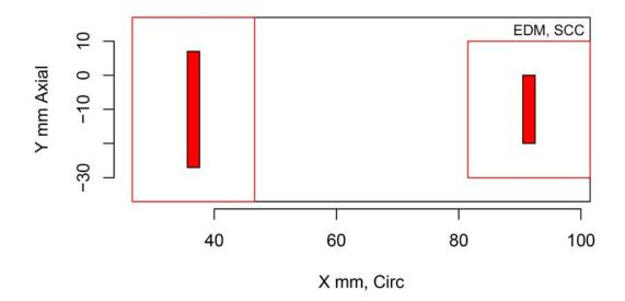
Figure H.369 Indication Plot for Procedure PAATOFD.29.1 Applied to Test Block P12 in PARENT Open Testing (X – Y view)
