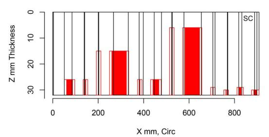
Figure H.176 Indication Plot for Procedure ECT.16 Applied to Test Block P41 in PARENT Open Testing (X – Z view)
