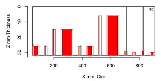
Figure H.152 Indication Plot for Procedure PAUT.131.2 Applied to Test Block P41 in PARENT Open Testing (X – Z view)
