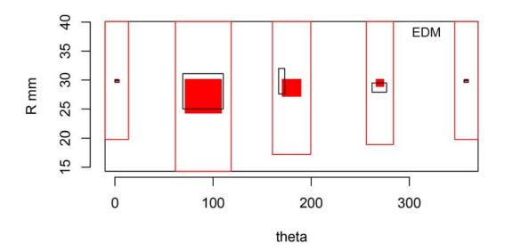
Figure H.31 Indication Plot for Procedure ECT.7 Applied to Test Block P22 in PARENT Open Testing (theta – R view)
