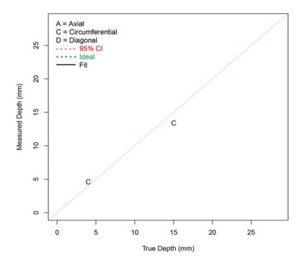
Figure F.35 Depth Sizing Regression (in mm) for PAUT Procedures on SBDMW Test Blocks in PARENT Open Testing (I.D. access – w/ FB test blocks)
