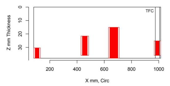
Figure H.216 Indication Plot for Procedure LUV.170 Applied to Test Block P1 in PARENT Open Testing (X – Z view)
