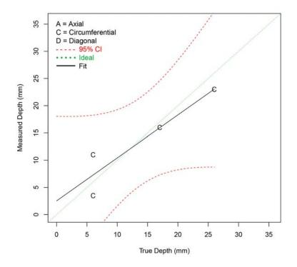
Figure F.48 Depth Sizing Regression (in mm) for Procedure UT.104 on SBDMW Test Blocks in PARENT Open Testing (O.D. access – w/o FB test blocks)
