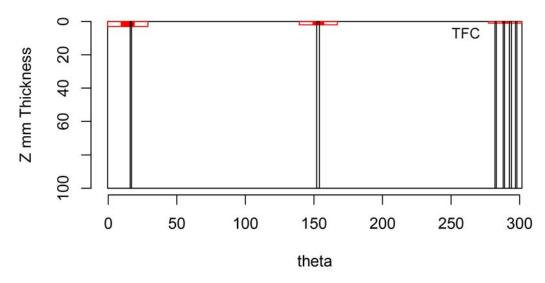
Figure H.22 Indication Plot for Procedure AECT.33 Applied to Test Block P5 in PARENT Open Testing (theta – Z view)
