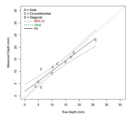
Figure F.28 Depth Sizing Regression (in mm) for UT Procedures SBDMW Test Blocks in PARENT Open Testing (O.D. access – w/ FB test blocks)
