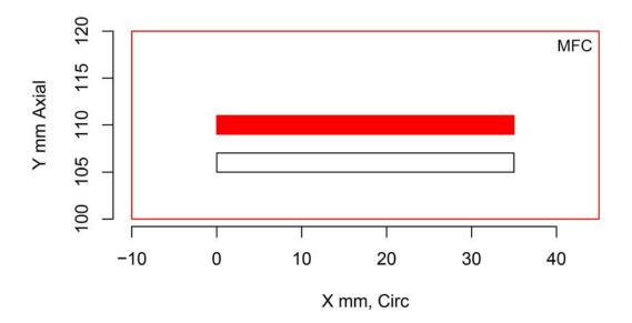
Figure H.39 Indication Plot for Procedure UT.104 Applied to Test Block P30 in PARENT Open Testing (X – Y view)
