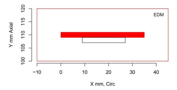
Figure H.129 Indication Plot for Procedure PAUT.122.1 Applied to Test Block P42 in PARENT Open Testing (X – Y view)
