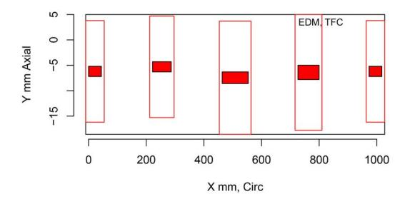
Figure H.431 Indication Plot for Procedure CEECT.5.1 Applied to Test Block P4 in PARENT Open Testing (X – Y view)
