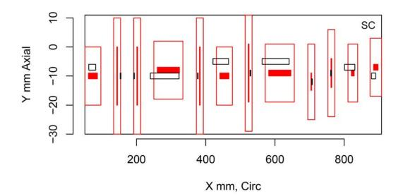
Figure H.101 Indication Plot for Procedure PAUT.114 Applied to Test Block P41 in PARENT Open Testing (X – Y view)
