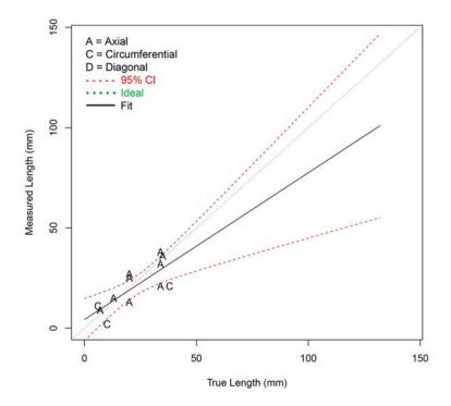
Figure G.26 Length Sizing Regression (in mm) for ECT Procedures on LBDMW Test Blocks in PARENT Open Testing (I.D. access)
