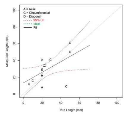
Figure G.6 Length Sizing Regression (in mm) for Procedure SAFT.17 on SBDMW Test Blocks in PARENT Open Testing (O.D. access)
