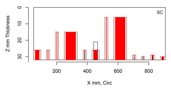
Figure H.84 Indication Plot for Procedure RT.112 Applied to Test Block P41 in PARENT Open Testing (X – Z view)
