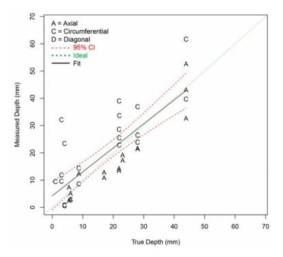
Figure F.88 Depth Sizing Regression (in mm) for ADVPAUT Procedures on LBDMW Test Blocks in PARENT Open Testing (O.D. access)
