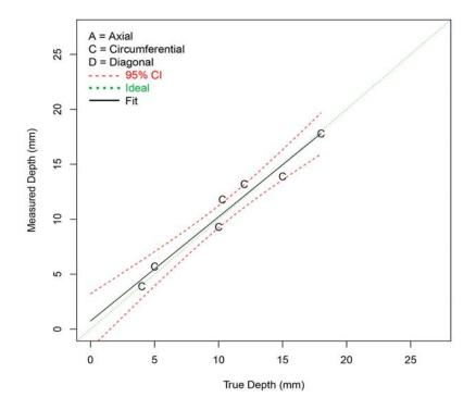
Figure F.75 Depth Sizing Regression (in mm) for UT Procedures on FB Test Blocks in PARENT Open Testing (O.D. access)
