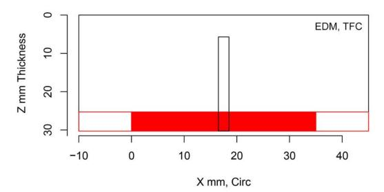
Figure H.148 Indication Plot for Procedure PAUT.131.1 Applied to Test Block P4 in PARENT Open Testing (X – Z view)
