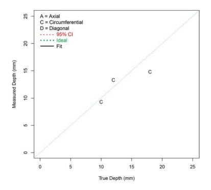
Figure F.76 Depth Sizing Regression (in mm) for Procedure HHUT.30 on FB Test Blocks in PARENT Open Testing (I.D. access)
