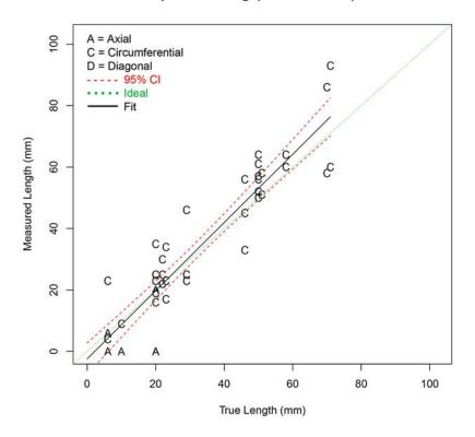
Figure G.12 Length Sizing Regression (in mm) for PAUT Procedures on SBDMW Test Blocks in PARENT Open Testing (O.D. access)
