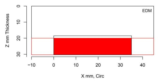
Figure H.50 Indication Plot for Procedure UT.104 Applied to Test Block P42 in PARENT Open Testing (X – Z view)
