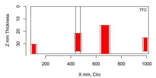
Figure H.212 Indication Plot for Procedure LUV.170 Applied to Test Block P1 in PARENT Open Testing (X – Z view)
