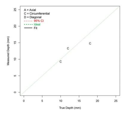
Figure F.81 Depth Sizing Regression (in mm) for NLUT Procedures on FB Test Blocks in PARENT Open Testing (I.D. access)
