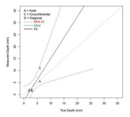
Figure F.44 Depth Sizing Regression (in mm) for Procedure RT.112 on SBDMW Test Blocks in PARENT Open Testing (O.D. access – w/o FB test blocks)
