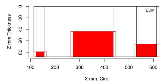
Figure H.302 Indication Plot for Procedure MM.28.1 Applied to Test Block P24 in PARENT Open Testing (X – Z view)
