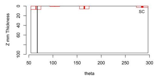
Figure H.12 Indication Plot for Procedure LUV.170 Applied to Test Block P7 in PARENT Open Testing (theta – Z view)
