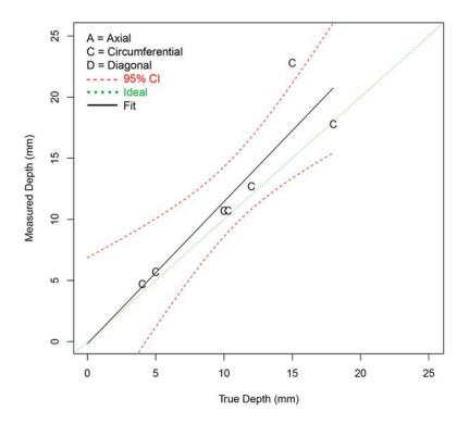
Figure F.78 Depth Sizing Regression (in mm) for Procedure PAATOFD.29.2 on FB Test Blocks in PARENT Open Testing (I.D. access)
