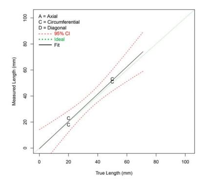
Figure G.13 Length Sizing Regression (in mm) for UT Procedures on SBDMW Test Blocks in PARENT Open Testing (O.D. access)
