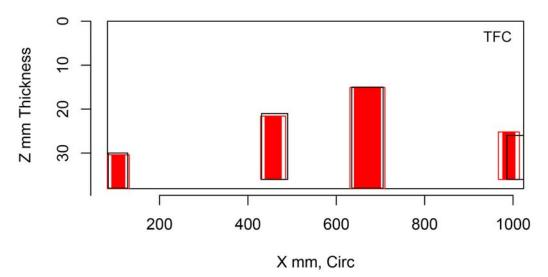
Figure H.98 Indication Plot for Procedure PAUT.114 Applied to Test Block P1 in PARENT Open Testing (X – Z view)
