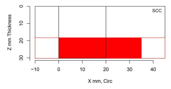
Figure H.68 Indication Plot for Procedure PECT.11 Applied to Test Block P28 in PARENT Open Testing (X – Z view)
