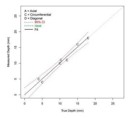
Figure F.58 Depth Sizing Regression (in mm) for Procedure PAUT.114 on FB Test Blocks in PARENT Open Testing (O.D. access)
