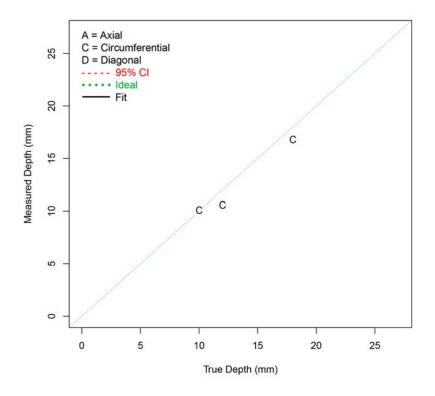
Figure F.63 Depth Sizing Regression (in mm) for Procedure RT.109 on FB Test Blocks in PARENT Open Testing (O.D. access)
