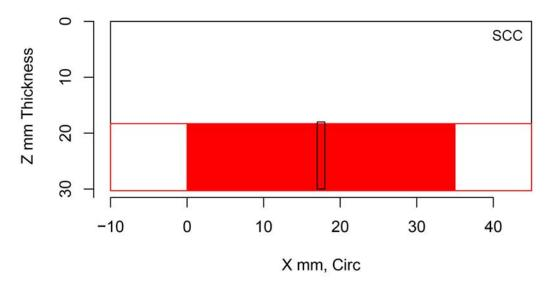
Figure H.108 Indication Plot for Procedure PAUT.122.2 Applied to Test Block P28 in PARENT Open Testing (X – Z view)
