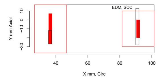
Figure H.157 Indication Plot for Procedure PAUT.150 Applied to Test Block P12 in PARENT Open Testing (X – Y view)
