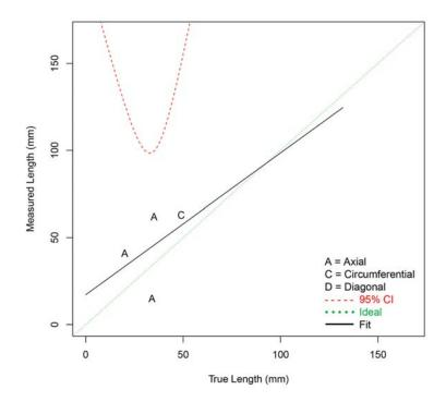
Figure G.17 Length Sizing Regression (in mm) for Procedure PAUT.150 on LBDMW Test Blocks in PARENT Open Testing (O.D. access)
