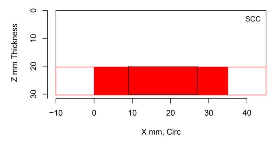
Figure H.110 Indication Plot for Procedure PAUT.122.1 Applied to Test Block P29 in PARENT Open Testing (X – Z view)
