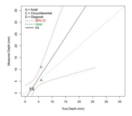
Figure F.53 Depth Sizing Regression (in mm) for UT Procedures on SBDMW Test Blocks in PARENT Open Testing (O.D. access – w/o FB test blocks)
