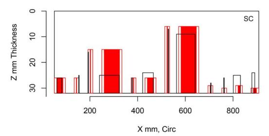
Figure H.102 Indication Plot for Procedure PAUT.114 Applied to Test Block P41 in PARENT Open Testing (X – Z view)
