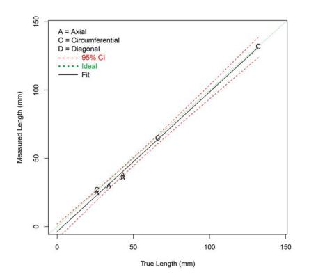
Figure G.27 Length Sizing Regression (in mm) for MM Procedures on LBDMW Test Blocks in PARENT Open Testing (I.D. access)
