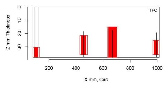
Figure H.358 Indication Plot for Procedure PAATOFD.29.0 Applied to Test Block P1 in PARENT Open Testing (X – Z view)
