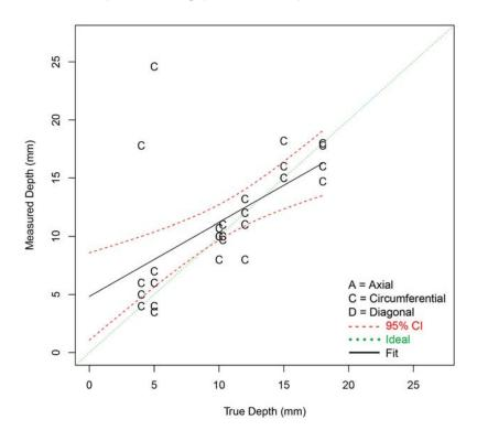
Figure F.72 Depth Sizing Regression (in mm) for PAUT Procedures on FB Test Blocks in PARENT Open Testing (O.D. access)
