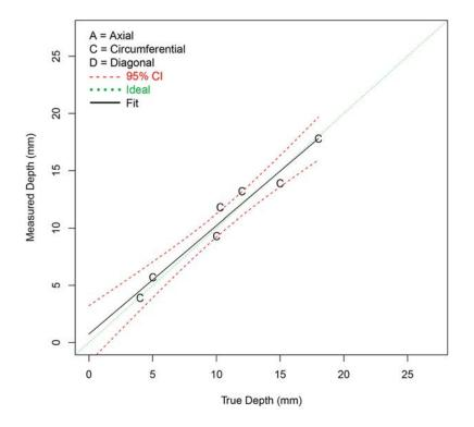
Figure F.67 Depth Sizing Regression (in mm) for Procedure SHPA.6.3 on FB Test Blocks in PARENT Open Testing (O.D. access)
