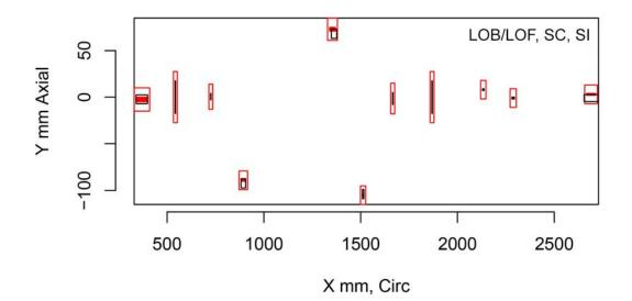
Figure H.193 Indication Plot for Procedure SAFT.17 Applied to Test Block P37 in PARENT Open Testing (X – Y view)
