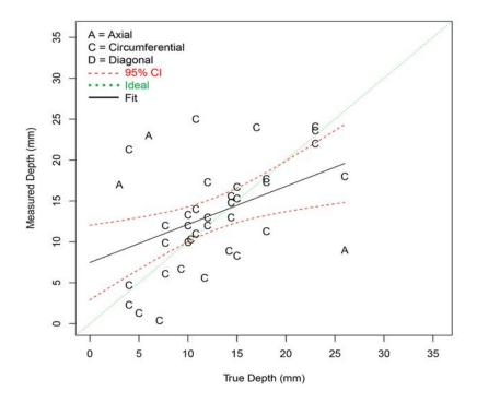
Figure F.24 Depth Sizing Regression (in mm) for NLUT Procedures SBDMW Test Blocks in PARENT Open Testing (O.D. access – w/ FB test blocks)
