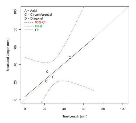
Figure G.7 Length Sizing Regression (in mm) for Procedure SHPA.6.1 on SBDMW Test Blocks in PARENT Open Testing (O.D. access)
