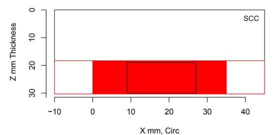
Figure H.86 Indication Plot for Procedure PAUT.114 Applied to Test Block P28 in PARENT Open Testing (X – Z view)
