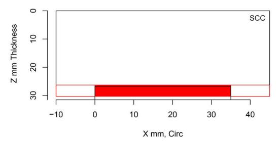
Figure H.188 Indication Plot for Procedure SAFT.17 Applied to Test Block P31 in PARENT Open Testing (X – Z view)
