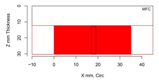
Figure H.320 Indication Plot for Procedure PAATOFD.29.0 Applied to Test Block P30 in PARENT Open Testing (X – Z view)
