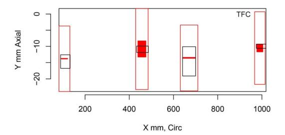
Figure H.195 Indication Plot for Procedure SAFT.17 Applied to Test Block P1 in PARENT Open Testing (X – Y view)
