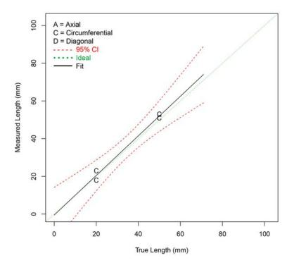
Figure G.9 Length Sizing Regression (in mm) for Procedure UT.104 on SBDMW Test Blocks in PARENT Open Testing (O.D. access)
