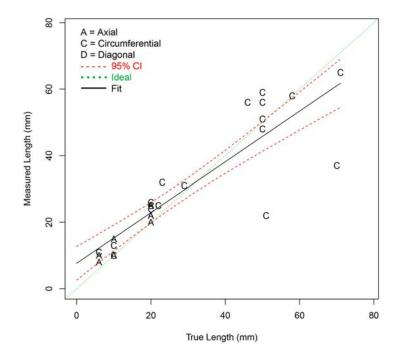
Figure G.16 Length Sizing Regression (in mm) for ECT Procedures on SBDMW Test Blocks in PARENT Open Testing (I.D. access)
