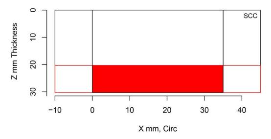
Figure H.284 Indication Plot for Procedure MM.28.1 Applied to Test Block P29 in PARENT Open Testing (X – Z view)
