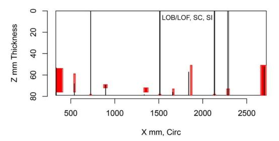
Figure H.352 Indication Plot for Procedure PAATOFD.29.0 Applied to Test Block P37 in PARENT Open Testing (X – Z view)
