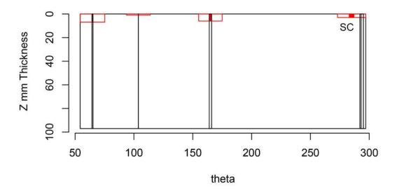
Figure H.33 Indication Plot for Procedure ECT.7 Applied to Test Block P7 in PARENT Open Testing (theta – R view)
