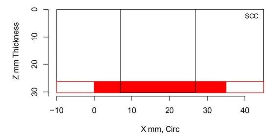
Figure H.414 Indication Plot for Procedure AECT.33 Applied to Test Block P31 in PARENT Open Testing (X – Z view)
