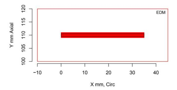
Figure H.205 Indication Plot for Procedure SAFT.17 Applied to Test Block P42 in PARENT Open Testing (X – Y view)
