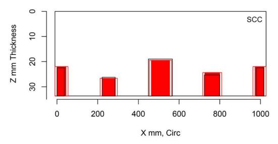
Figure H.144 Indication Plot for Procedure PAUT.131.1 Applied to Test Block P38 in PARENT Open Testing (X – Z view)
