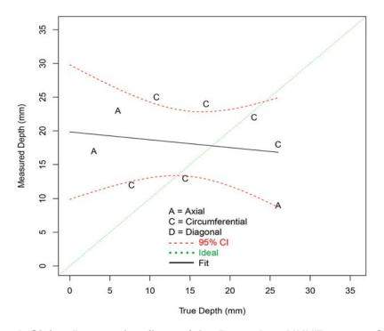
Figure F.1 Depth Sizing Regression (in mm) for Procedure HHUT.27.1 on SBDMW Test Blocks in PARENT Open Testing (O.D. access – w/ FB test blocks)
