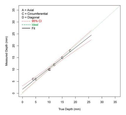
Figure F.9 Depth Sizing Regression (in mm) for Procedure PAUT.122.1 on SBDMW Test Blocks in PARENT Open Testing (O.D. access – w/ FB test blocks)
