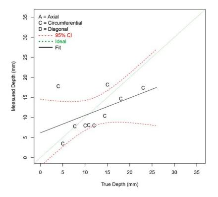
Figure F.14 Depth Sizing Regression (in mm) for Procedure PAUT.20 on SBDMW Test Blocks in PARENT Open Testing (O.D. access – w/ FB test blocks)
