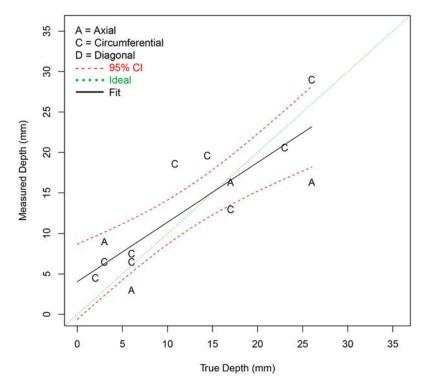
Figure F.4 Depth Sizing Regression (in mm) for Procedure PAATOFD.29.0 on SBDMW Test Blocks in PARENT Open Testing (O.D. access – w/ FB test blocks)
