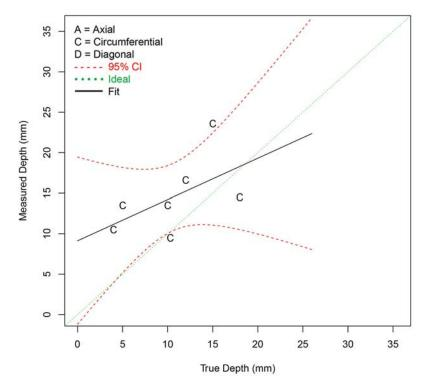
Figure F.6 Depth Sizing Regression (in mm) for Procedure PAATOFD.29.2 on SBDMW Test Blocks in PARENT Open Testing (O.D. access – w/ FB test blocks)
