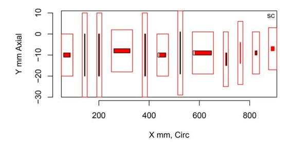
Figure H.151 Indication Plot for Procedure PAUT.131.2 Applied to Test Block P41 in PARENT Open Testing (X – Y view)
