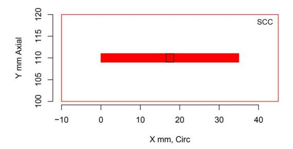
Figure H.141 Indication Plot for Procedure PAUT.131.1 Applied to Test Block P32 in PARENT Open Testing (X – Y view)
