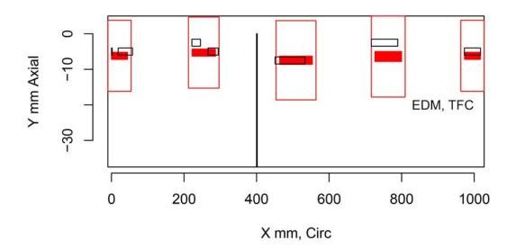
Figure H.173 Indication Plot for Procedure ECT.16 Applied to Test Block P4 in PARENT Open Testing (X – Y view)
