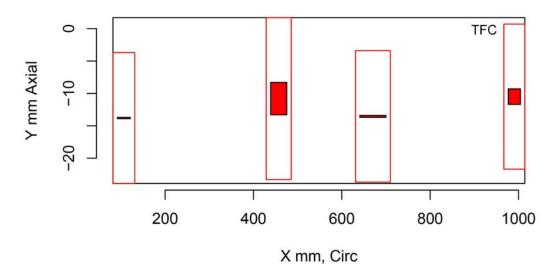
Figure H.429 Indication Plot for Procedure CEECT.5.1 Applied to Test Block P1 in PARENT Open Testing (X – Y view)
