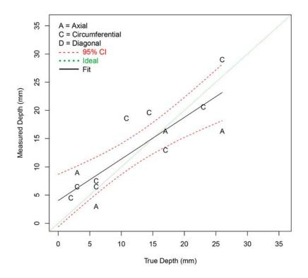
Figure F.38 Depth Sizing Regression (in mm) for Procedure PAATOFD.29.0 on SBDMW Test Blocks in PARENT Open Testing (O.D. access – w/o FB test blocks)
