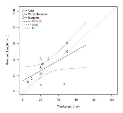
Figure G.10 Length Sizing Regression (in mm) for ADVPAUT Procedures on SBDMW Test Blocks in PARENT Open Testing (O.D. access)
