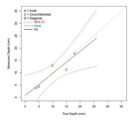
Figure F.15 Depth Sizing Regression (in mm) for Procedure RT.109 on SBDMW Test Blocks in PARENT Open Testing (O.D. access – w/ FB test blocks)
