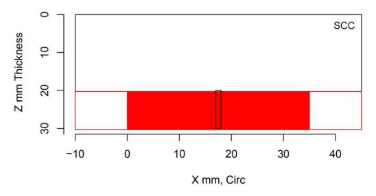
Figure H.112 Indication Plot for Procedure PAUT.122.2 Applied to Test Block P29 in PARENT Open Testing (X – Z view)
