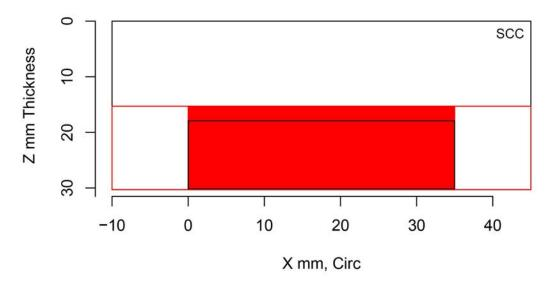
Figure H.250 Indication Plot for Procedure UIR.20 Applied to Test Block P32 in PARENT Open Testing (X – Z view)
