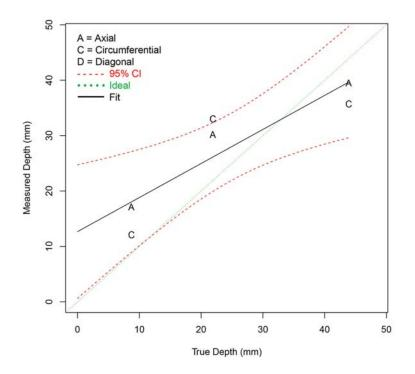
Figure F.91 Depth Sizing Regression (in mm) for Procedure PAATOFD.29.1 on LBDMW Test Blocks in PARENT Open Testing (I.D. access)
