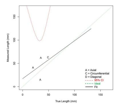
Figure G.20 Length Sizing Regression (in mm) for PAUT Procedures on LBDMW Test Blocks in PARENT Open Testing (O.D. access)
