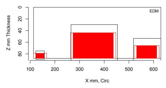
Figure H.204 Indication Plot for Procedure SAFT.17 Applied to Test Block P24 in PARENT Open Testing (X – Z view)
