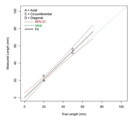
Figure G.4 Length Sizing Regression (in mm) for Procedure PAUT.131.4 on SBDMW Test Blocks in PARENT Open Testing (O.D. access)
