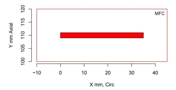
Figure H.55 Indication Plot for Procedure RT.109 Applied to Test Block P30 in PARENT Open Testing (X – Y view)
