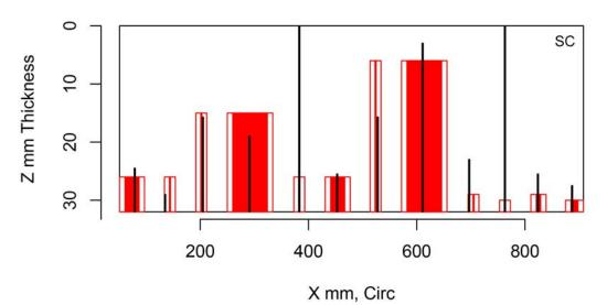
Figure H.362 Indication Plot for Procedure PAATOFD.29.0 Applied to Test Block P41 in PARENT Open Testing (X – Z view)
