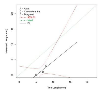
Figure G.29 Length Sizing Regression (in mm) for Procedure AECT.33 on BMI Test Blocks in PARENT Open Testing (J-groove weld access)
