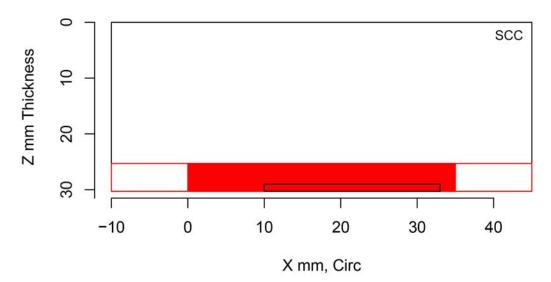
Figure H.272 Indication Plot for Procedure HHUT.27.1 Applied to Test Block P38 in PARENT Open Testing (X – Z view)
