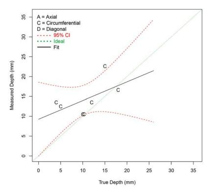
Figure F.5 Depth Sizing Regression (in mm) for Procedure PAATOFD.29.1 on SBDMW Test Blocks in PARENT Open Testing (O.D. access – w/ FB test blocks)
