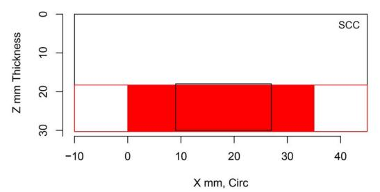
Figure H.106 Indication Plot for Procedure PAUT.122.1 Applied to Test Block P28 in PARENT Open Testing (X – Z view)
