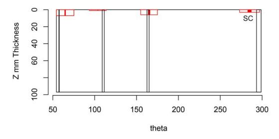
Figure H.34 Indication Plot for Procedure ECT.7 Applied to Test Block P7 in PARENT Open Testing (theta – Z view)
