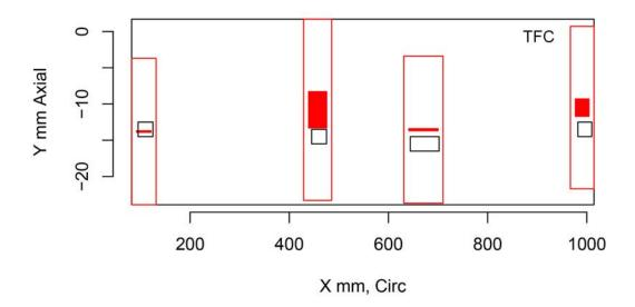
Figure H.145 Indication Plot for Procedure PAUT.131.1 Applied to Test Block P1 in PARENT Open Testing (X – Y view)
