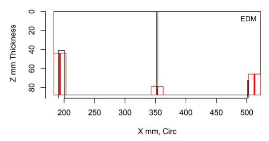
Figure H.202 Indication Plot for Procedure SAFT.17 Applied to Test Block P23 in PARENT Open Testing (X – Z view)
