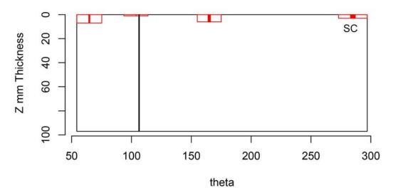
Figure H.14 Indication Plot for Procedure LUV.170 Applied to Test Block P7 in PARENT Open Testing (theta – Z view)
