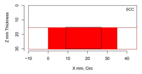
Figure H.122 Indication Plot for Procedure PAUT.122.1 Applied to Test Block P32 in PARENT Open Testing (X – Z view)
