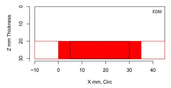
Figure H.278 Indication Plot for Procedure HHUT.27.1 Applied to Test Block P42 in PARENT Open Testing (X – Z view)
