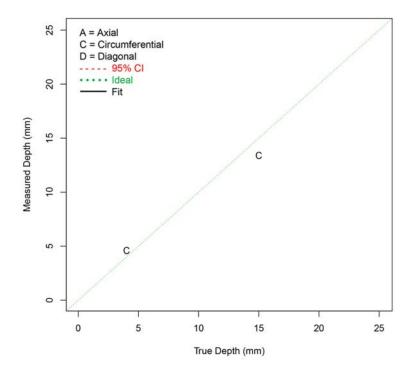
Figure F.82 Depth Sizing Regression (in mm) for PAUT Procedures on FB Test Blocks in PARENT Open Testing (I.D. access)
