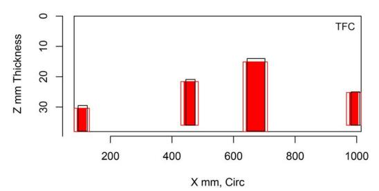
Figure H.146 Indication Plot for Procedure PAUT.131.1 Applied to Test Block P1 in PARENT Open Testing (X – Z view)
