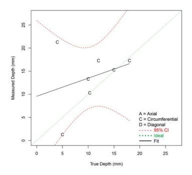
Figure F.54 Depth Sizing Regression (in mm) for Procedure HHUT.27.2 on FB Test Blocks in PARENT Open Testing (O.D. access)
