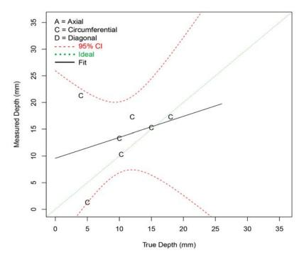
Figure F.2 Depth Sizing Regression (in mm) for Procedure HHUT.27.2 on SBDMW Test Blocks in PARENT Open Testing (O.D. access – w/ FB test blocks)
