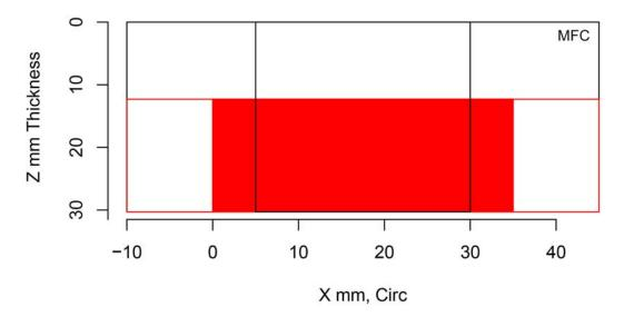
Figure H.412 Indication Plot for Procedure AECT.33 Applied to Test Block P30 in PARENT Open Testing (X – Z view)
