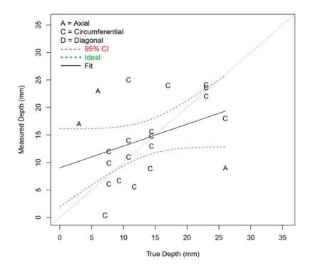
Figure F.50 Depth Sizing Regression (in mm) for NLUT Procedures on SBDMW Test Blocks in PARENT Open Testing (O.D. access – w/o FB test blocks)
