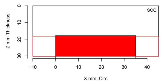
Figure H.182 Indication Plot for Procedure SAFT.17 Applied to Test Block P28 in PARENT Open Testing (X – Z view)
