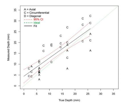
Figure F.49 Depth Sizing Regression (in mm) for ADVPAUT Procedures on SBDMW Test Blocks in PARENT Open Testing (O.D. access – w/o FB test blocks)
