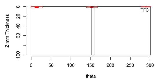
Figure H.8 Indication Plot for Procedure LUV.170 Applied to Test Block P5 in PARENT Open Testing (theta – Z view)
