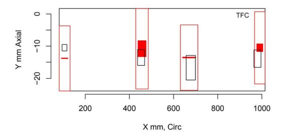
Figure H.255 Indication Plot for Procedure PAUT.20 Applied to Test Block P1 in PARENT Open Testing (X – Y view)
