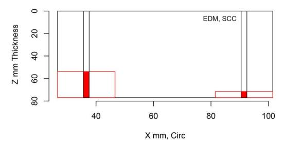
Figure H.370 Indication Plot for Procedure PAATOFD.29.1 Applied to Test Block P12 in PARENT Open Testing (X – Z view)
