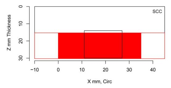
Figure H.94 Indication Plot for Procedure PAUT.114 Applied to Test Block P32 in PARENT Open Testing (X – Z view)
