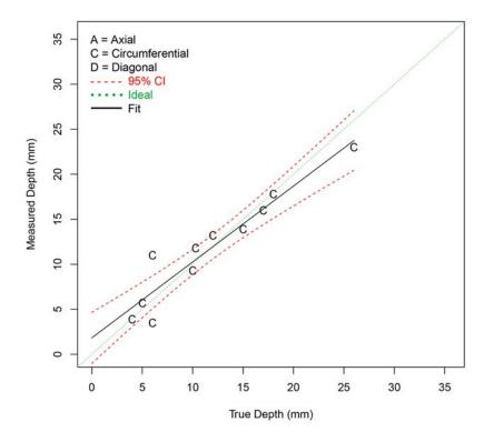
Figure F.22 Depth Sizing Regression (in mm) for Procedure UT.104 on SBDMW Test Blocks in PARENT Open Testing (O.D. access – w/ FB test blocks)
