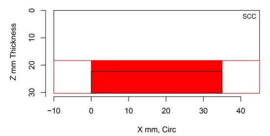
Figure H.232 Indication Plot for Procedure PAUT.20 Applied to Test Block P28 in PARENT Open Testing (X – Z view)
