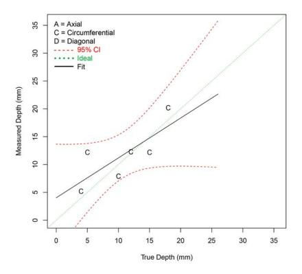
Figure F.21 Depth Sizing Regression (in mm) for Procedure UIR.20 on SBDMW Test Blocks in PARENT Open Testing (O.D. access – w/ FB test blocks)
