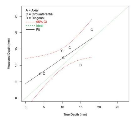
Figure F.68 Depth Sizing Regression (in mm) for Procedure UIR.20 on FB Test Blocks in PARENT Open Testing (O.D. access)
