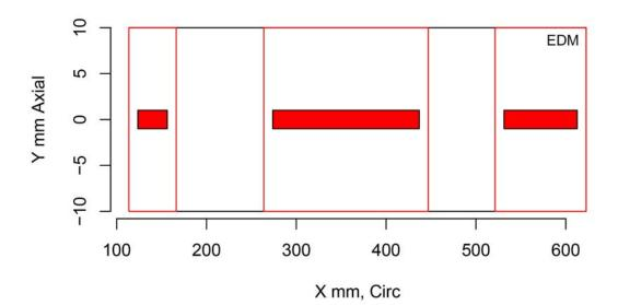
Figure H.379 Indication Plot for Procedure PAATOFD.29.0 Applied to Test Block P24 in PARENT Open Testing (X – Y view)
