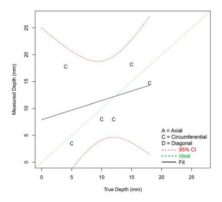
Figure F.61 Depth Sizing Regression (in mm) for Procedure PAUT.131.1 on FB Test Blocks in PARENT Open Testing (O.D. access)
