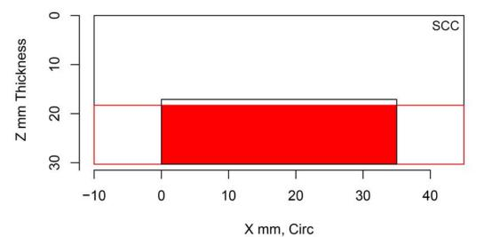
Figure H.36 Indication Plot for Procedure UT.104 Applied to Test Block P28 in PARENT Open Testing (X – Z view)
