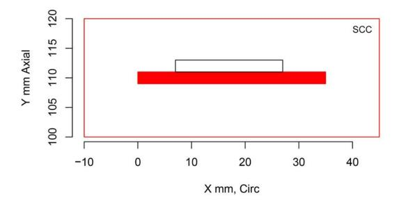
Figure H.413 Indication Plot for Procedure AECT.33 Applied to Test Block P31 in PARENT Open Testing (X – Y view)
