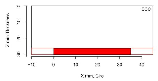
Figure H.42 Indication Plot for Procedure UT.104 Applied to Test Block P31 in PARENT Open Testing (X – Z view)
