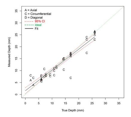
Figure F.51 Depth Sizing Regression (in mm) for PAUT Procedures on SBDMW Test Blocks in PARENT Open Testing (O.D. access – w/o FB test blocks)
