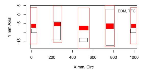
Figure H.99 Indication Plot for Procedure PAUT.114 Applied to Test Block P4 in PARENT Open Testing (X – Y view)
