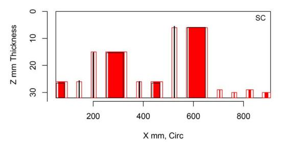
Figure H.150 Indication Plot for Procedure PAUT.131.1 Applied to Test Block P41 in PARENT Open Testing (X – Z view)
