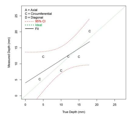
Figure F.74 Depth Sizing Regression (in mm) for UIR Procedures on FB Test Blocks in PARENT Open Testing (O.D. access)
