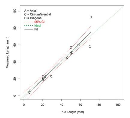
Figure G.3 Length Sizing Regression (in mm) for Procedure PAUT.131.2 on SBDMW Test Blocks in PARENT Open Testing (O.D. access)
