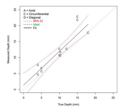
Figure F.80 Depth Sizing Regression (in mm) for ADVPAUT Procedures on FB Test Blocks in PARENT Open Testing (I.D. access)
