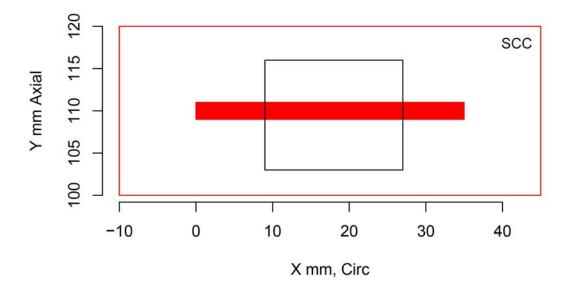
Figure H.87 Indication Plot for Procedure PAUT.114 Applied to Test Block P29 in PARENT Open Testing (X – Y view)
