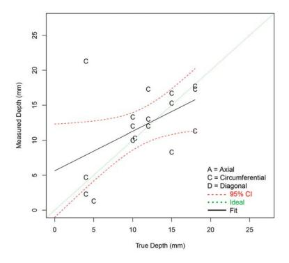
Figure F.71 Depth Sizing Regression (in mm) for NLUT Procedures on FB Test Blocks in PARENT Open Testing (O.D. access)
