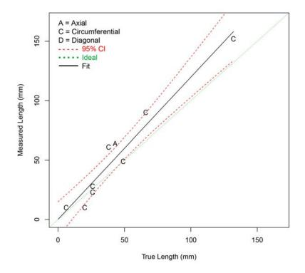
Figure G.18 Length Sizing Regression (in mm) for Procedure SAFT.17 on LBDMW Test Blocks in PARENT Open Testing (O.D. access)
