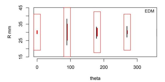
Figure H.29 Indication Plot for Procedure ECT.7 Applied to Test Block P21 in PARENT Open Testing (theta – R view)
