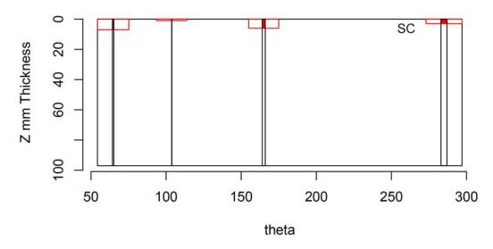
Figure H.26 Indication Plot for Procedure CEECT.5.1 Applied to Test Block P7 in PARENT Open Testing (theta – Z view)
