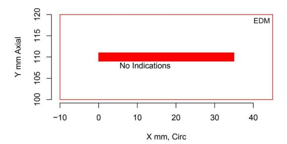
Figure H.63 Indication Plot for Procedure RT.109 Applied to Test Block P42 in PARENT Open Testing (X – Y view)
