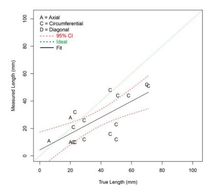
Figure G.11 Length Sizing Regression (in mm) for NLUT Procedures on SBDMW Test Blocks in PARENT Open Testing (O.D. access)
