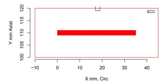
Figure H.347 Indication Plot for Procedure PAATOFD.29.1 Applied to Test Block P38 in PARENT Open Testing (X – Y view)
