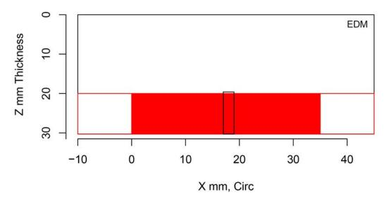
Figure H.388 Indication Plot for Procedure PATP.29 Applied to Test Block P42 in PARENT Open Testing (X – Z view)
