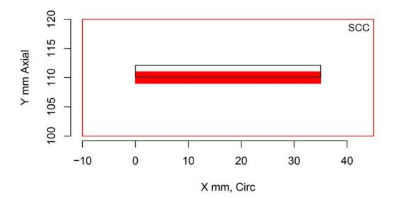
Figure H.37 Indication Plot for Procedure UT.104 Applied to Test Block P29 in PARENT Open Testing (X – Y view)
