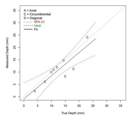
Figure F.3 Depth Sizing Regression (in mm) for Procedure LASH.18 on SBDMW Test Blocks in PARENT Open Testing (O.D. access – w/ FB test blocks)
