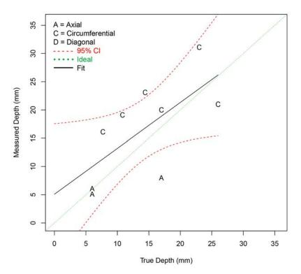
Figure F.7 Depth Sizing Regression (in mm) for Procedure PATP.29 on SBDMW Test Blocks in PARENT Open Testing (O.D. access – w/ FB test blocks)
