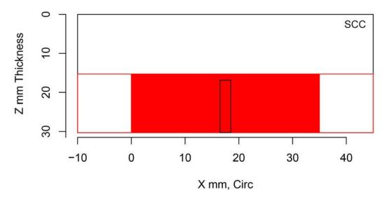
Figure H.142 Indication Plot for Procedure PAUT.131.1 Applied to Test Block P32 in PARENT Open Testing (X – Z view)
