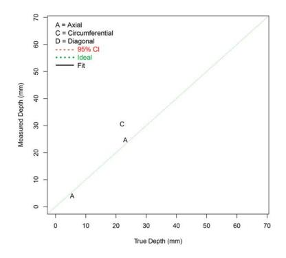
Figure F.90 Depth Sizing Regression (in mm) for PAUT Procedures on LBDMW Test Blocks in PARENT Open Testing (O.D. access)
