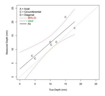
Figure F.77 Depth Sizing Regression (in mm) for Procedure PAATOFD.29.1 on FB Test Blocks in PARENT Open Testing (I.D. access)
