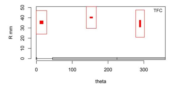
Figure H.17 Indication Plot for Procedure GW.21 Applied to Test Block P5 in PARENT Open Testing (theta – R view)
