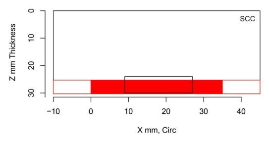
Figure H.126 Indication Plot for Procedure PAUT.122.1 Applied to Test Block P38 in PARENT Open Testing (X – Z view)
