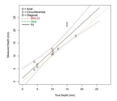
Figure F.33 Depth Sizing Regression (in mm) for ADVPAUT Procedures on SBDMW Test Blocks in PARENT Open Testing (I.D. access – w/ FB test blocks)
