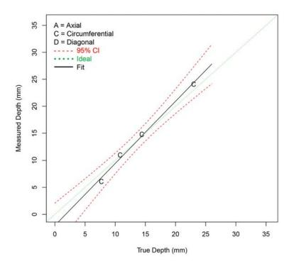
Figure F.37 Depth Sizing Regression (in mm) for Procedure LASH.18 on SBDMW Test Blocks in PARENT Open Testing (O.D. access – w/o FB test blocks)
