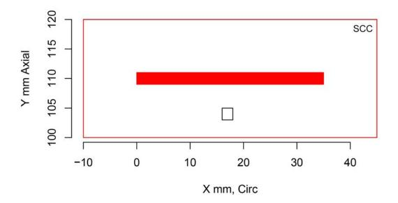
Figure H.345 Indication Plot for Procedure PATP.29 Applied to Test Block P38 in PARENT Open Testing (X – Y view)
