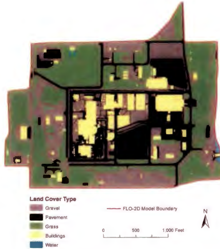
Figure 3.2-4. Land-use Map for the Wolf Creek Site Used for Local Intense Precipitation Flood Analysis.
